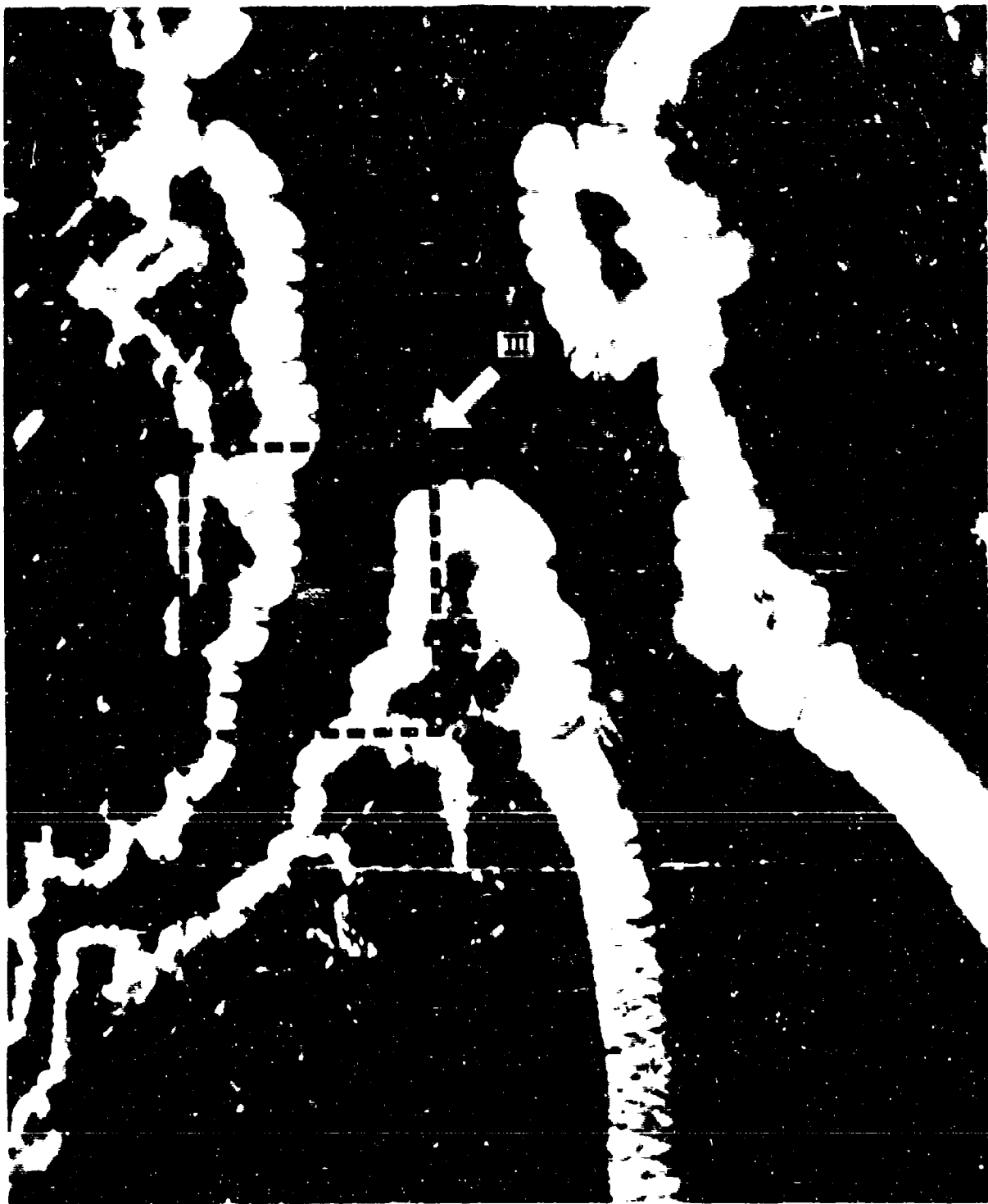
1000X View Made on Thin Section "A", at One Location Indicated on the 50X View (Arrow-II), Showing Anisotropic Material Deposition at Pore Surfaces and Between Carbon Fibers
