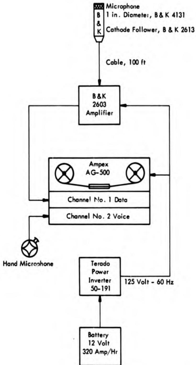
FIGURE A1 - Instrumentation Used for Recording Aircraft Noise
