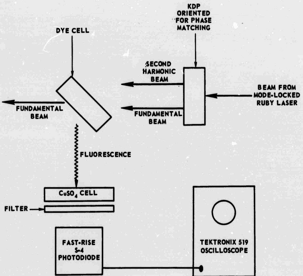
EXPERIMENTAL ARRANGEMENT FOR OBSERVING GAIN IN SATURABLE ABSORBERS
