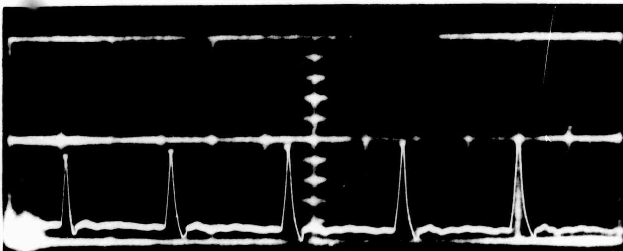
(a) MODE-LOCKED RUBY LASER OUTPUT - 10 nsec/cm
