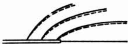
Fig. 18.1. Diagram of the lines of force of the magnetic field. — in the absence of motion; - - - with jet motion.
