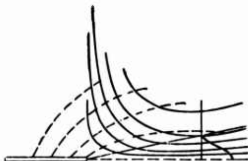
Fig. 18.5. Diagram of the streamlines and the magnetic lines of force in a jet.
