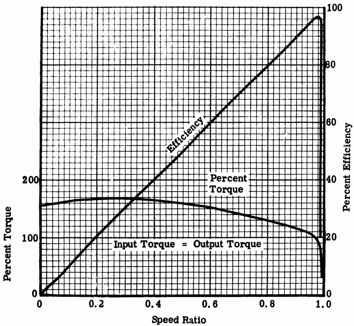
Figure 27. Typical Torque and Efficiency Characteristics of a Fluid Coupling.
