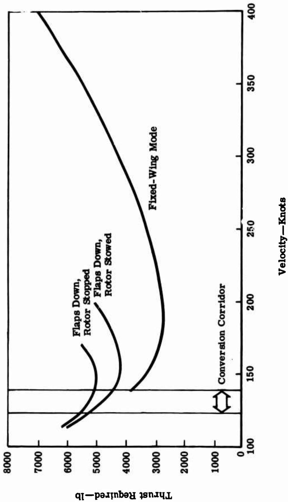
Figure 3. Thrust Required for Representative Advanced Rotary-Wing Aircraft.
