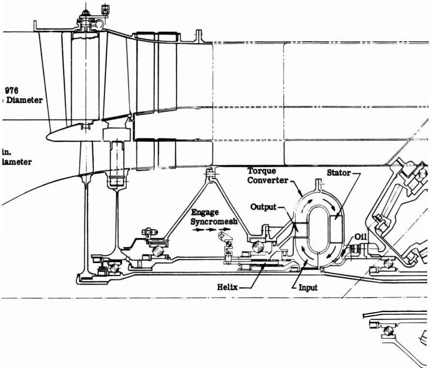
Supercharged With Torque Converter Decoupler
