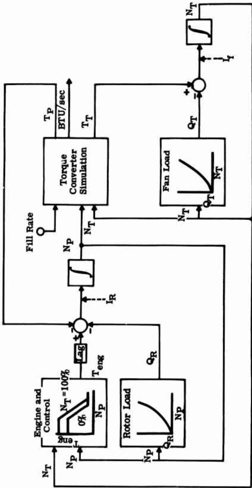
Figure 71. Block Diagram of Convertible Fan/Shaft Engine Simulation.
