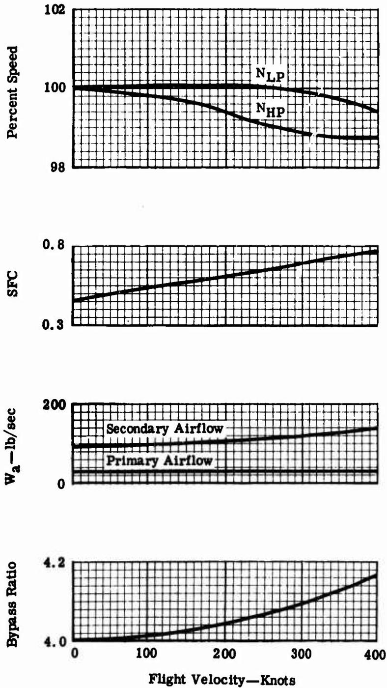
Figure 10. Type III Engine, Cruise Fan Performance Characteristics Versus Flight Speed.
