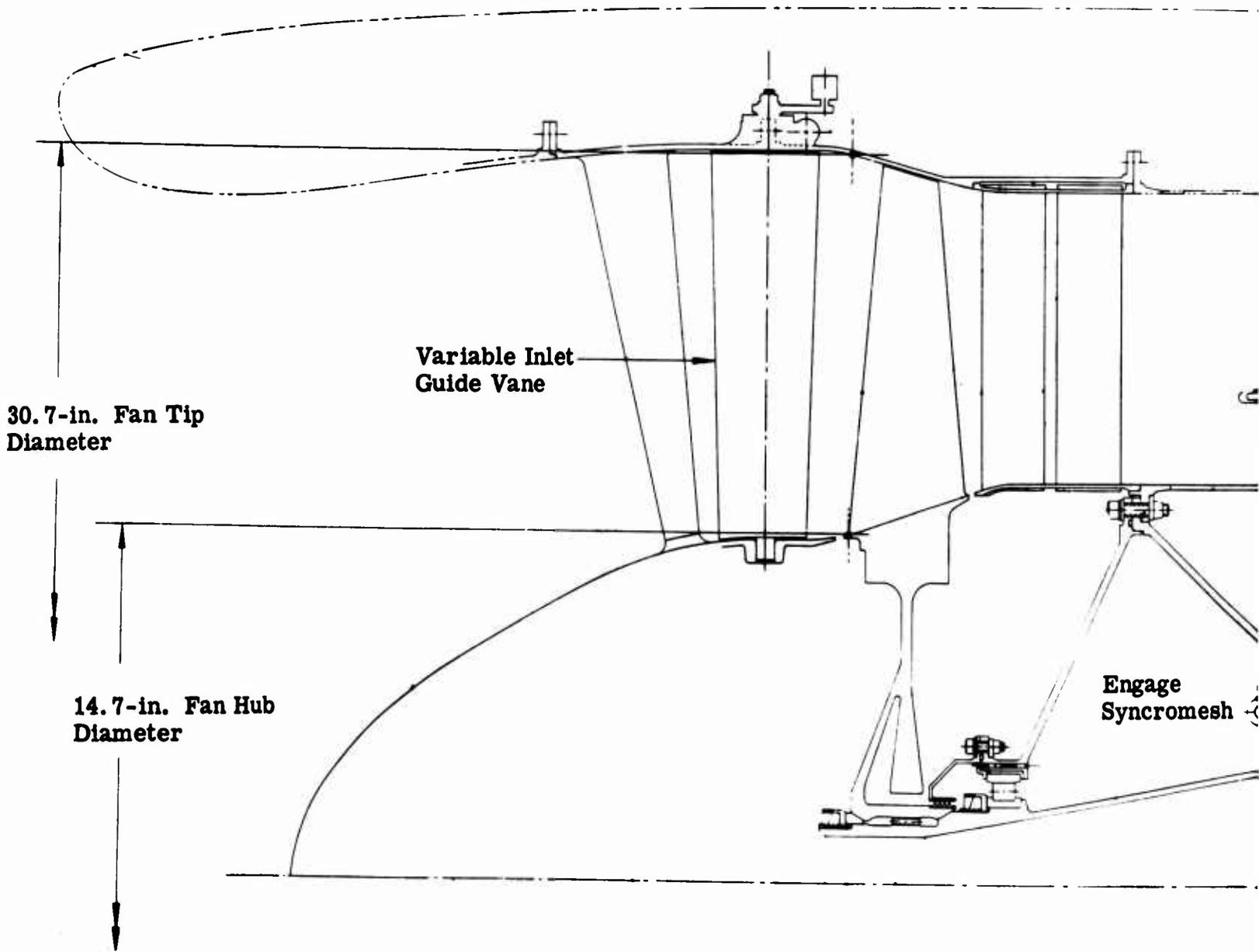
**Figure 32. Type IA, Supercharged Engine With Variable Inlet Guide Vanes, Torque Converter, and Front 90-Degree Rotor Drive.**
