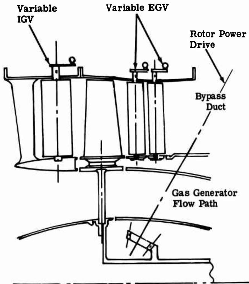
Figure 44. Type III Engine, Nonsupercharged With Variable Bypass Inlet Guide Vanes and Variable Bypass Exit Guide Vanes.
