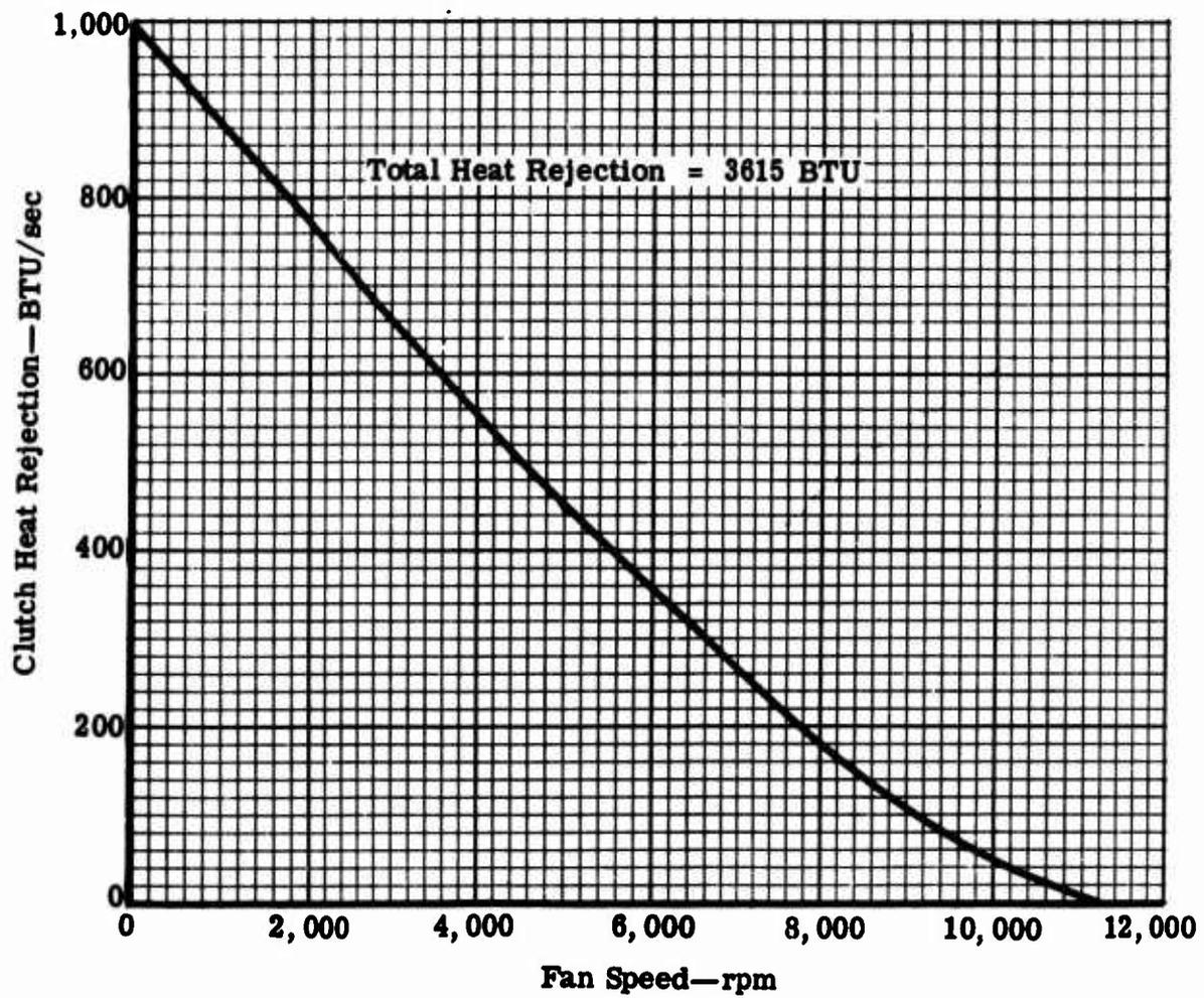
Figure 25. Friction Clutch Heat Rejection Rate Versus Fan Speed.
