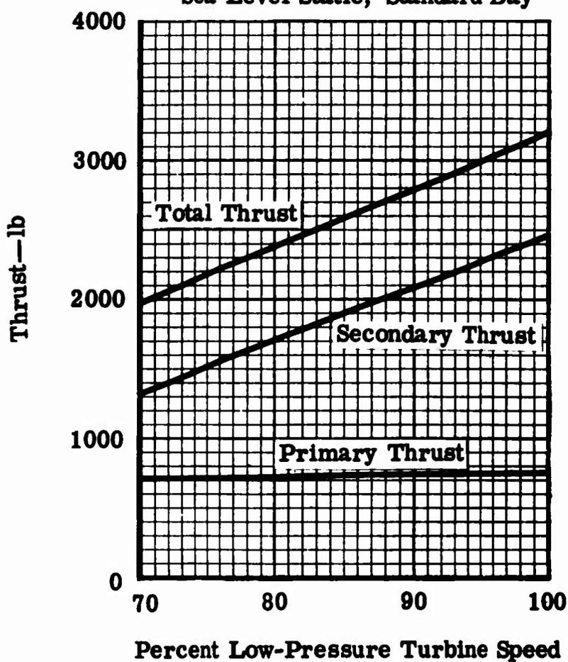
Figure 20. Thrust Available From Type III Engine at Reduced Low-Pressure Turbine Speed.
