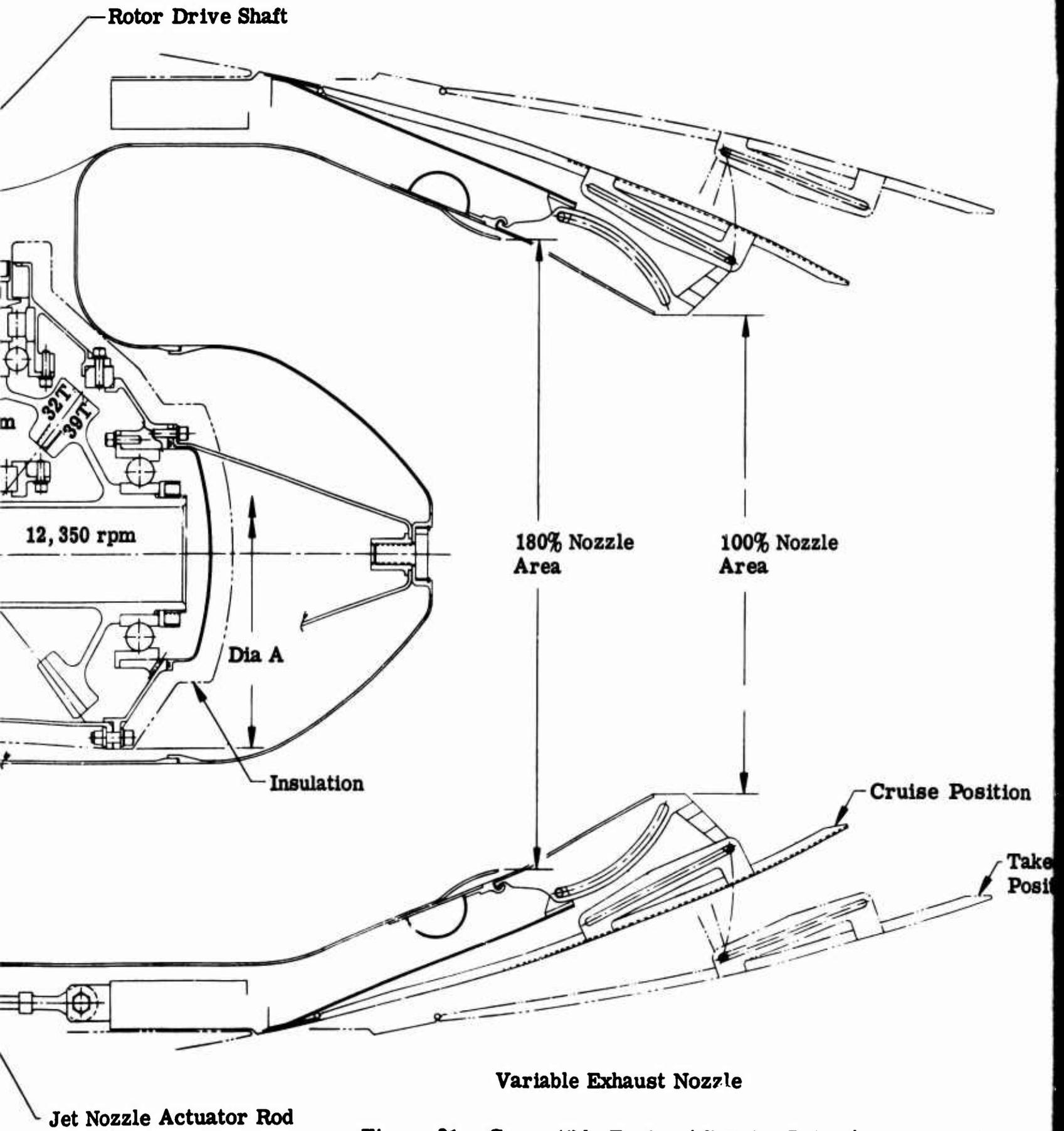
Figure 31. Convertible Engine Aft Rotor Drive Arrangement.
