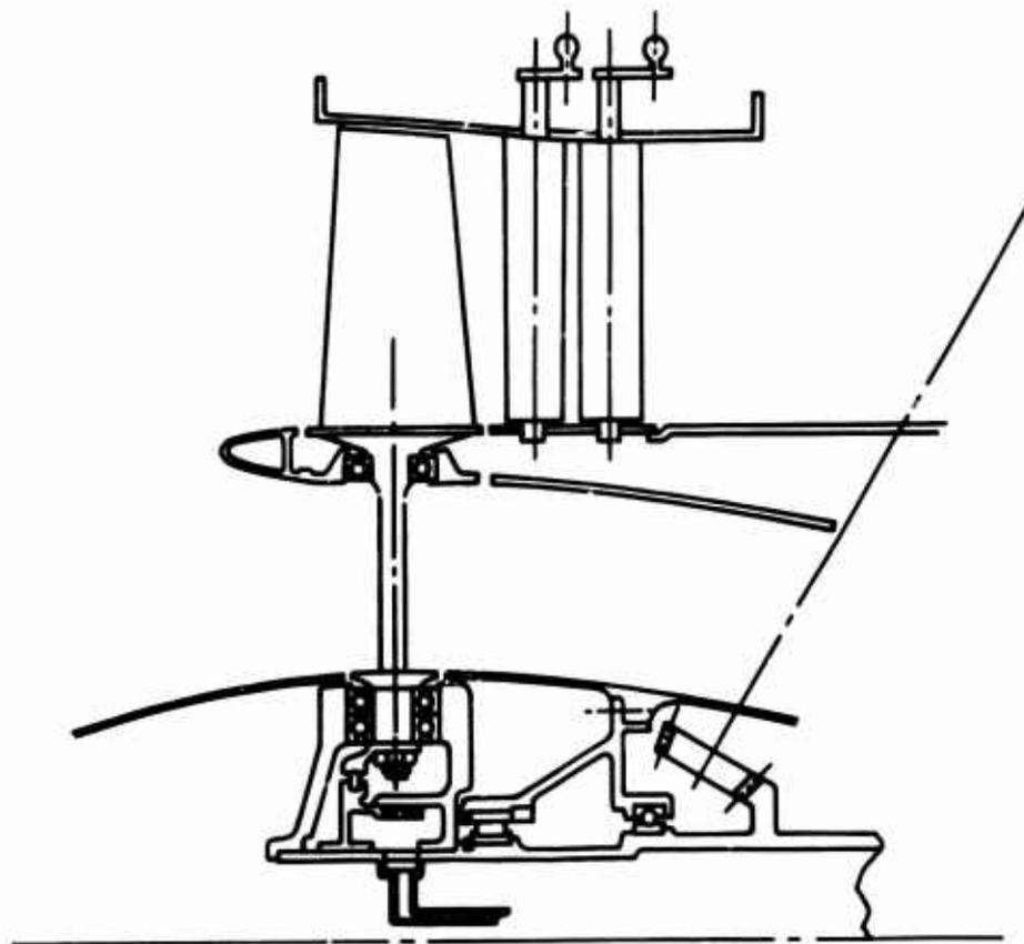
Figure 46. Type III Engine With Variable Fan Blade.
