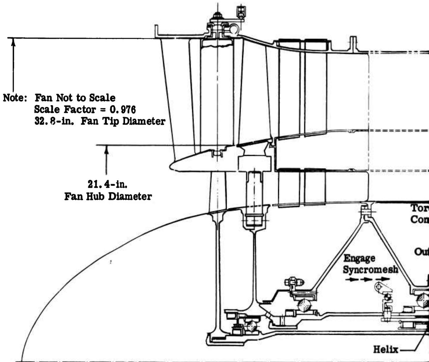
Figure 30. Type IIA, Supercharged With Torque Converter Decoupler for Bypass Fan.
