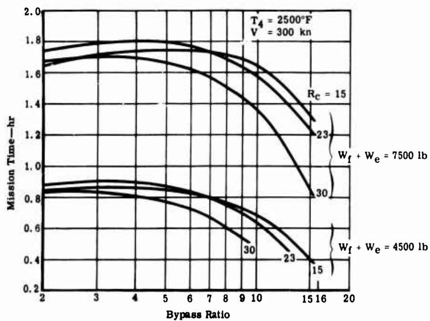
Figure 68. Mission Time Versus Bypass Ratio—2500°F.
