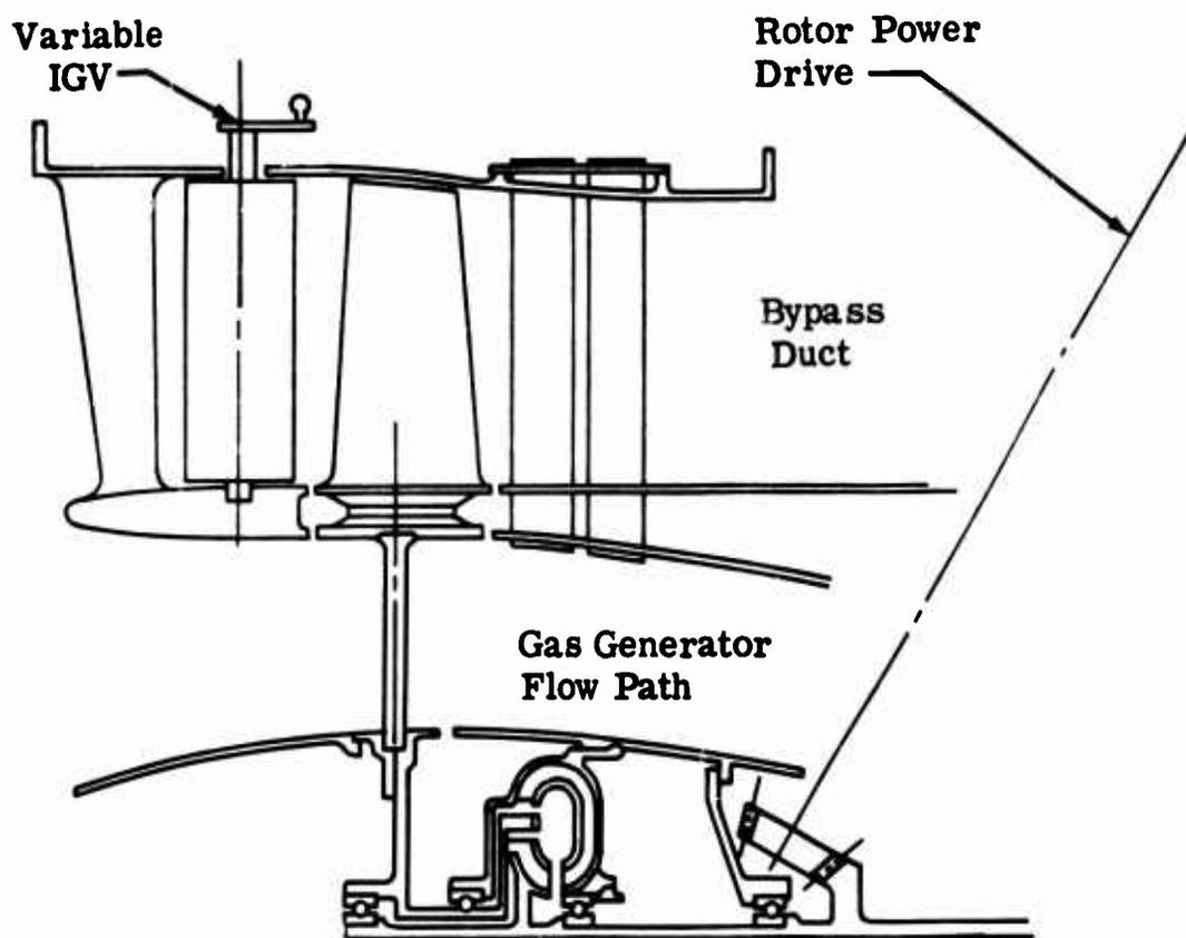
**Figure 47. Type IIIA Engine, Nonsupercharged With Variable Bypass Inlet Guide Vanes, Fixed Bypass Exit Guide Vanes, and Fan Decoupler.**
