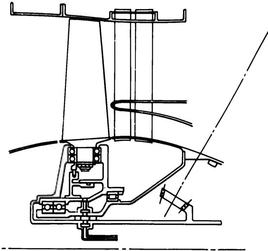
**Figure 35. Type I Engine With Variable Total Fan Blade.**
