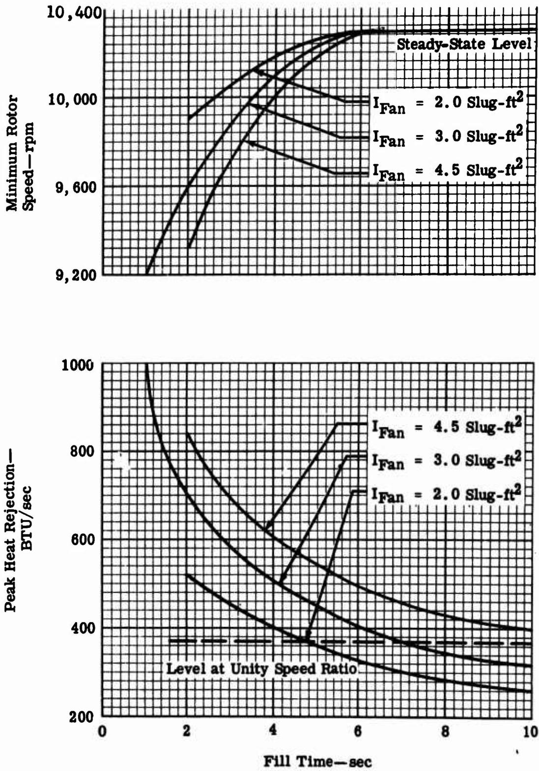
Figure 50. Analog Analysis of Torque Converter Filling Rate.
