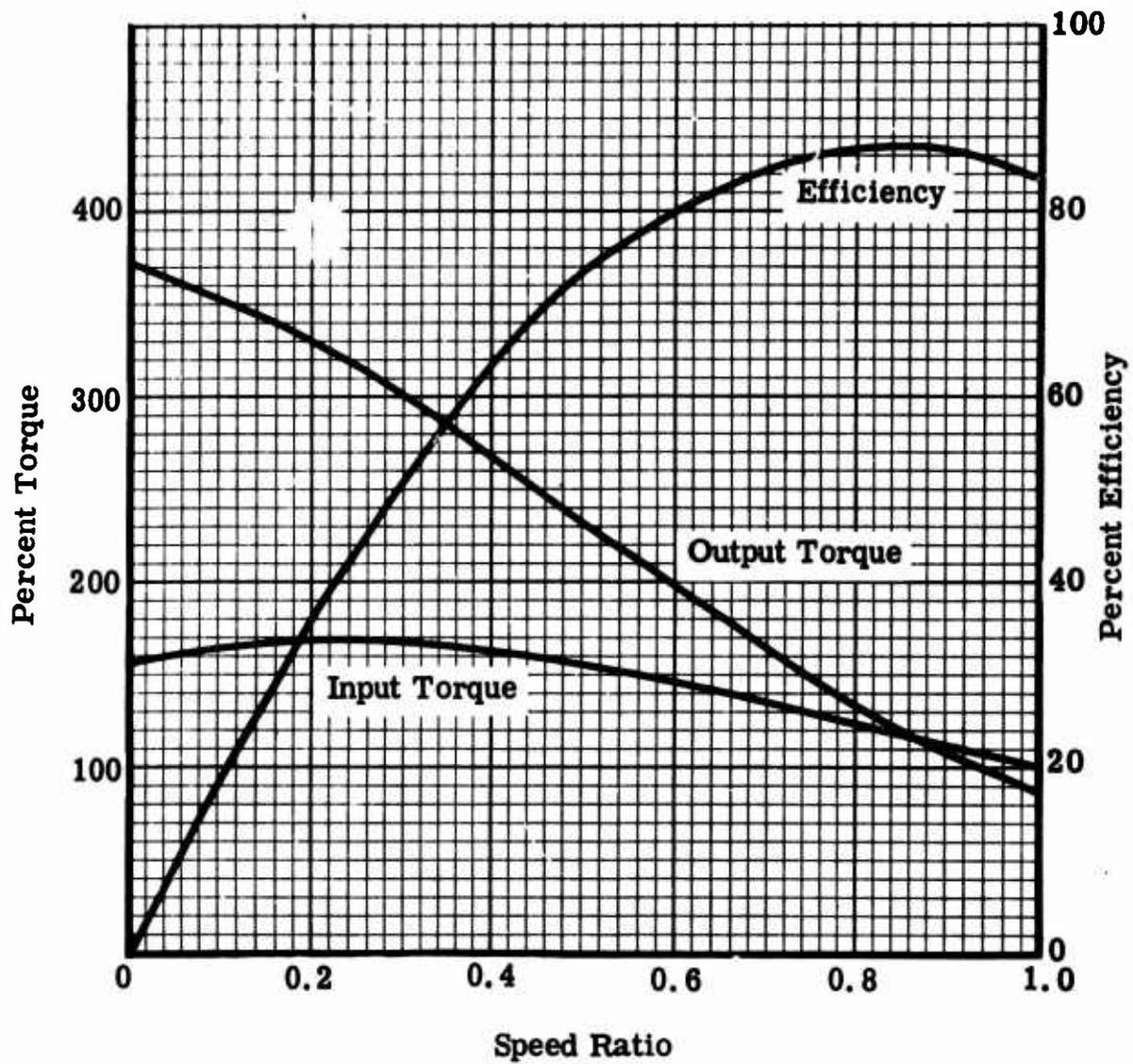
Figure 28. Typical Torque and Efficiency Characteristics of a Torque Converter.
