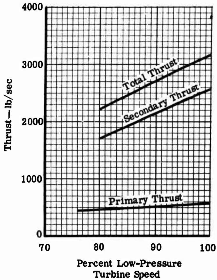
Figure 15. Thrust Available From Type I Engine at Reduced Low-Pressure Turbine Speed.
