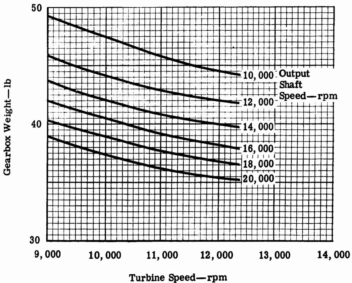
Figure 59. Weight Scaling Data for 45-Degree Shaft Angle Gearbox.
