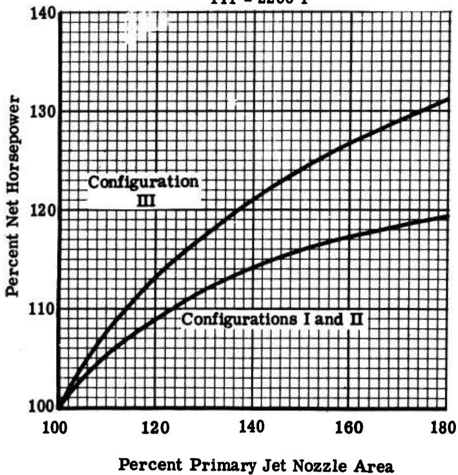
Figure 11. Effect of Primary Jet Nozzle Area on Net Horsepower.
