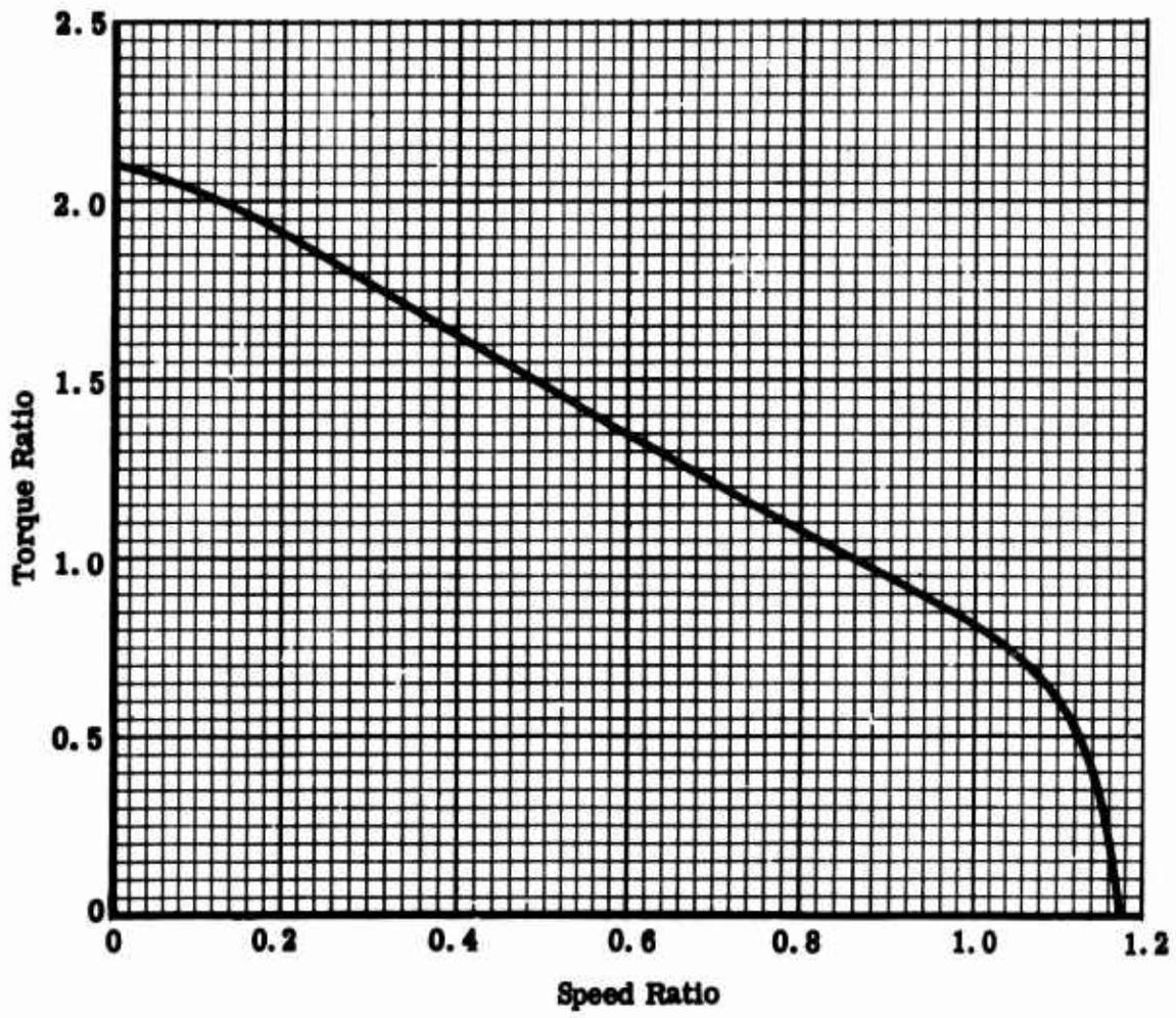
Figure 74. Torque Ratio as a Function of Speed Ratio.
