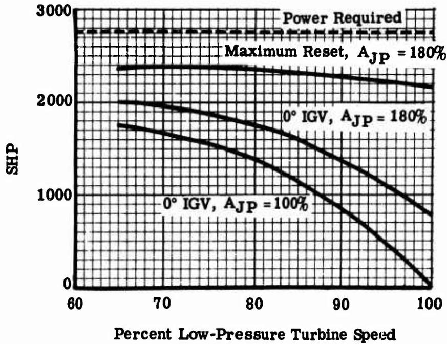
Figure 14. Shaft Horsepower and Total Thrust Available From Type I Engine at Reduced Low-Pressure Turbine Speed.
