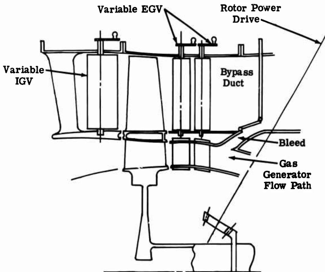
**Figure 40. Type II Engine, Supercharged With Variable Bypass Inlet Guide Vanes, Variable Bypass Exit Guide Vanes, and Gas Generator Inlet Air Bleed.**
