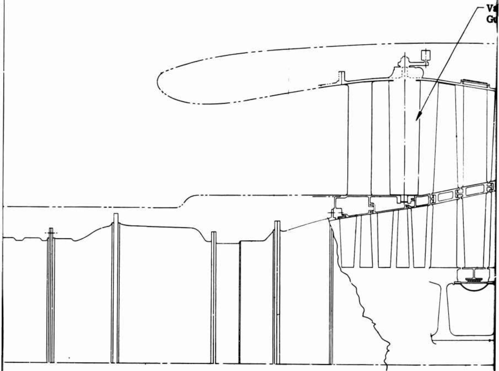
45. Nonsupercharged Engine With Aft Fan, 90-Degree Rear Rotor Drive, and Variable Inlet Guide Vanes.
