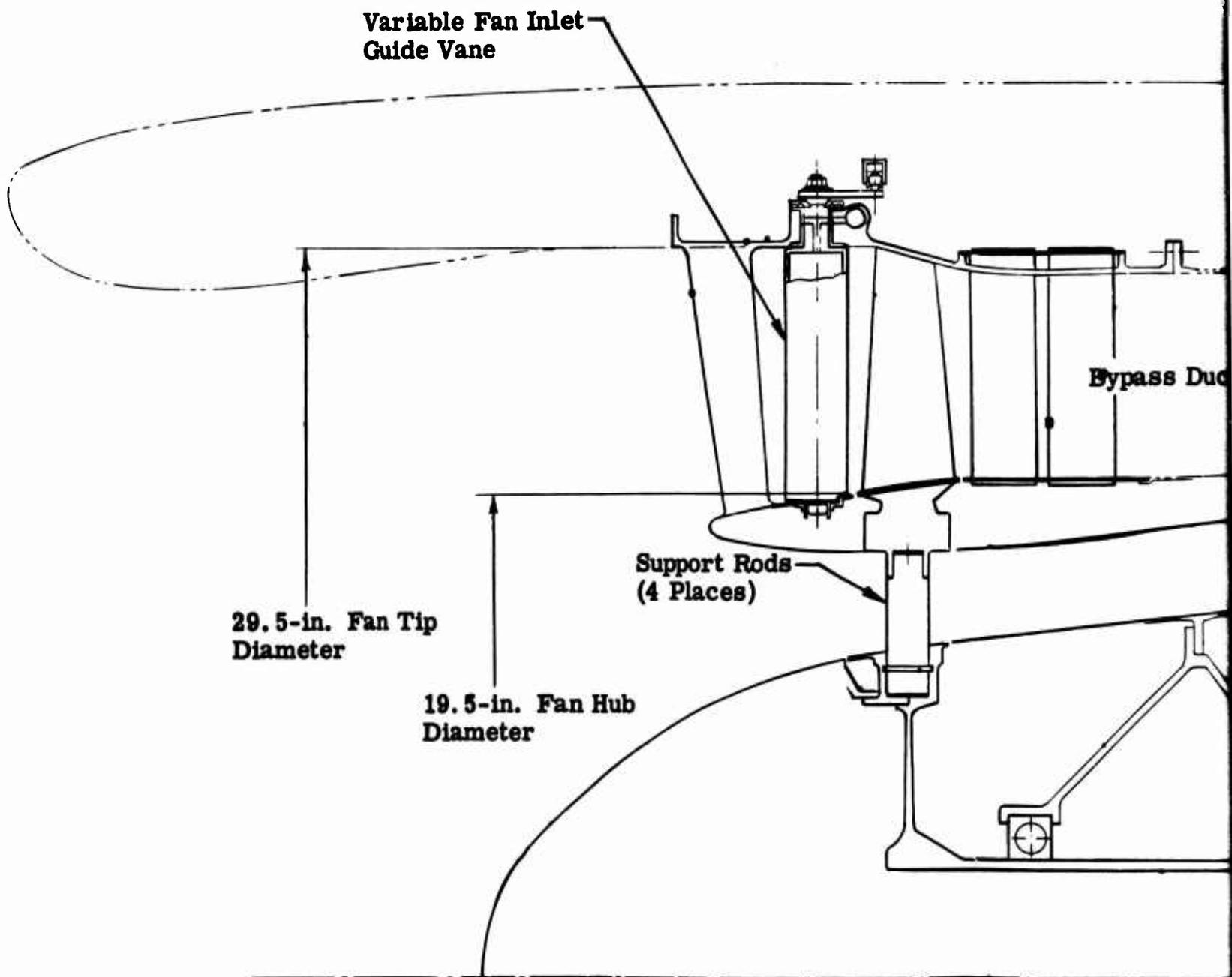
Figure 48. Type IIIA Nonsupercharged Engine With Aft Drive and Fan Decoupler.
