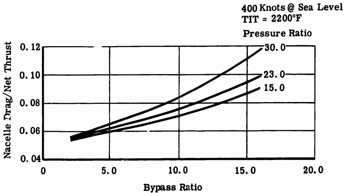
Figure 65. Study Engine Drag Characteristics Versus Bypass Ratio.
