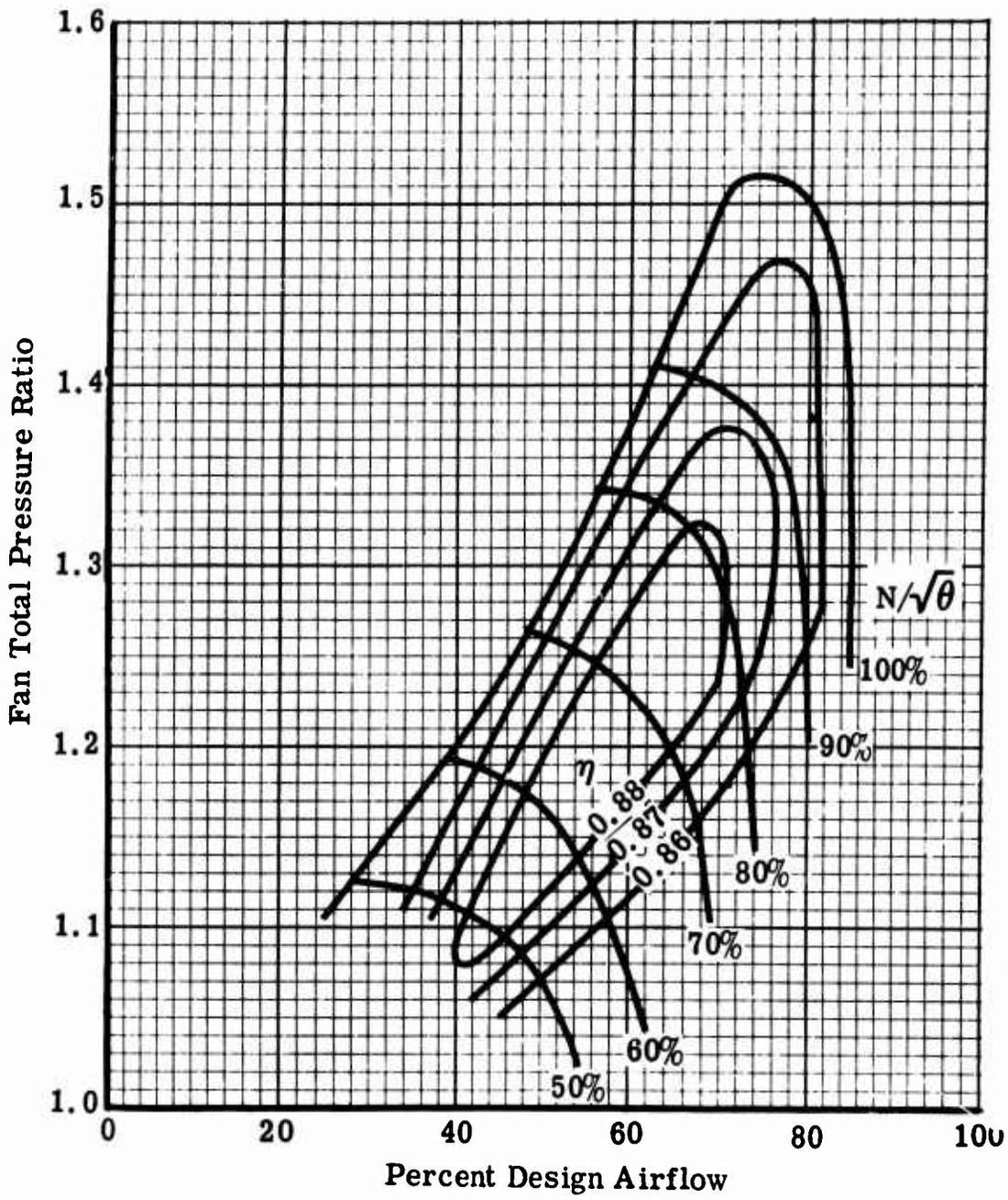
Figure 13. Fan Characteristics With Inlet Guide Vanes in the Maximum Reset Position.
