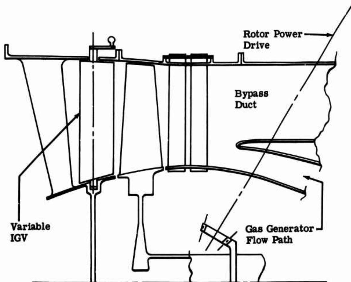
**Figure 33. Type I Engine, Supercharged With Variable Total Inlet Guide Vanes and Fixed Total Exit Guide Vanes.**
