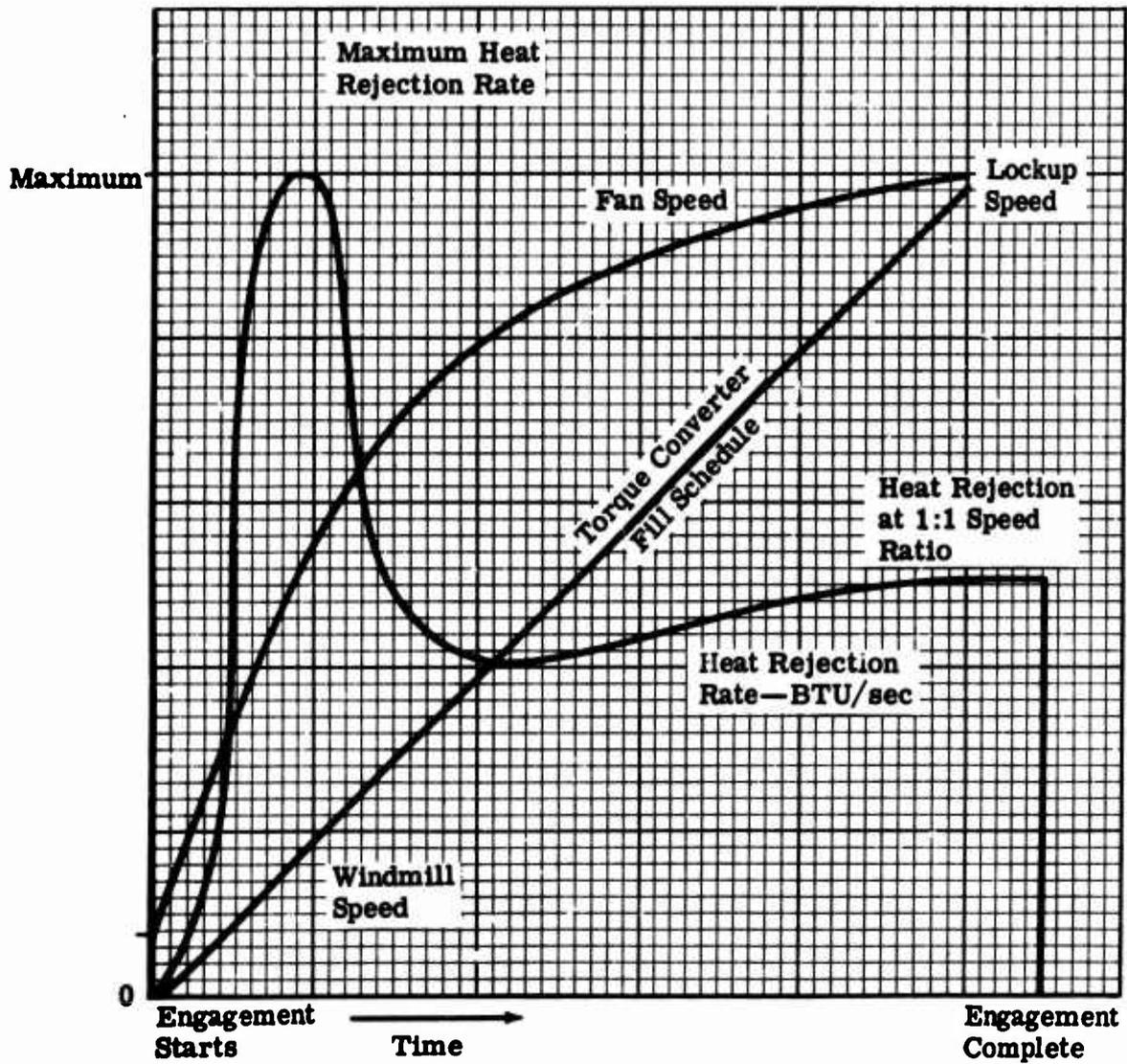
Figure 29. Typical Curves for Torque Converter Fill Study.
