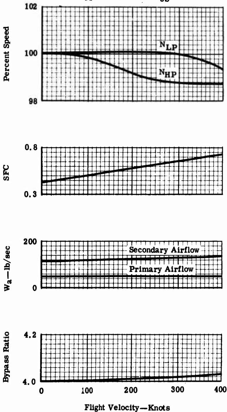
Figure 8. Type II Engine, Cruise Fan Performance Characteristics Versus Flight Speed.
