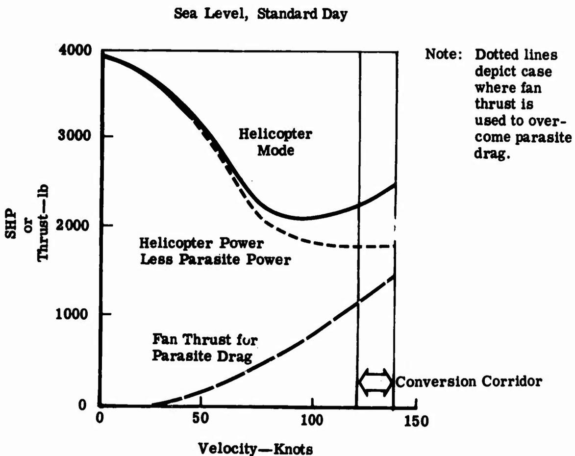
Figure 2. Power Required for Representative Advanced Rotary-Wing Aircraft.
