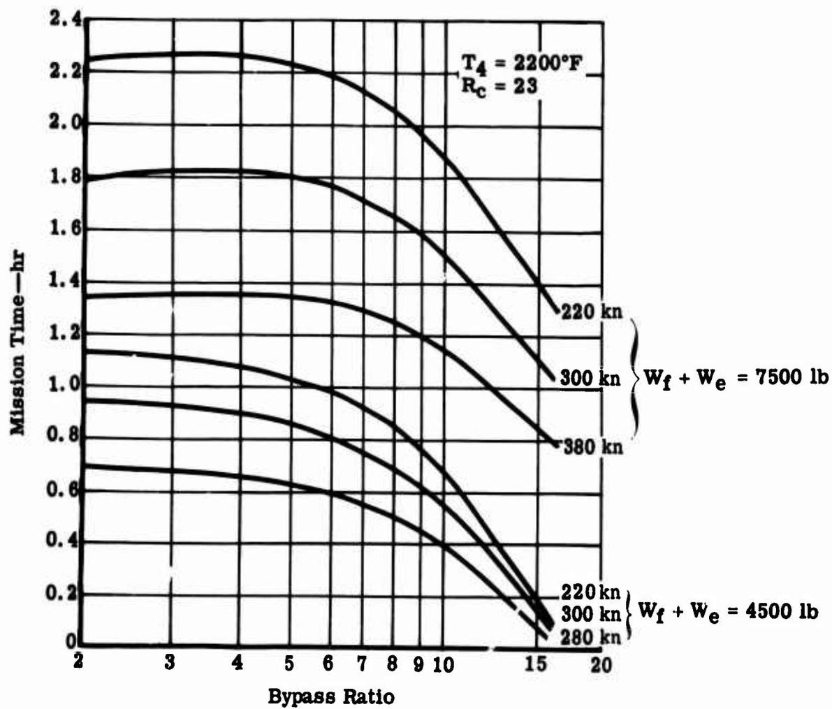
Figure 70. Effect of Cruise Speed on Mission Time.
