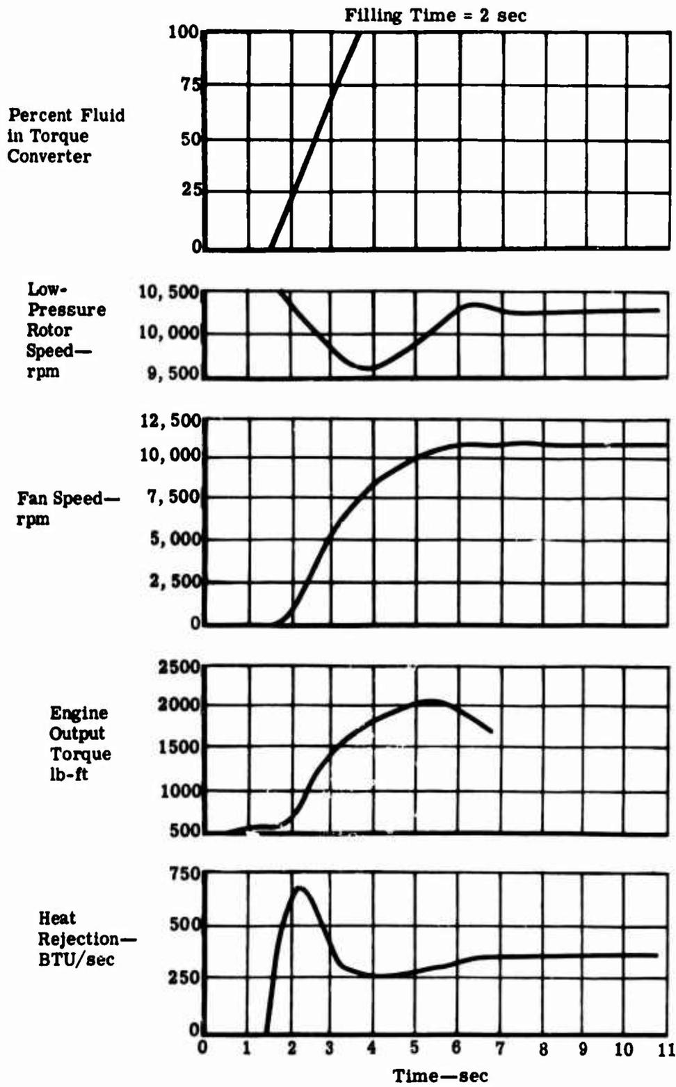
Figure 76. Analog Computer Analysis of Torque Converter—2 Seconds Fill Time.
