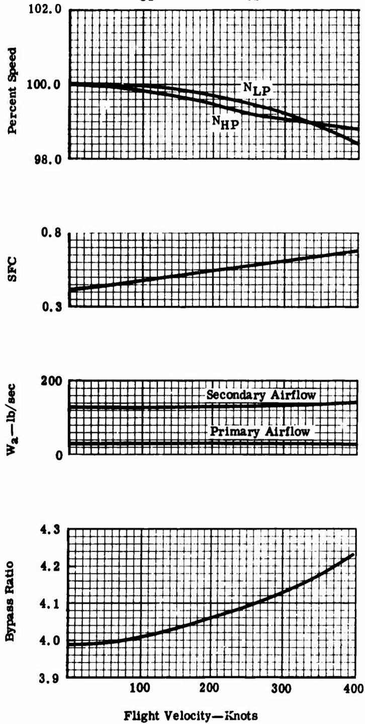
Figure 6. Type I Engine, Cruise Fan Performance Characteristics Versus Flight Speed.
