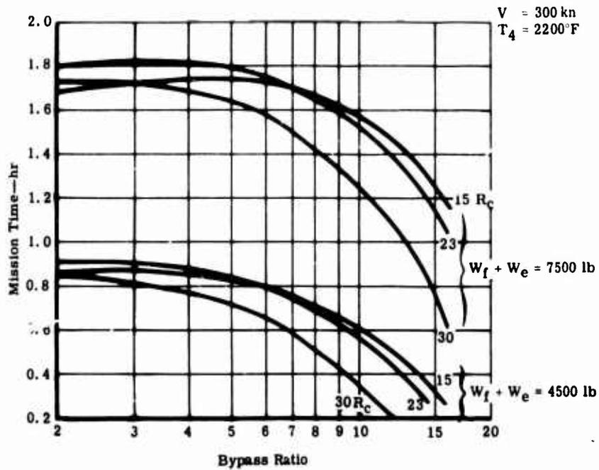
Figure 67. Mission Time Versus Bypass Ratio—2200°F.
