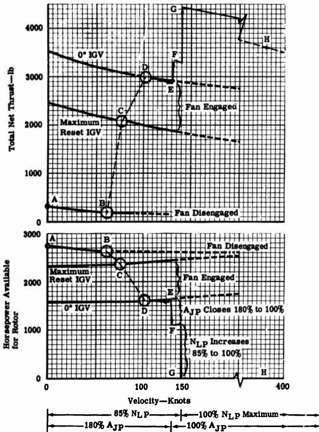
Figure 64. Type IA Shaft-to-Fan Conversion Analysis—Sea Level Standard Day.
