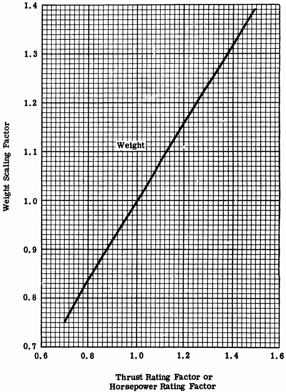
Figure 57. Type IA Engine Weight Scaling Factor.
