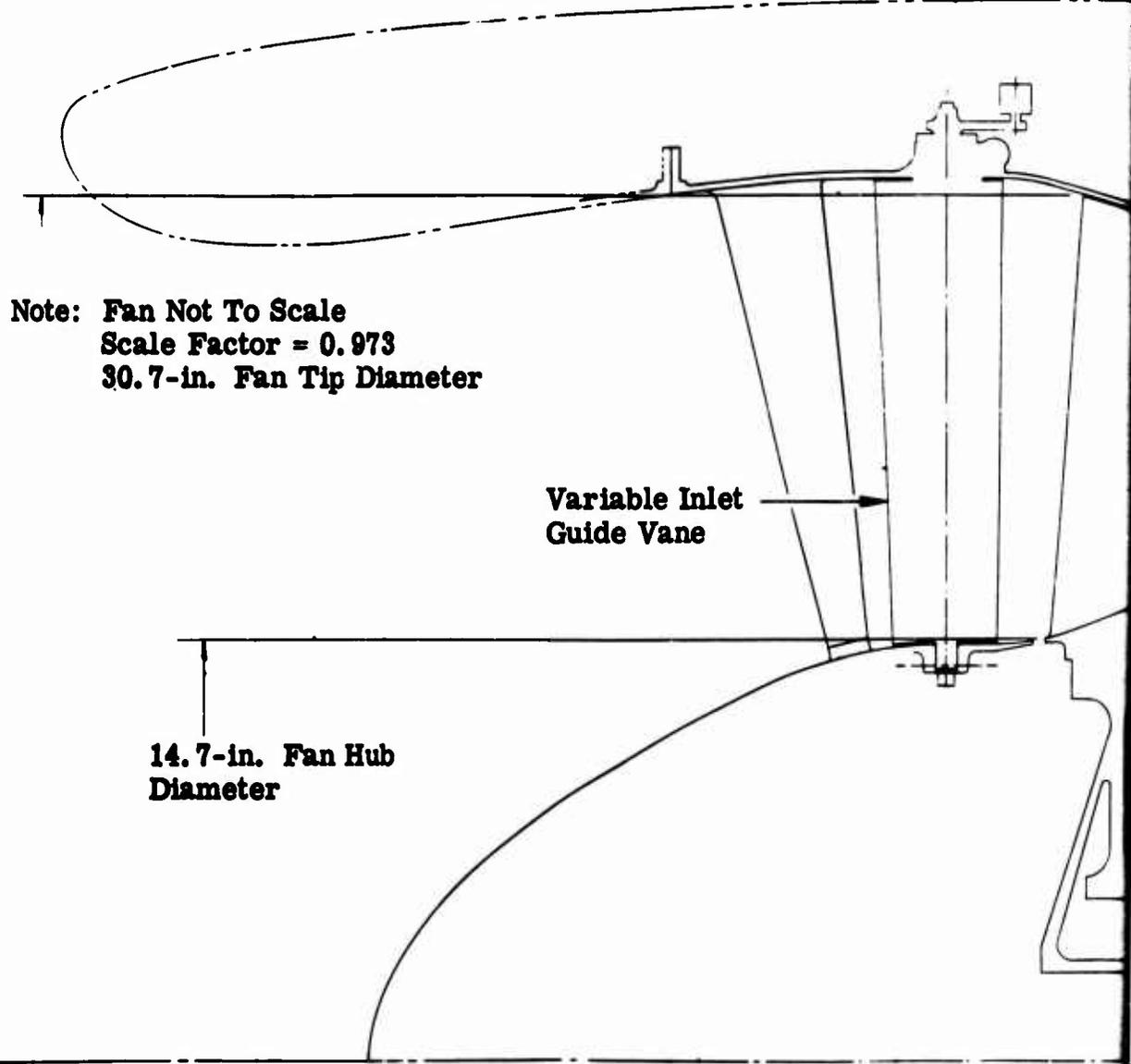
Figure 34. Type I Supercharged Engine With Variable Inlet Guide Vane and Front 45-Degree Rotor Drive.
