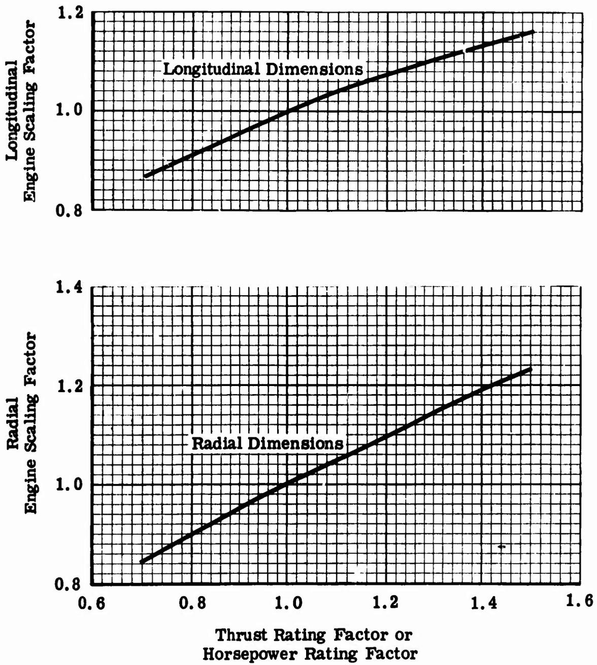
Figure 56. Type IA Engine Size Scaling Factors.
