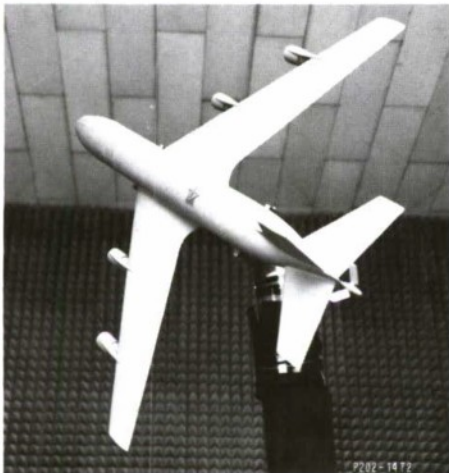
Fig. 3. KC-135 aircraft and antenna (1/25-scale model) under test.
