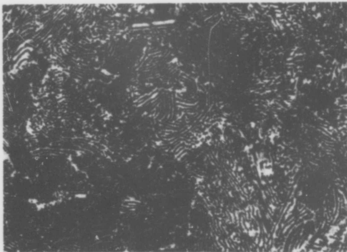
Figure 16. Hf-Cr (59-41 At%), Rapidly Cooled from 1510°C. X1000 \beta -Hf + \text{HfCr}_2 Eutectic
