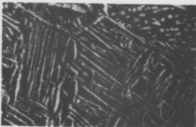
Figure 14(b). X375 Hf-Cr (90-10 At%), Cooled at 3°C per Second from 1550°C. Slightly Hypo-Eutectoid Composition. Eutectoid Not Resolved.
