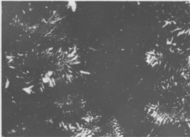
Figure 5. Hf-V (81-19 At%), Cooled at 3°C per Second X2500 from 1400°C.
