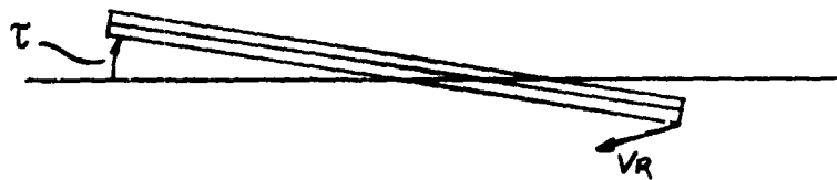
CASE (9): Lower Surface Wetted, 0 < \tau < +3^\circ ("Two-Dimensional Impact")
