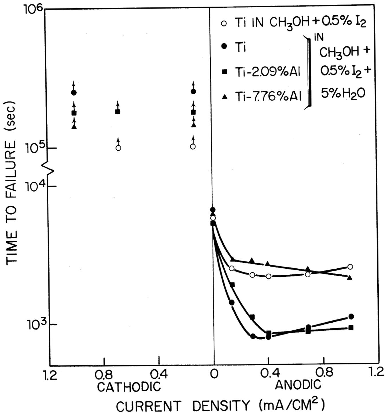
Fig. 4. Effect of applied anodic and cathodic currents on  $t_f$  of titanium and Ti-Al binary alloys in methanol-iodine and methanol-iodine-water solutions. Applied stress:- Ti  $\equiv$  95% Y.S., Ti-2.09 w/o Al  $\equiv$  90% Y.S., Ti-7.76 w/o Al  $\equiv$  85% Y.S.
