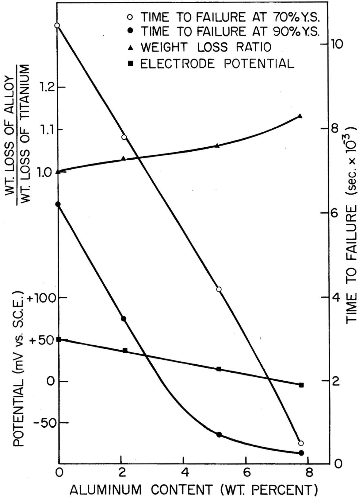
Fig. 2. Effect of aluminum content on weight loss (96 hr. exposure), electrode potential, and  $t_p$  in methanol-iodine solution containing no added water.
