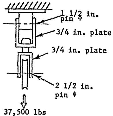
After the cables leave the movable sheaves, the remaining stresses are identical for all three systems.
