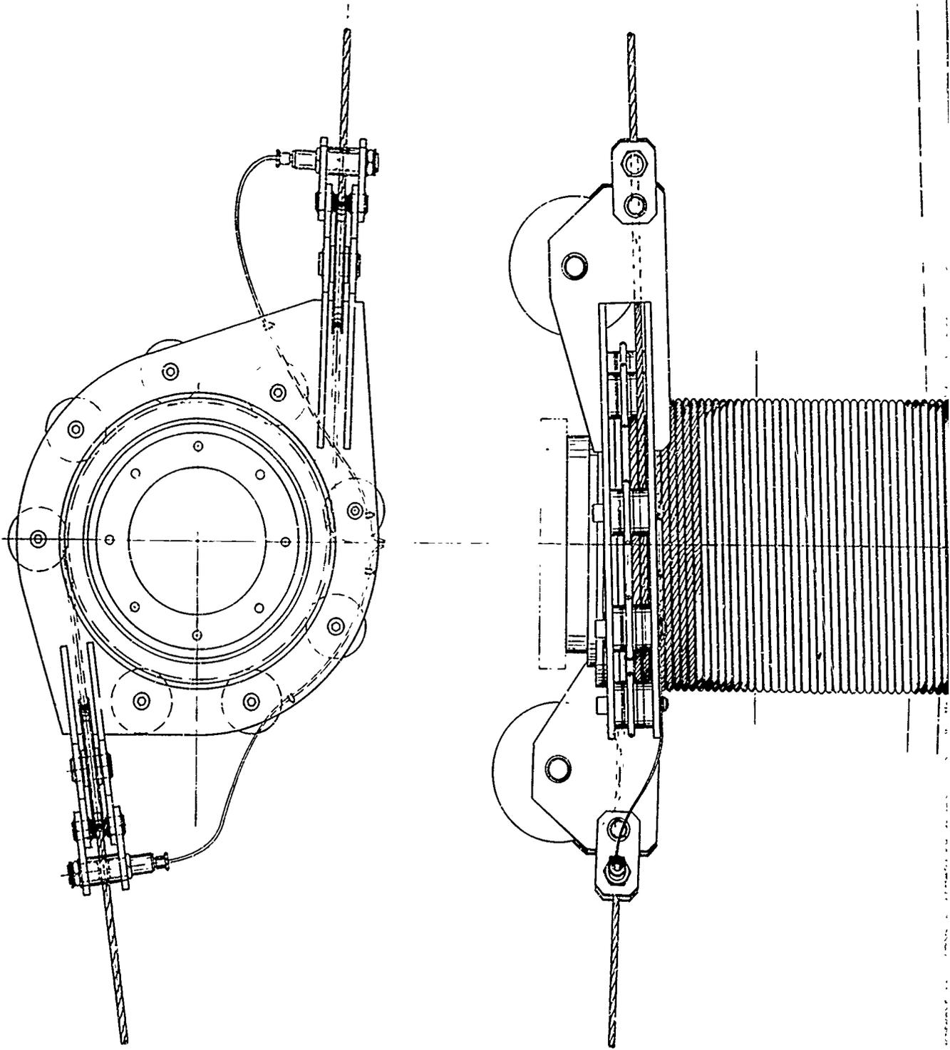
Figure 17. Top and Side Views of Drum System
