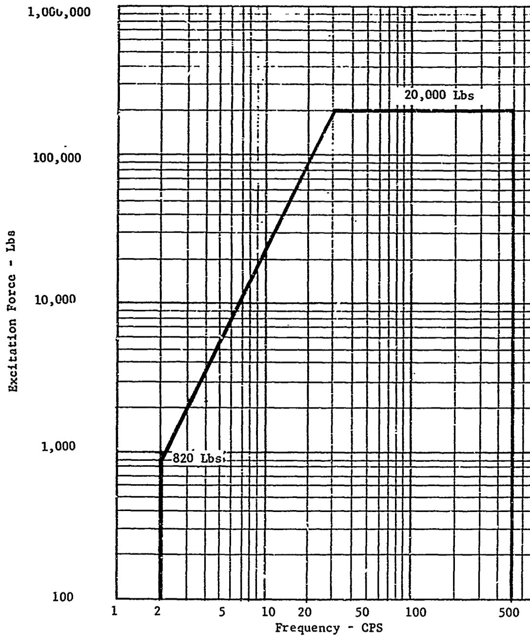
Figure 19. Force Spectrum for Helicopter in Flight
