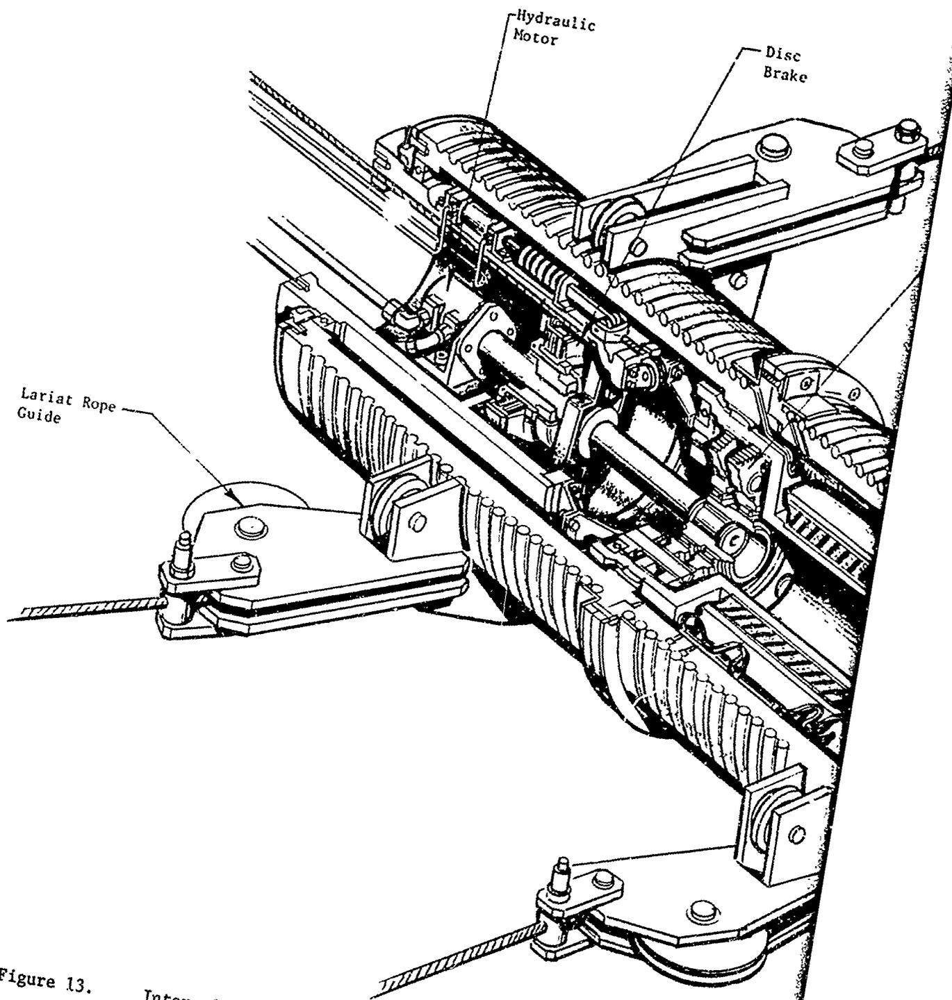
Figure 13. Internal Drive Drum
