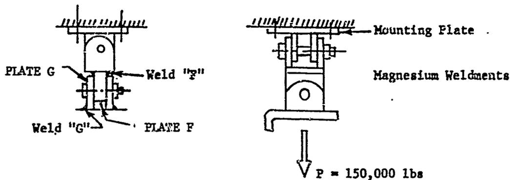
Plate thickness, 2.00 in Magnesium
