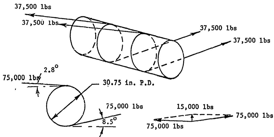
Resultant upward load on drum of 15,000 lbs is reacted equally at each end of drum. The 7,500 lbs reaction is carried in shear by eight 3/4-in.-diameter bolts at each end of the drum. The torque in the system,  $T_d = 30.75/2 (150,000)$ .
