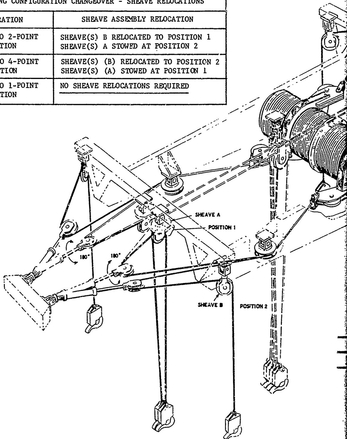
Figure 29. 1-, 2-, and 4-Point Reeving Systems Superimposed
