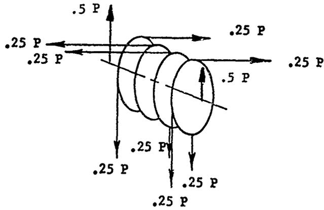
One quarter of the design load  $P$  applied by one sheave to the shaft results in the following load distribution.
