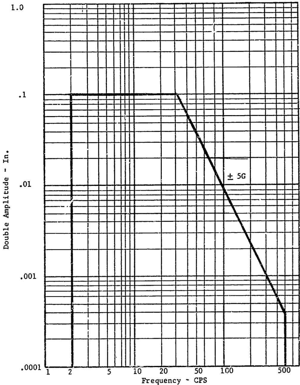
Figure 18. Vibration Spectrum for Helicopter in Flight
