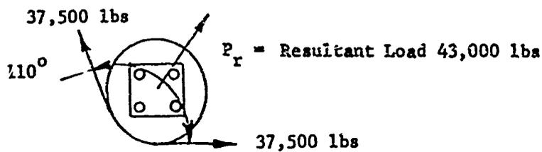
2-1/2" diameter tube in double shear, wall thickness 1/8"
