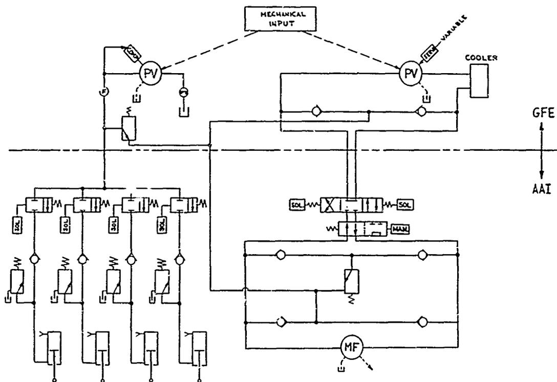
Figure 23. Dual Hydraulic System Schematic
