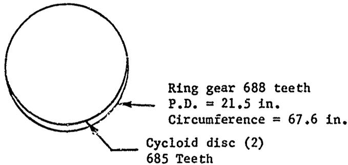
33% of the teeth on each of the two cycloid discs are in engagement at all times. Number of teeth in engagement =  $(.33)(685)(2) = 452$  teeth.
