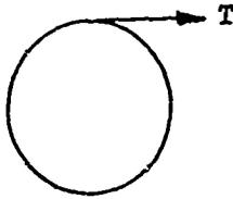
**M.S. = + .10** Crushing of drum based on the compressive yield strength of 5056-H18 aluminum.
