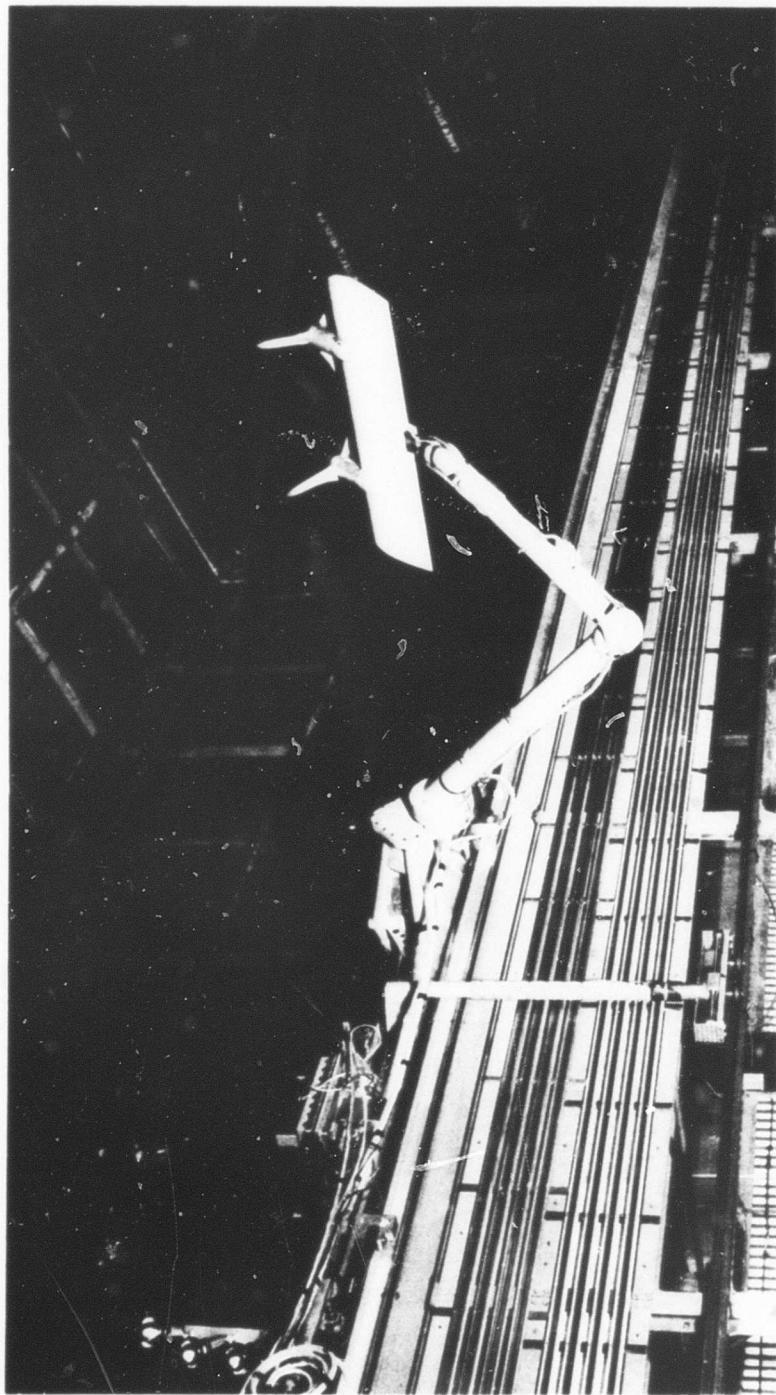
Figure 1. Model Installation in 30-by-30-Foot Test Section of the Princeton Dynamic Model Track Facility
