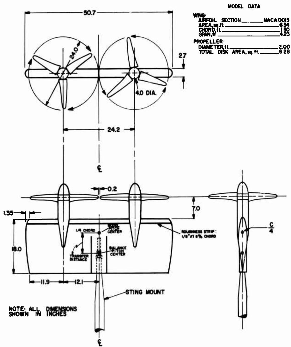
Figure 3. Tilt-Wing/Twin Propeller Model Configuration
