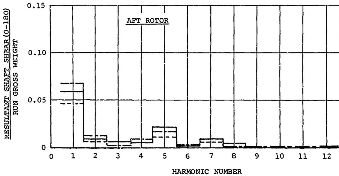
Figure 90. Harmonic Content of Typical Shaft Shear Data.
