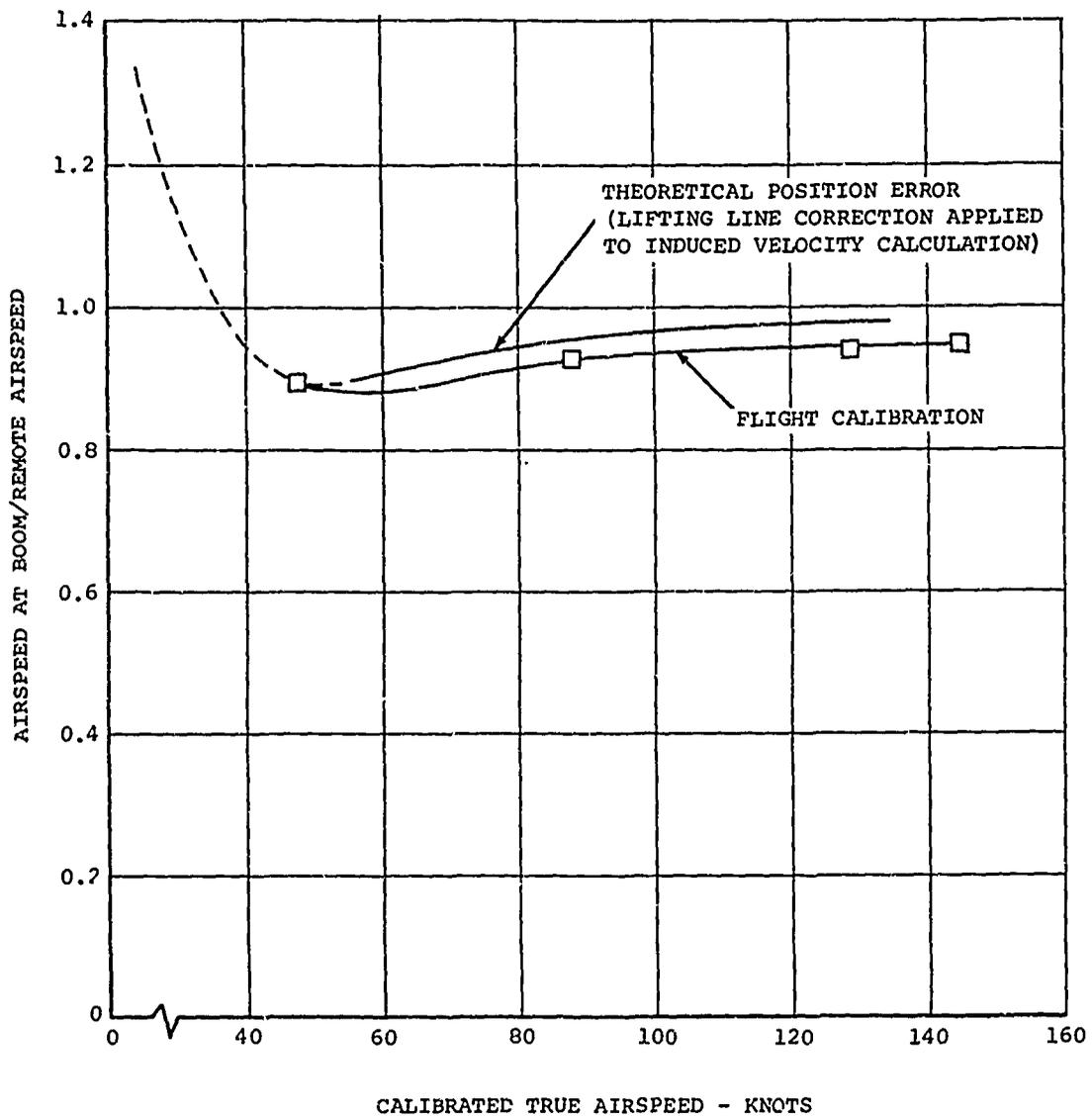
Figure 20. Comparison of Theoretical and Experimental Position Error Variation with Airspeed.
