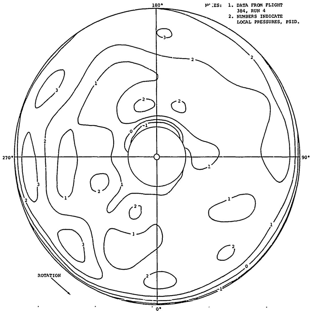
Figure 40. Contour Plot of Airload Pressures at 9-Percent Chord of the Forward Rotor at 108 Knots.
