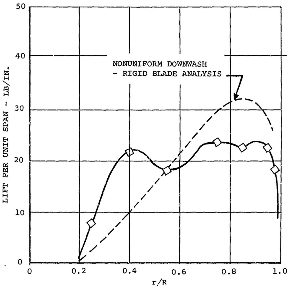
Figure 107. Comparison of Theoretical and Measured Average Loading of Forward Rotor.
