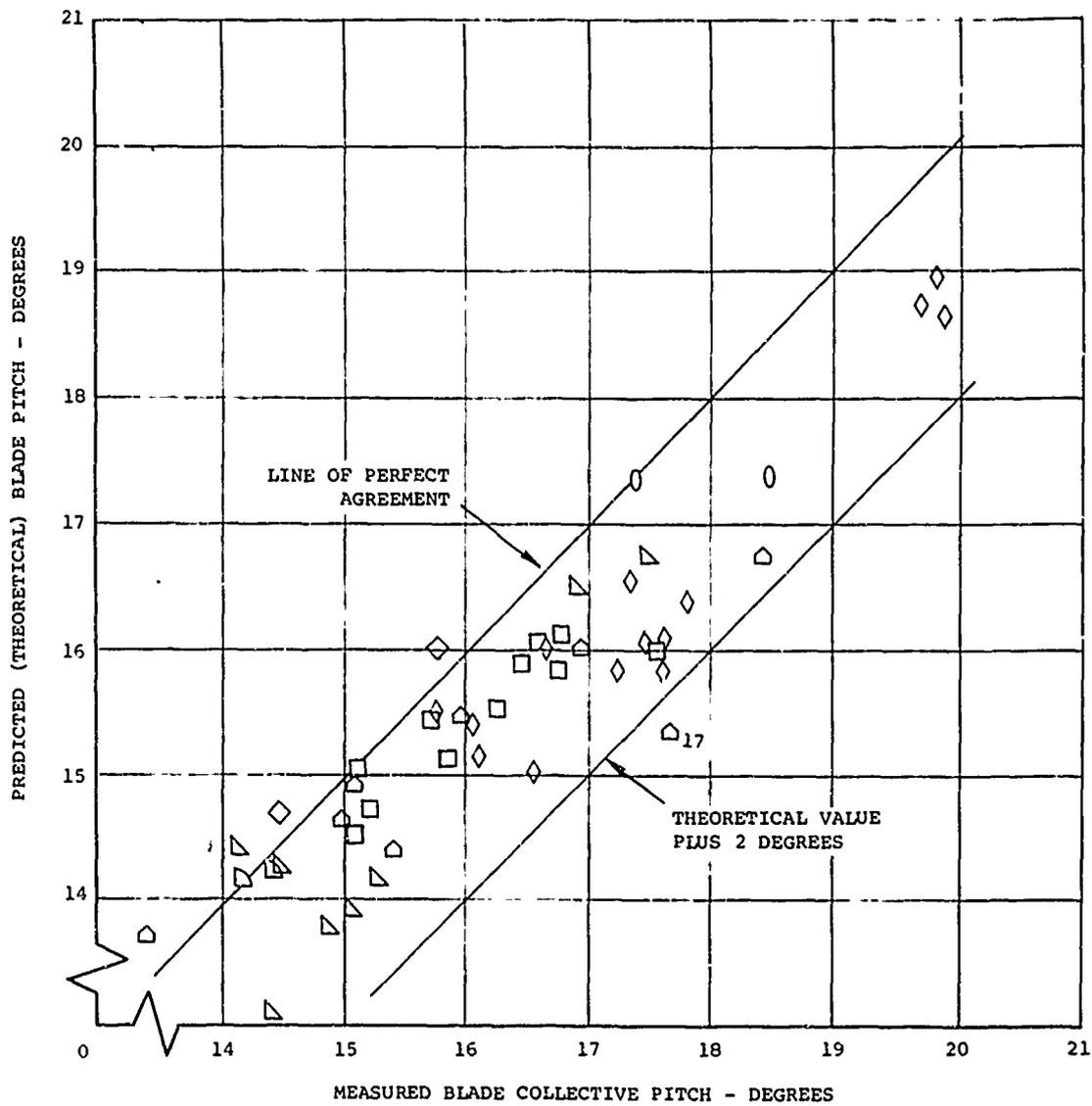
Figure 109. Comparison of Theoretical and Measured Collective Pitch Values for Forward Rotor.
