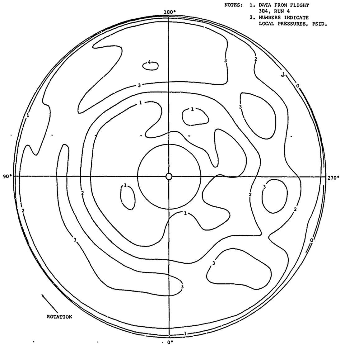
Figure 41. Contour Plot of Airload Pressures at 9-Percent Chord of the Aft Rotor at 108 Knots.
