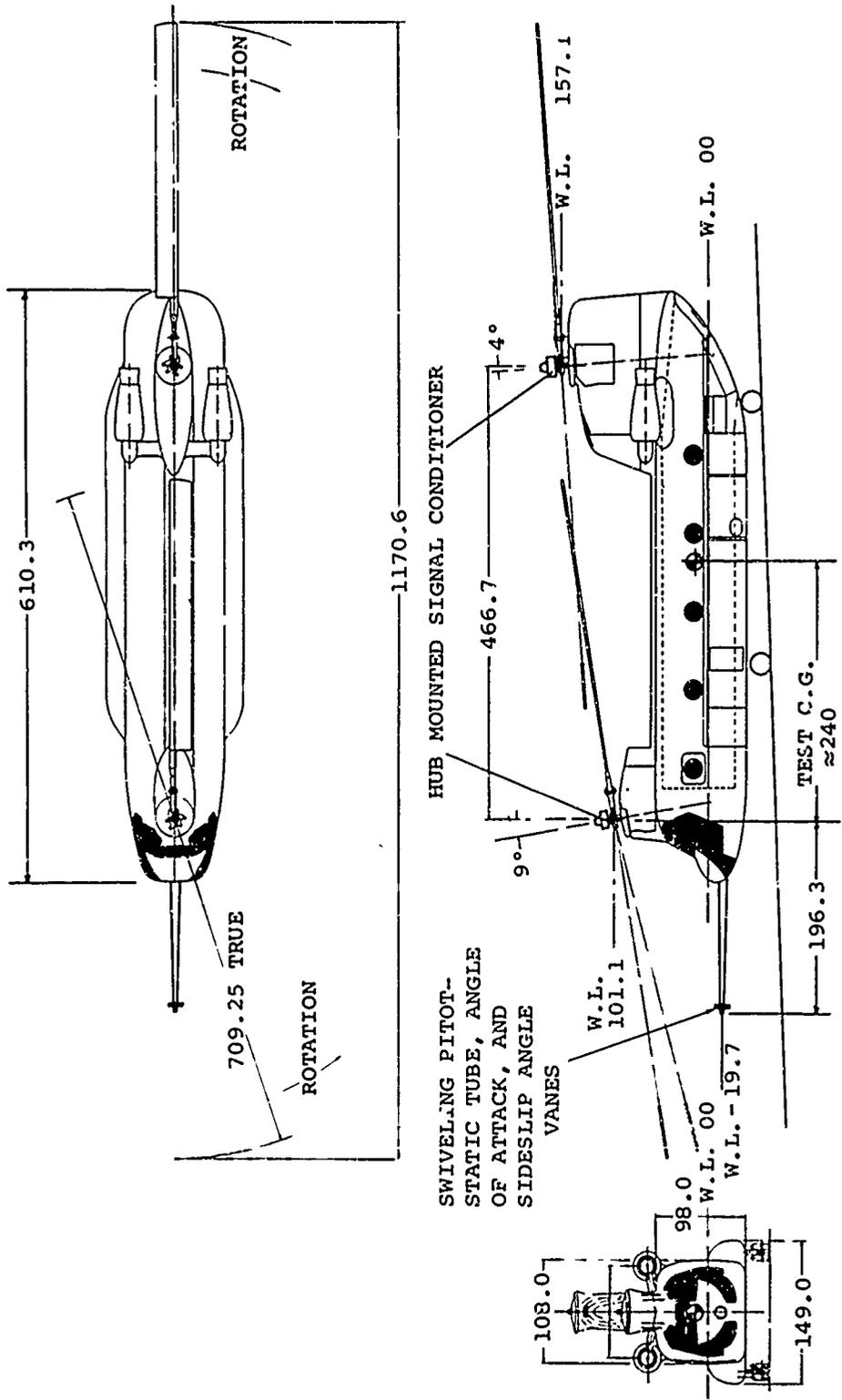
Figure 3. General Arrangement of CH-47A Helicopter as Tested.
