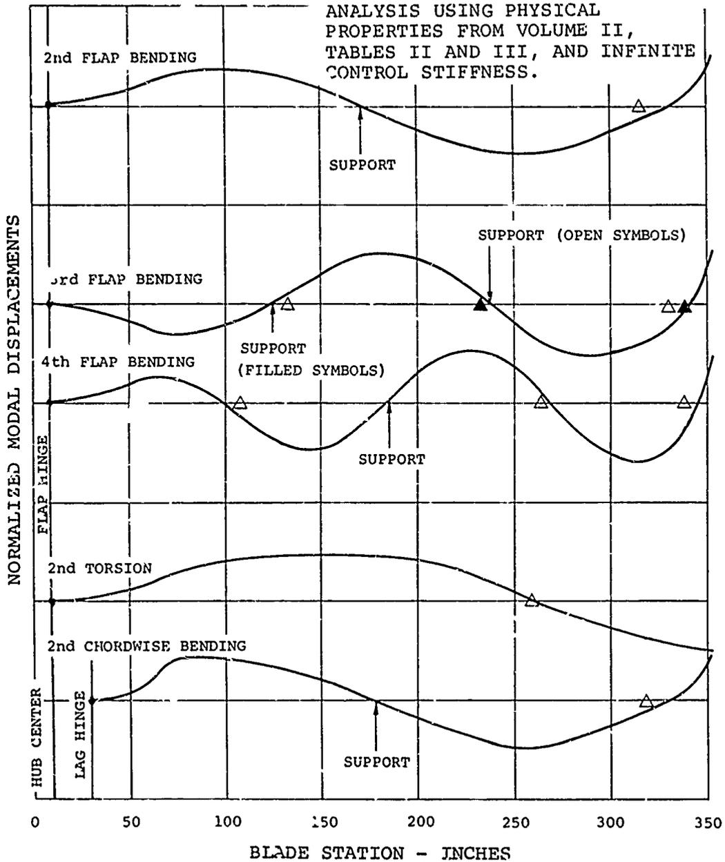
Figure 10. Calculated Blade Mode Shapes and Nodal Points Obtained in Nonrotating Blade Response Tests.
