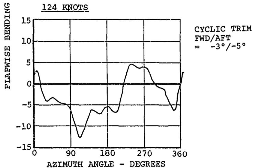
Figure 72. Azimuthal Variation of Blade Flap Bending Measured at 25-Percent Radius of the Forward Rotor.
