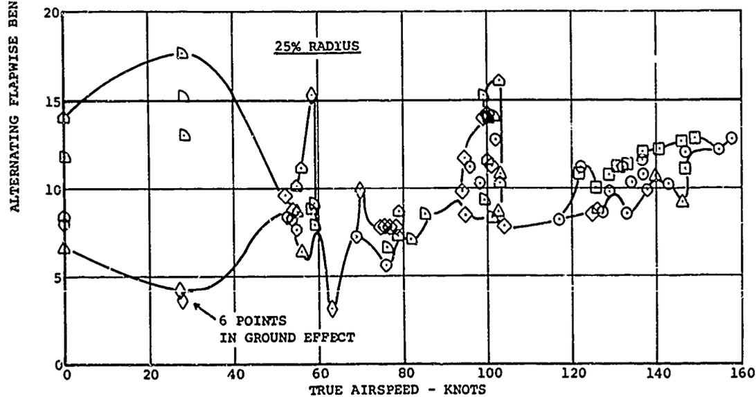
Figure 69. Effect of Airspeed on Alternating Flapwise Bending of Forward Rotor Blades in Level Flight.
