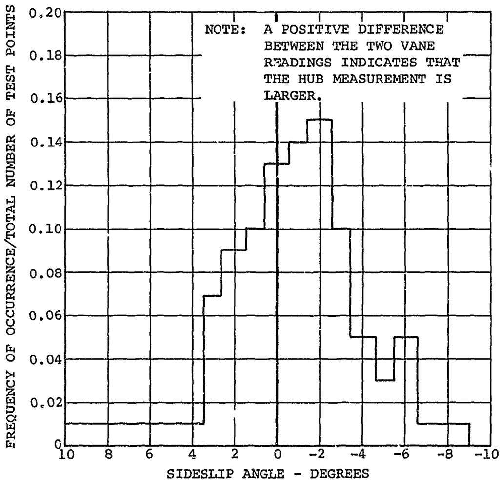
Figure 26. Comparison of the Two Sideslip Vane Readings Showing Statistical Confidence of Measurements.
