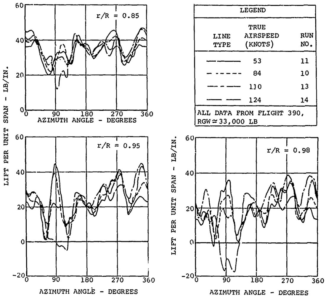
Figure 50. Typical Azimuthal Variation of Lift per Unit Span for Three Outboard Stations of Aft Rotor Blade.
