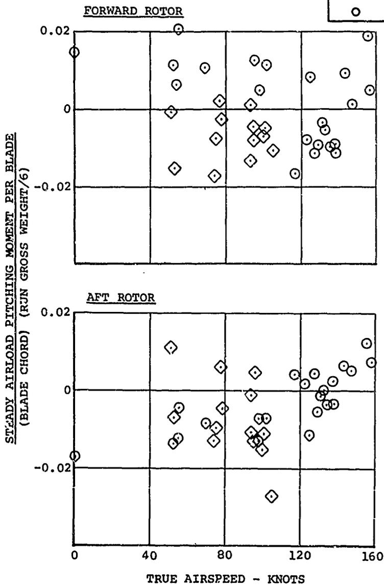
Figure 122. Azimuthal Averaged Rotor Blade Aerodynamic Pitching Moment Data.
