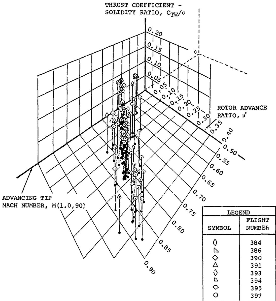
Figure 16. Perspective Illustration of Primary Parameters of Test Conditions.
