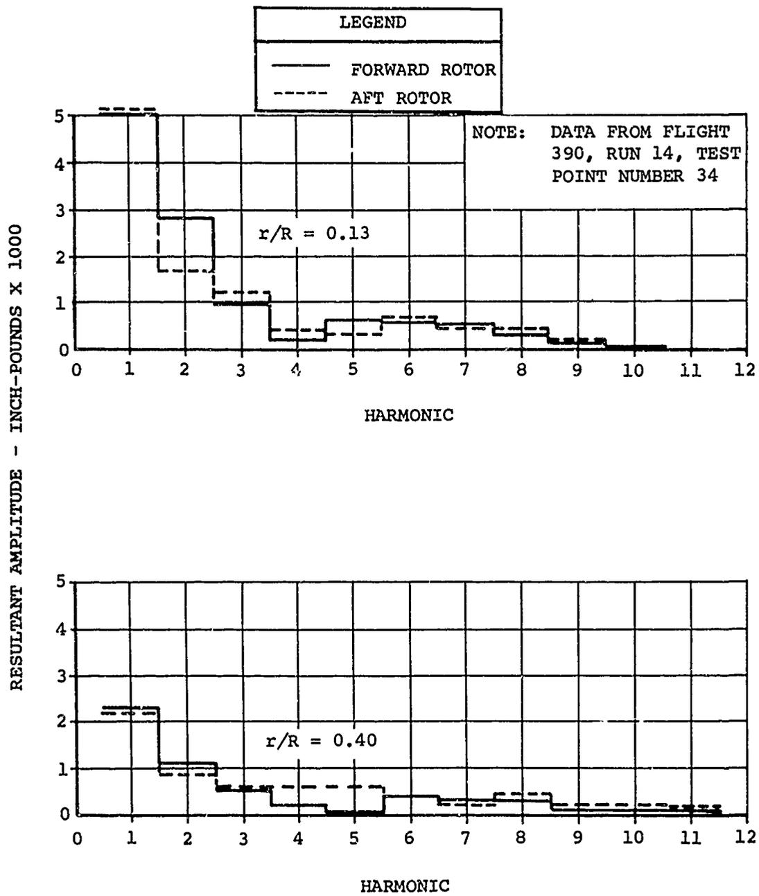
Figure 83. Harmonic Content of Torsional Moments at 124 Knots.
