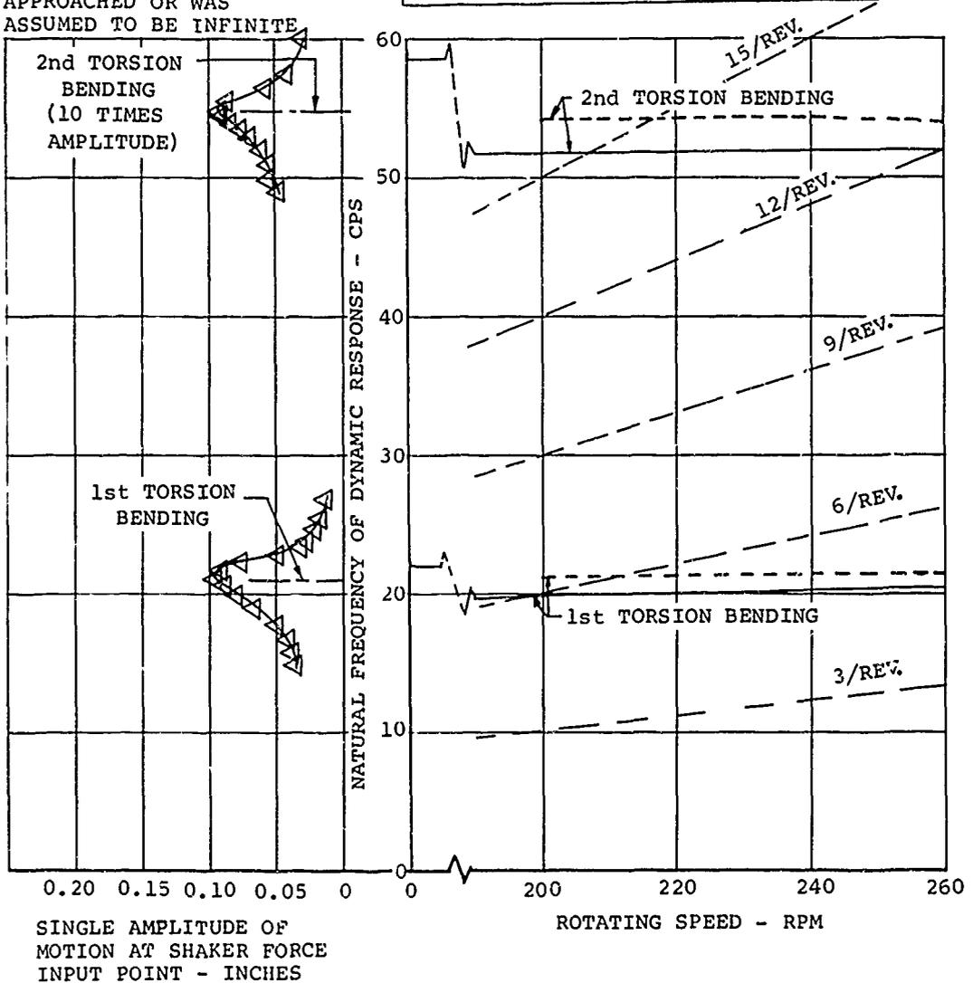
Figure 8. Comparison of Static Shake Test and Calculated Torsional Rotor Blade Natural Frequencies.
