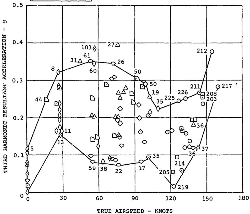
Figure 91. Third Harmonic Cockpit Vibration of Test Aircraft in Level Flight.
