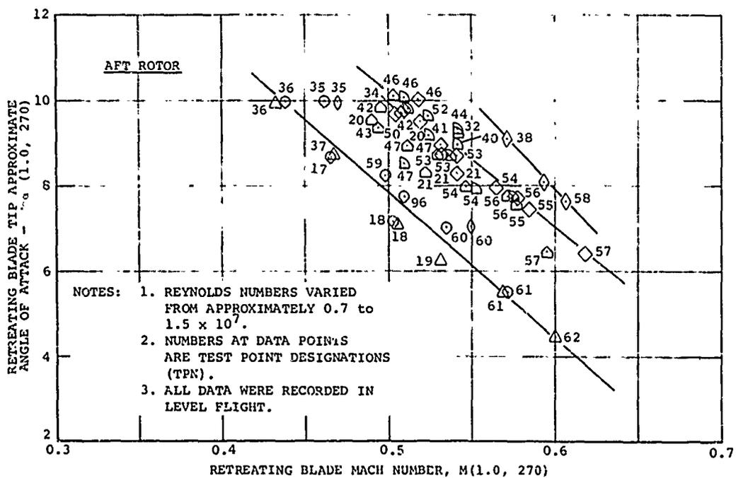
Figure 17. Retreating Blade Tip Operating Conditions Tested.
