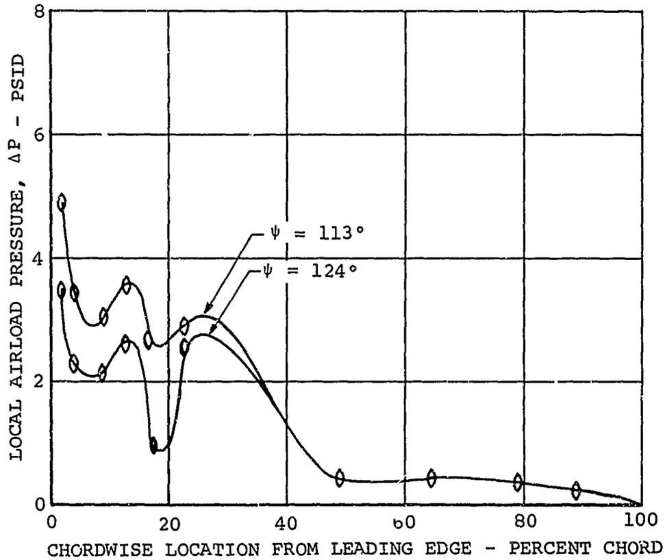
Figure 44. Typical Chordwise Pressure Distributions of Aft Rotor When in Proximity of Forward Rotor Tip Vortex.
