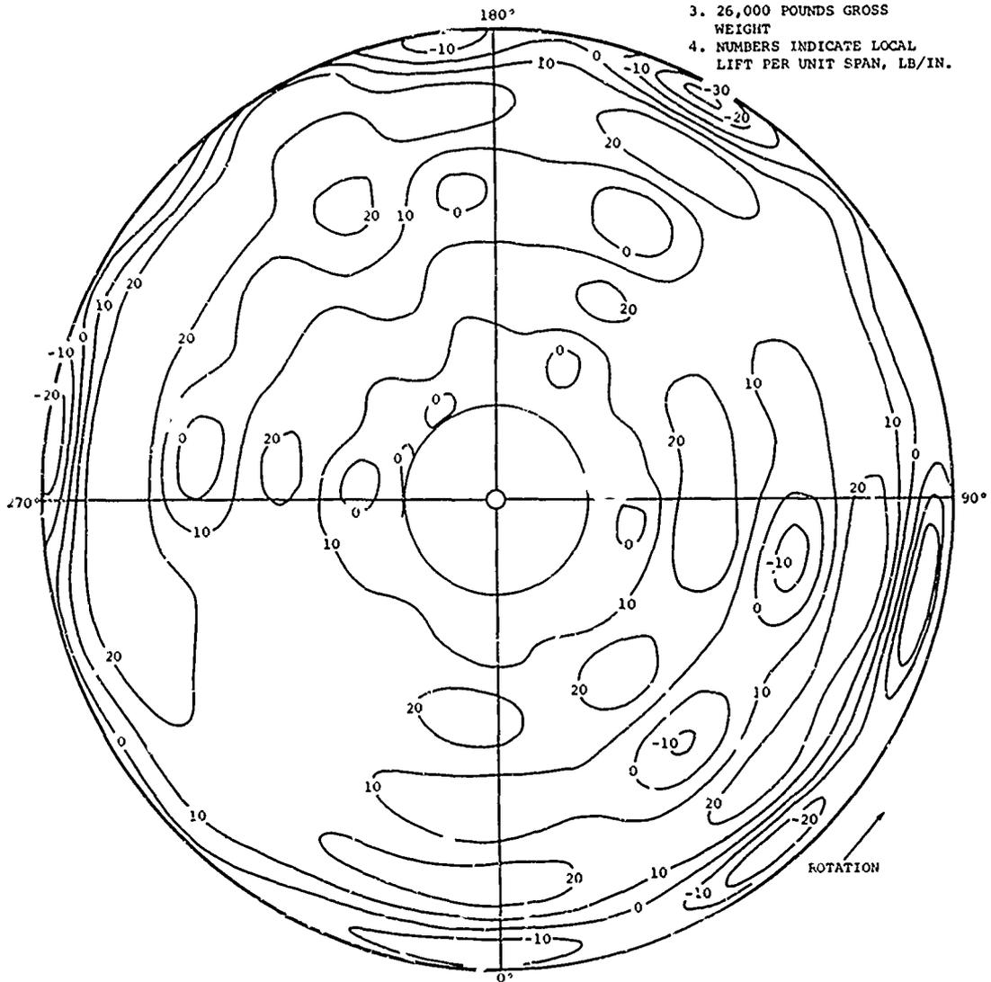
Figure 51. Contour Plot of Lift per Unit Span for Forward Rotor at 108 Knots.
