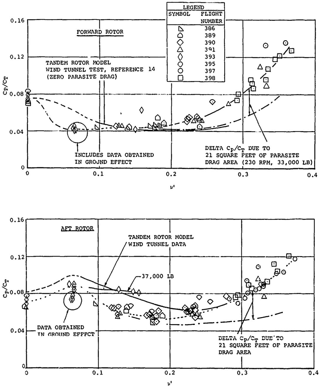
Figure 94. Nondimensional Rotor Performance of Test Aircraft.
