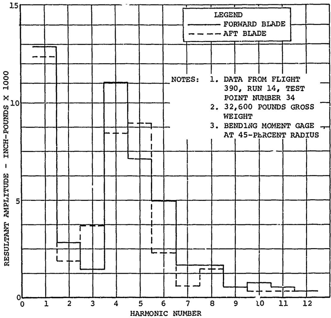
Figure 82. Harmonic Content of Chordwise Blade Bending Moments at 124 Knots.
