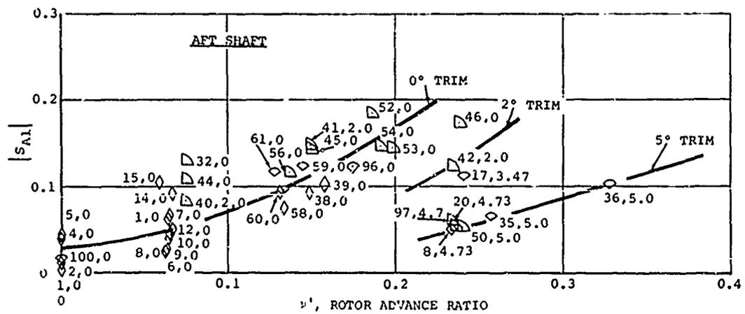
Figure 88. First Harmonic Shaft Shear Data Measured in Level Flight.
