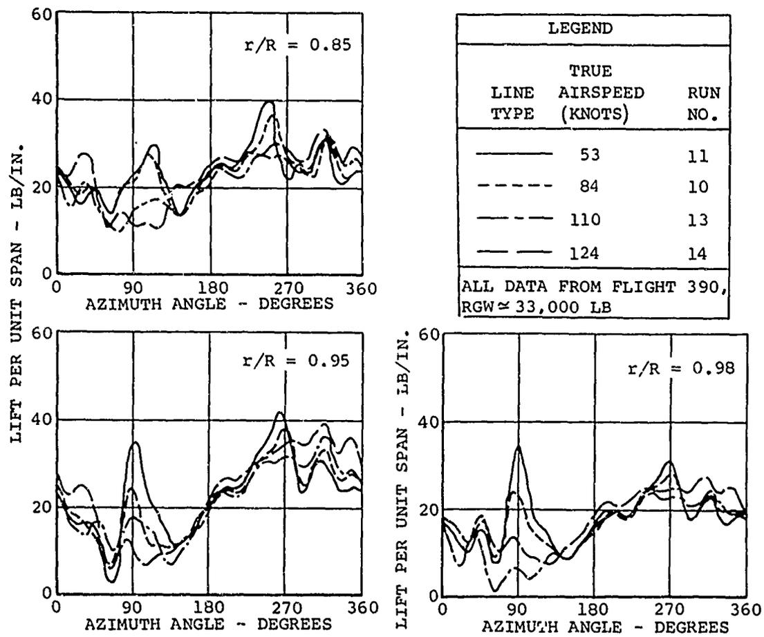
Figure 49. Typical Azimuthal Variation of Lift per Unit Span for Three Outboard Stations of Forward Rotor Blade.
