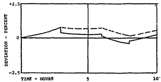
Figure 28. Drift Corrections Achieved in Ground Functional Testing.
