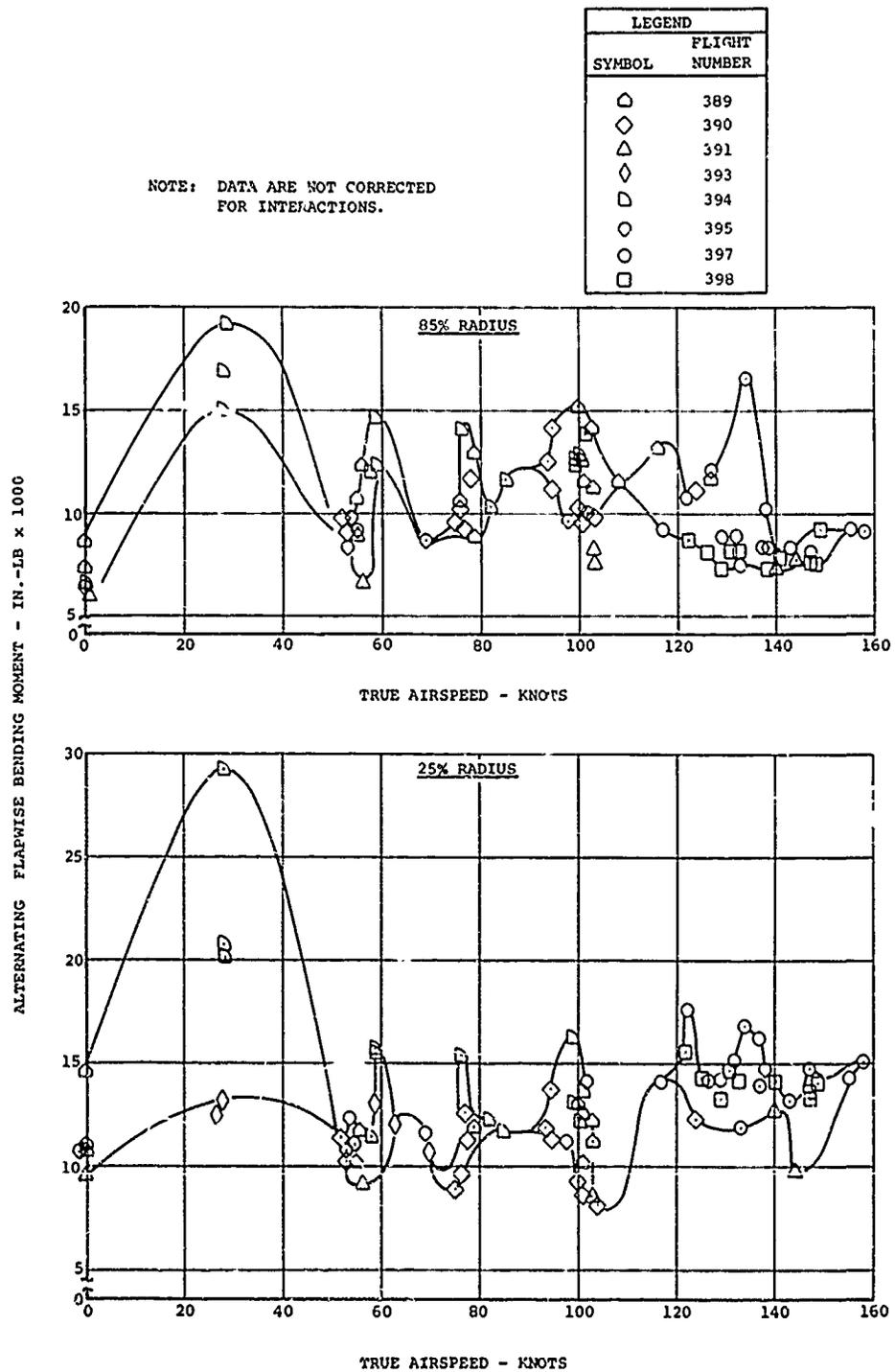
Figure 70. Effect of Airspeed on Alternating Flapwise Bending of Aft Rotor Blades in Level Flight.
