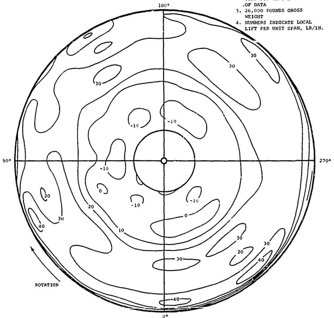
Figure 52. Contour Plot of Lift per Unit Span for Aft Rotor at 108 Knots.
