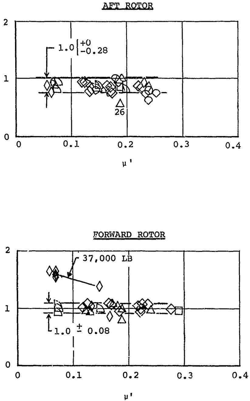
Figure 111. Effect of Advance Ratio on Prediction of Rotor Shaft Torque by Uniform Downwash-Rigid Blade Analysis.
