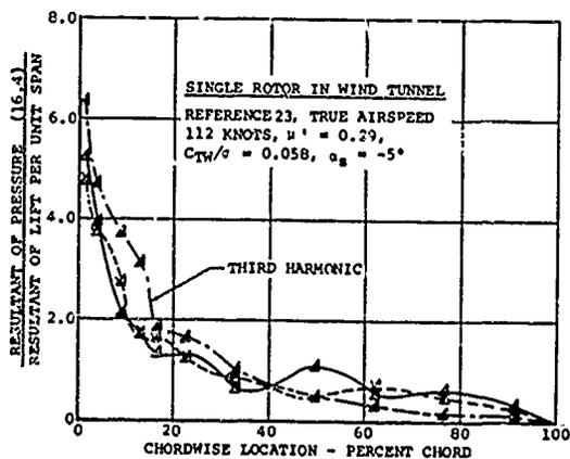
Figure 117. Comparison of Chordwise Loading Harmonics of Other Airloads Programs with Forward Rotor Data.
