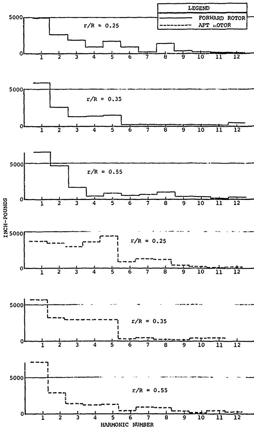
Figure 74. Harmonic Content of Flapwise Bending Moments at 124 Knots Airspeed and 33,000 Pounds Gross Weight.
