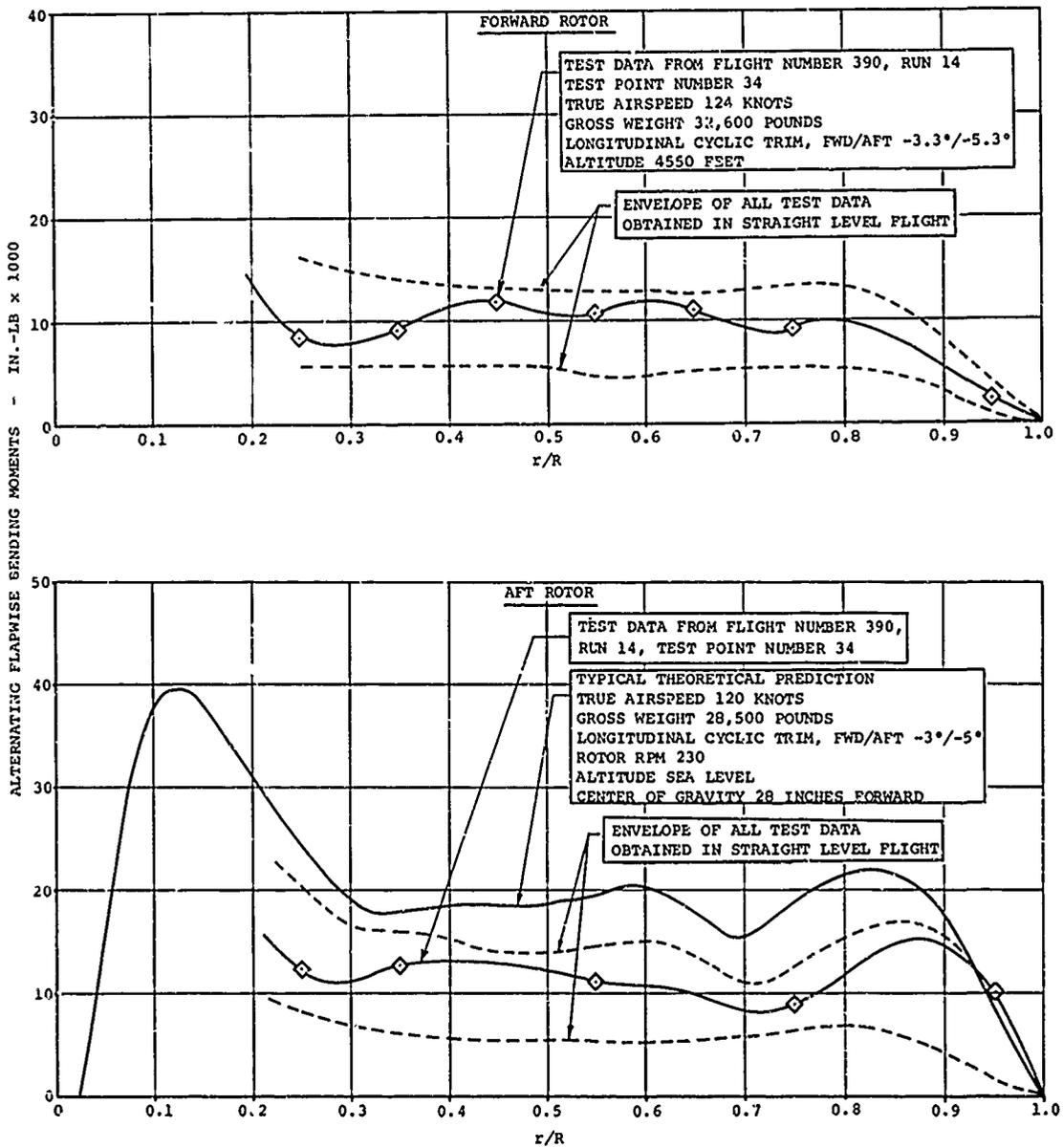
Figure 68. Typical Variation with Radius of Alternating Flapwise Bending Data Obtained in Level Flight.
