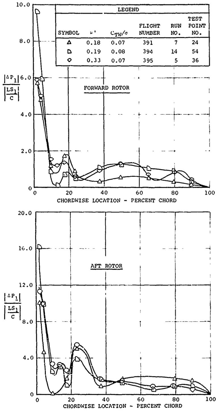
Figure 45. Chordwise Distribution of First Harmonic Airloads at 85 Percent of the Blade Radius for Three Tests.
