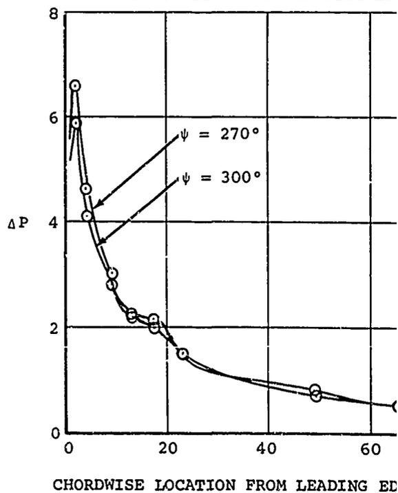
Figure 43. Chordwise Pressure Distributions Measured on Retreating Side of Rotor Disk at 108 Knots Airspeed and 26,000 Pounds Gross Weight.
