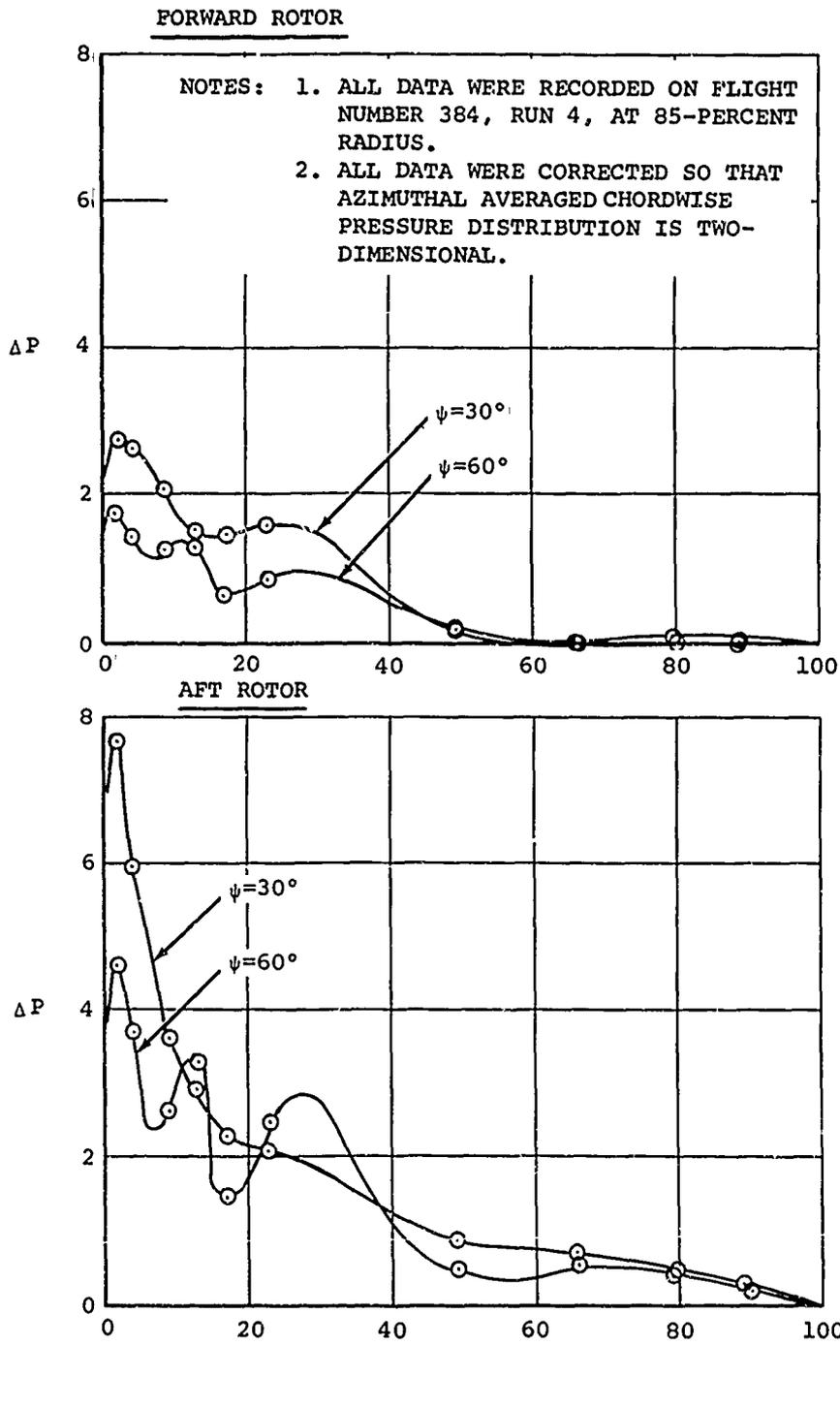
Figure 42. Chordwise Pressure Distributions Measured on Advancing Side of Rotor Disk at 108 Knots Airspeed and 26,000 Pounds Gross Weight.
