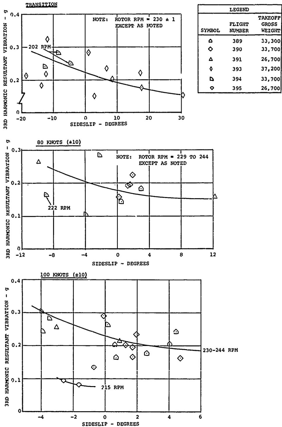
Figure 92. Effect of Sideslip on Cockpit Vibration.
