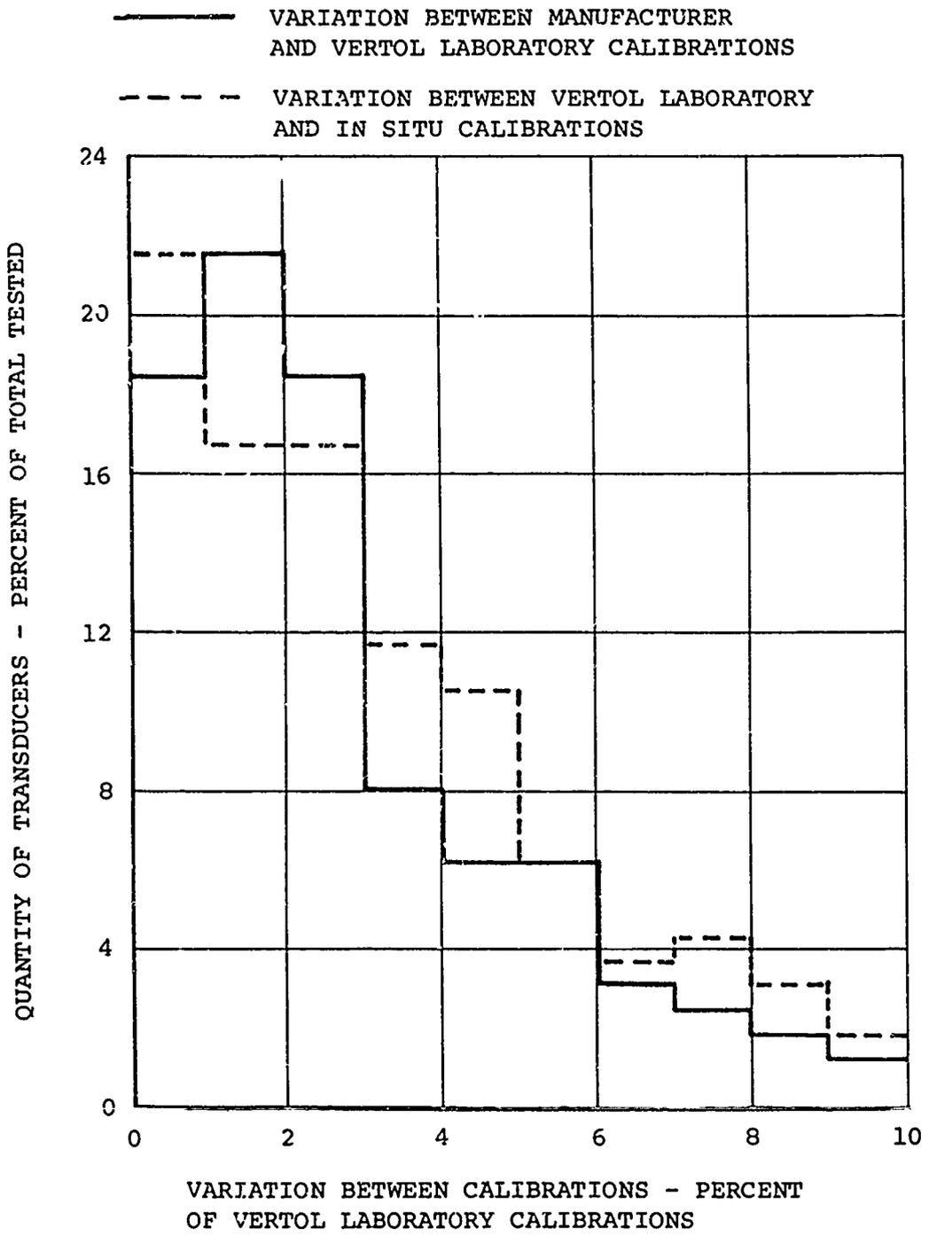
Figure 38. Repeatability of Airloads Pressure Transducer Calibrations.
