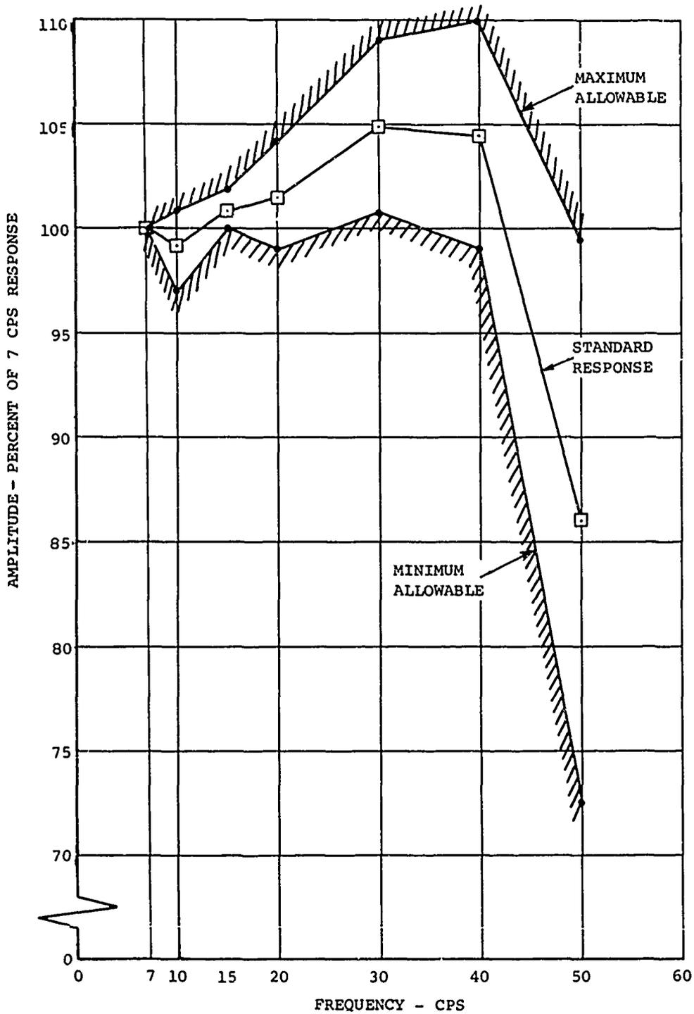
Figure 30. Frequency Response of Airframe Accelerometers.
