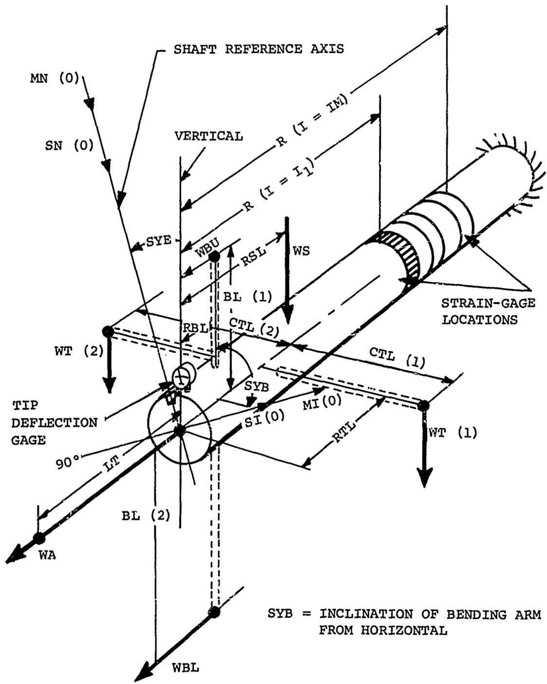
Figure 21. Illustration of Geometry and Notation of Rotor Shaft Calibration Problem.
