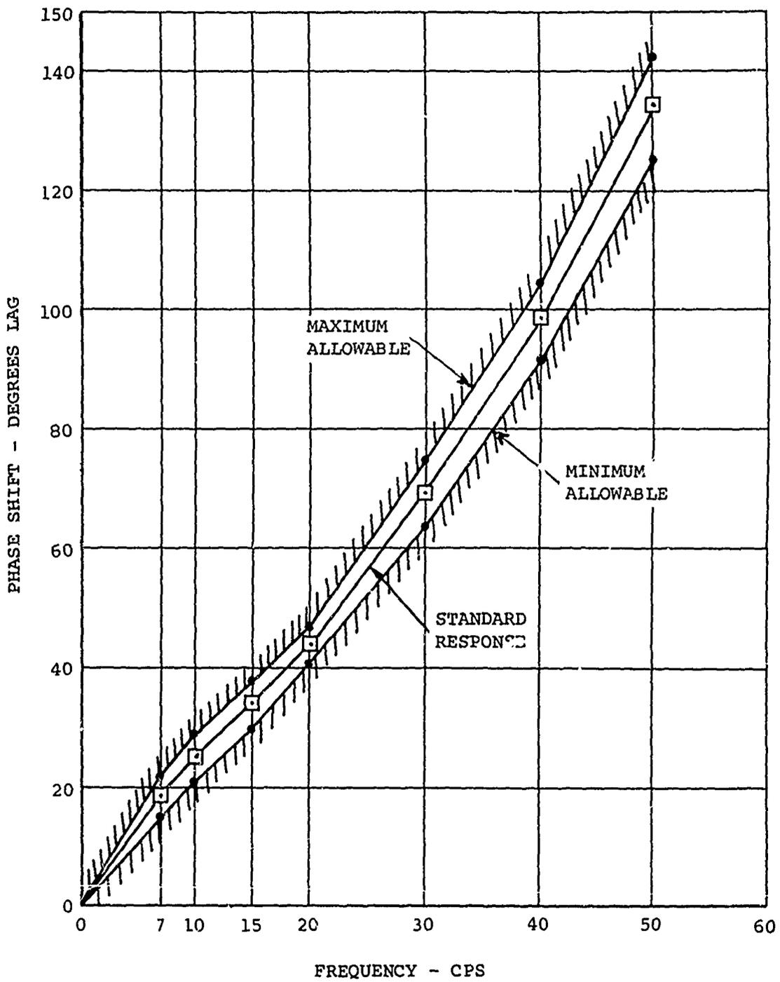
Figure 31. Phase Lag of Airframe Accelerometer Output Signals.
