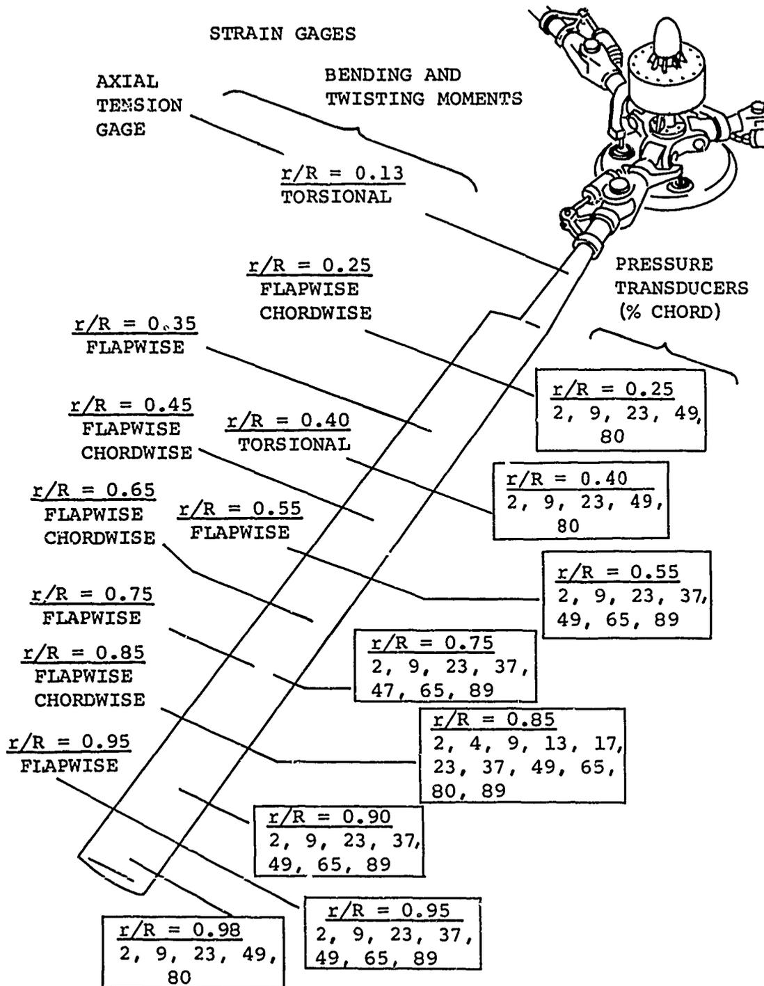
Figure 1. Installation of Rotor Blade Instrumentation.
