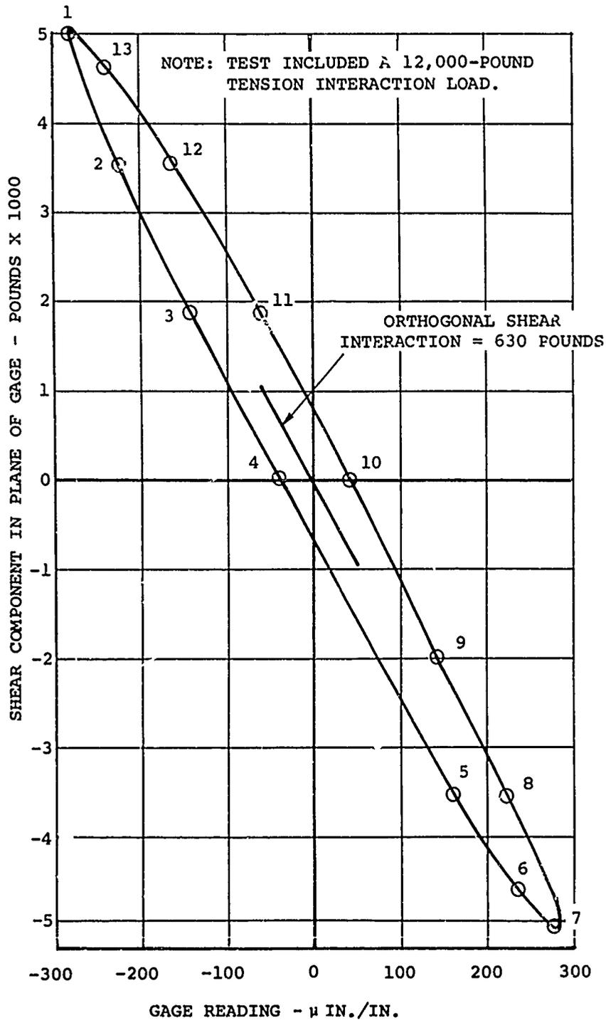
Figure 26. Interactions of 0-180 Shear Gage Readings Due to an Orthogonal Shear on the Forward Shaft.
