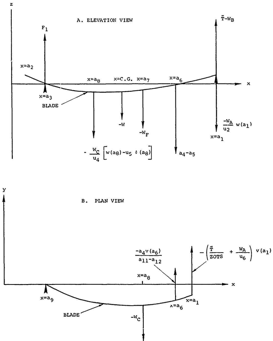
Figure 43. Blade Loads and Geometry of Application.
