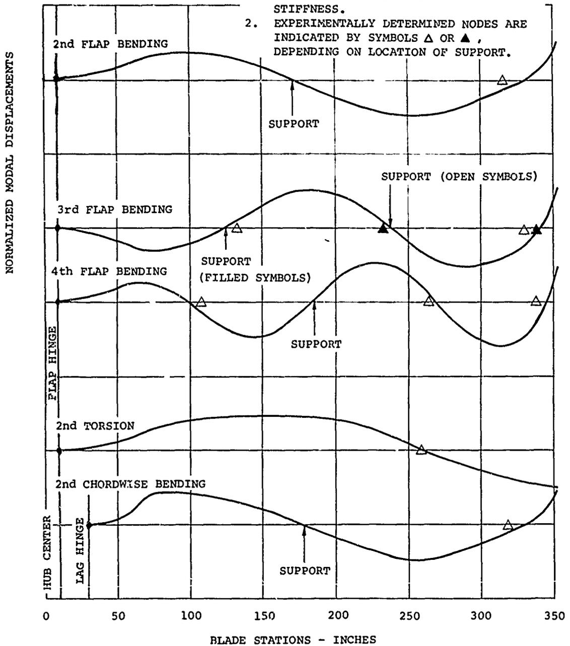
Figure 33. Nodal Points Obtained in Nonrotating Blade Response Tests.
