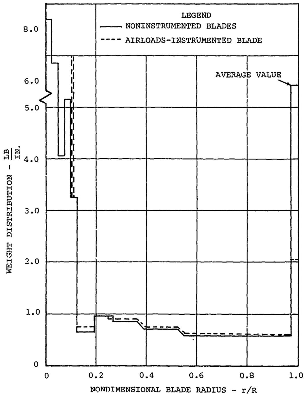
Figure 6. Spanwise Mass Distribution of Instrumented Blade and Noninstrumented Blades.
