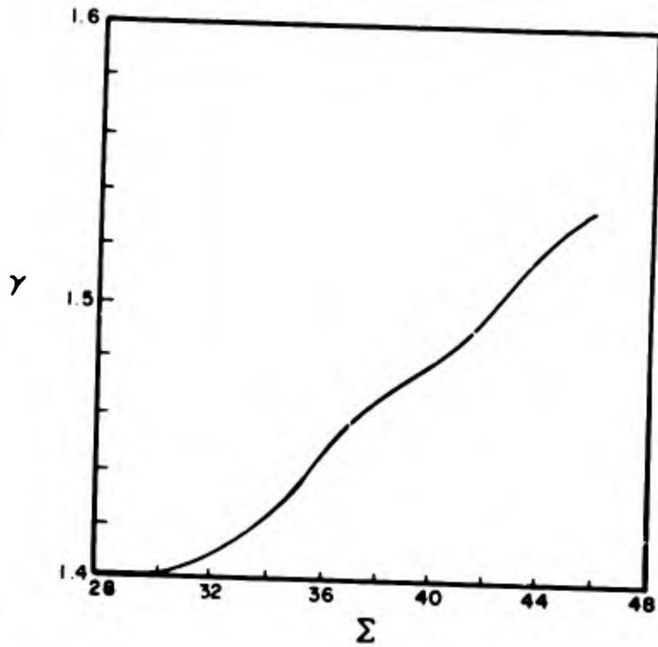
Figure 1. Frozen Ratio of Specific Heats vs the Nozzle Nonequilibrium Similarity Parameter for Air Expansions
