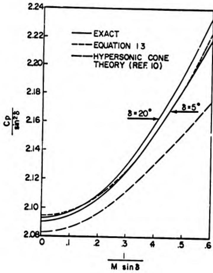
Figure 4. Comparison of Small Disturbance Approximations With Exact Cone Flow Solutions (Perfect Gas,  $\gamma = 1.4$ )
