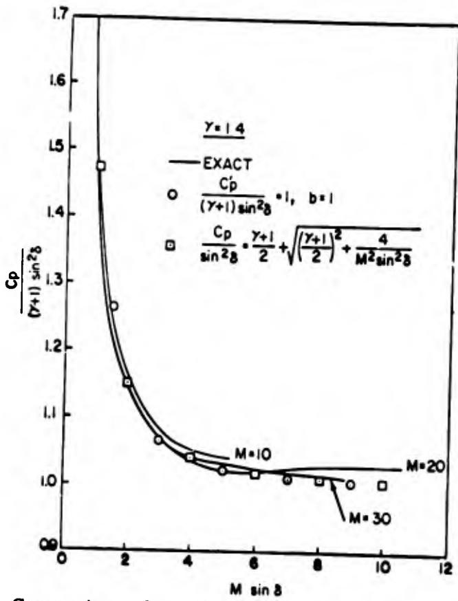
Figure 2. Comparison of Small Disturbance Approximations With Exact Wedge Flow Solutions (Perfect Gas,  $\gamma = 1.4$ )
