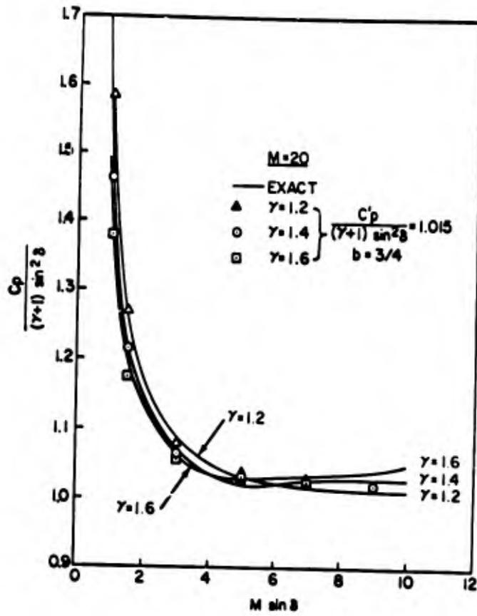
Figure 3. Comparison of the Hypersonic Small Disturbance Rule for Wedge Flow With Variable  $\gamma$
