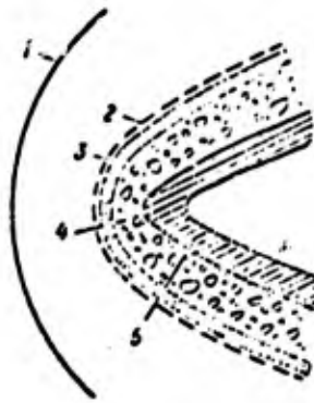
Figure 2. Schematic diagram of the ablation process. 1 - shock wave; 2 - gas boundary layer; 3 - molten layer; 4 - porous carbonized layer; 5 - layer in which decomposition takes place
