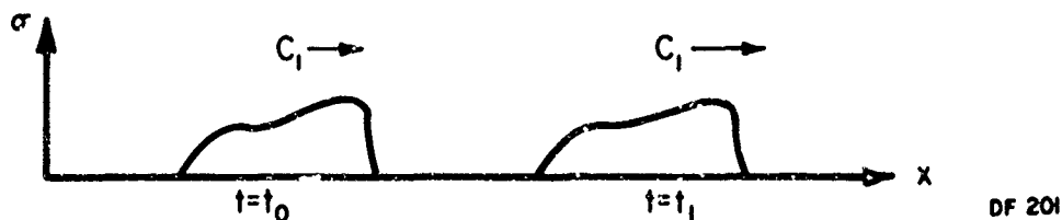
FIGURE B-1. UNDISTORTED STRESS-PULSE PROPAGATION
