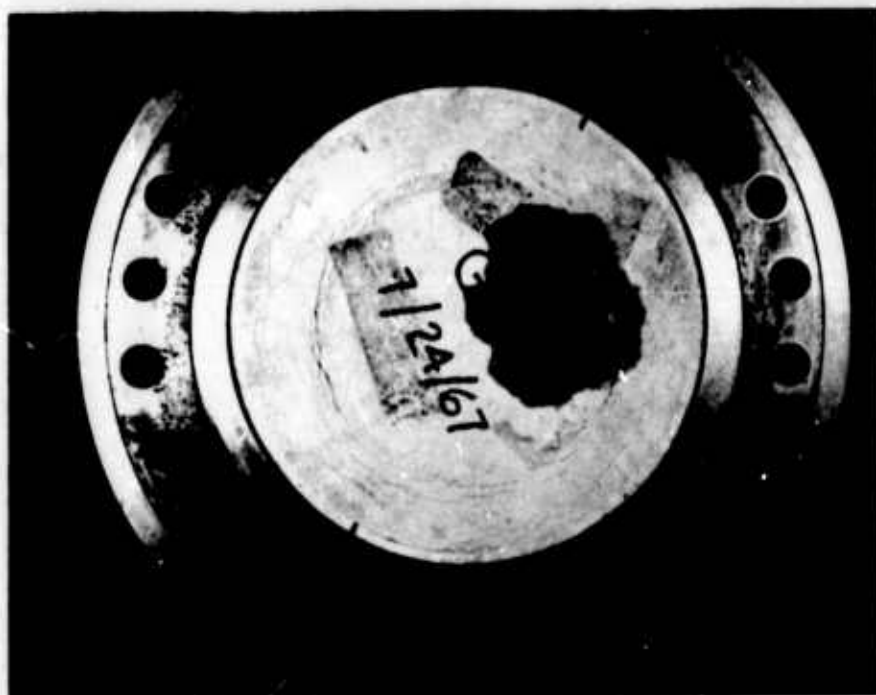
Fig. 5.69 Slab G-7, Deformation of Top Surface
