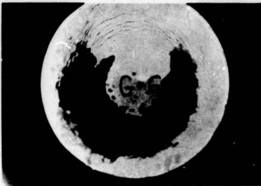
Fig. 5.66 Slab G-6, Deformation of Top Surface
