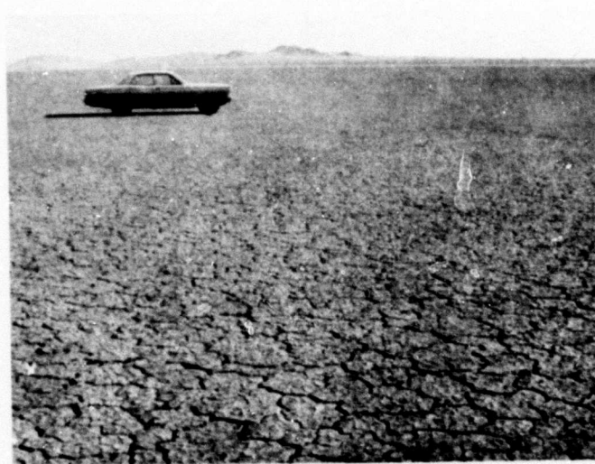
Figure 17. Identical Location as Figure 16, November 1966. Depressions had been completely filled following flooding of the playa during the 1965-66 winter.
