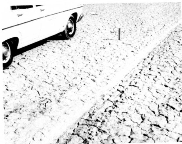
Figure 14. Hard, Dry Crust in November 1966 at Same Location as Figure 13. Surface was flooded the previous winter. Note virtual absence of wheel ruts. Vestiges of tracks from previous rutting in 1962 are visible, however.
