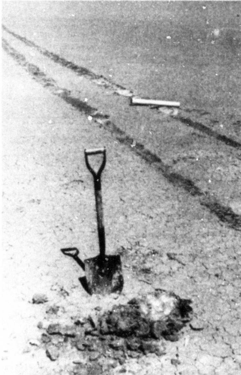
Figure 17. Surface of Soft Powdery Silt, 37 km Southeast of Moalleman. Rut is 7 cm deep. View east along anticlinal dome of Miocene, 2 September 1966.
