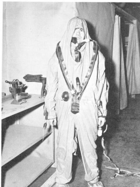
Fig. 6. British Submarine Escape Immersion Suit with Thermistor and EEG Leads Emerging Through Neck Area.
