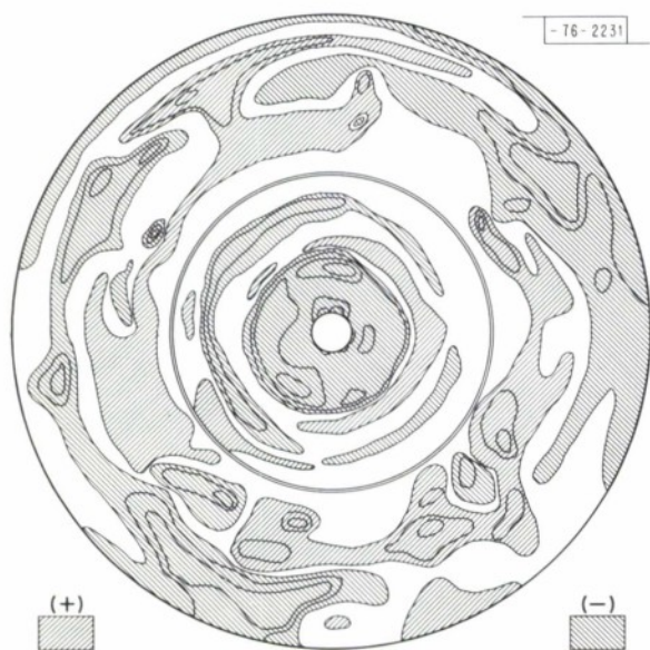
Fig. 20. Deviations from best-fit paraboloid before adjustment (rms = 0.037 inch; contours of deviation at 0.025-inch intervals).
