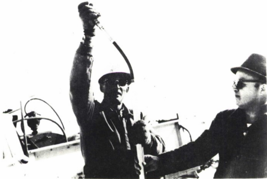
Figure 7 Eastman Drift Indicator Being Prepared For Use
