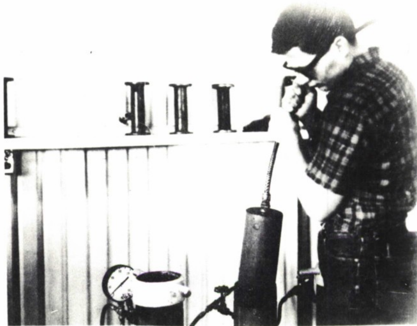
Figure 16 Seismometer Being Placed in Pressure Test Chamber
