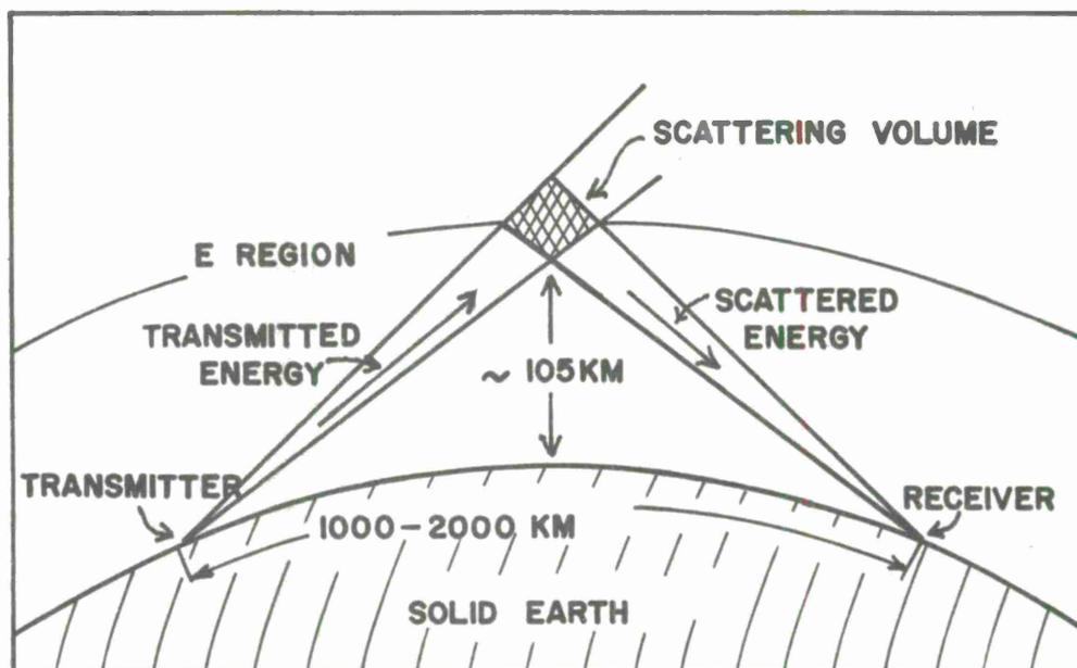
Figure 78. The scattering volume viewed in common by transmitter and receiver in an ionosscatter communication mode.
