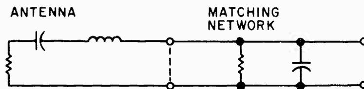
FIGURE 27. MONOPOLE ANTENNA AND BASIC MATCHING NETWORK EQUIVALENT CIRCUIT
