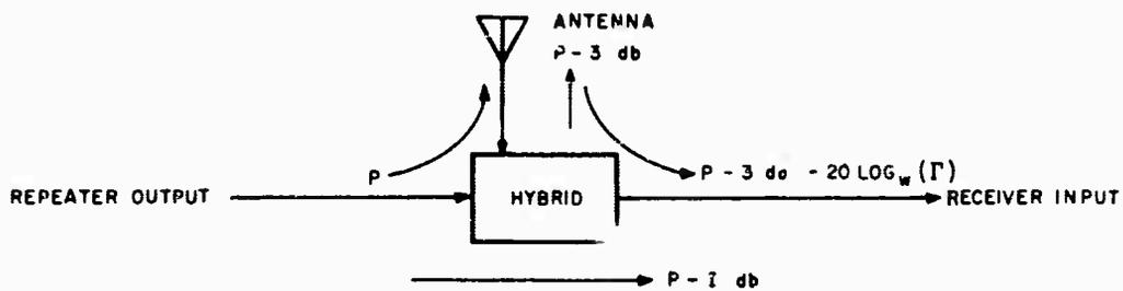
FIGURE 23. HYBRID FOR COUPLING REPEATER OUTPUT TO RECEIVER INPUT
