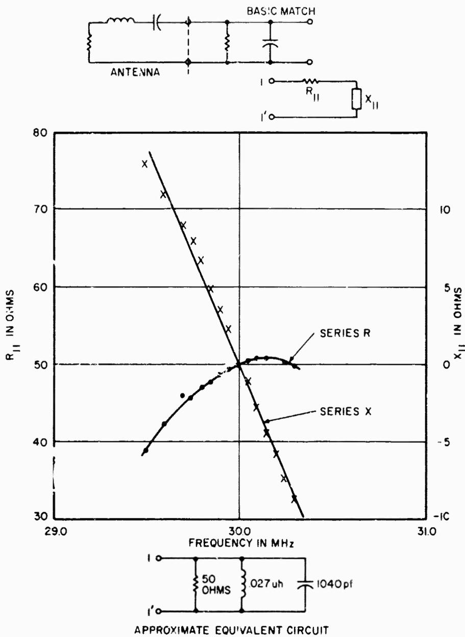
FIGURE 29. RESISTANCE AND REACTANCE VS FREQUENCY FOR MONOPOLE ANTENNA AND BASIC MATCHING NETWORK
