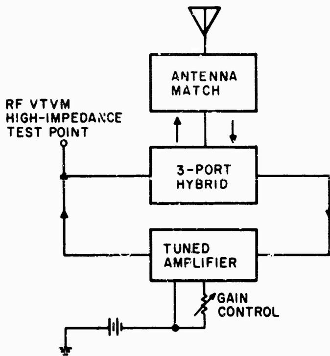
FIGURE 2. WIDE-BAND REPEATER, BLOCK DIAGRAM
