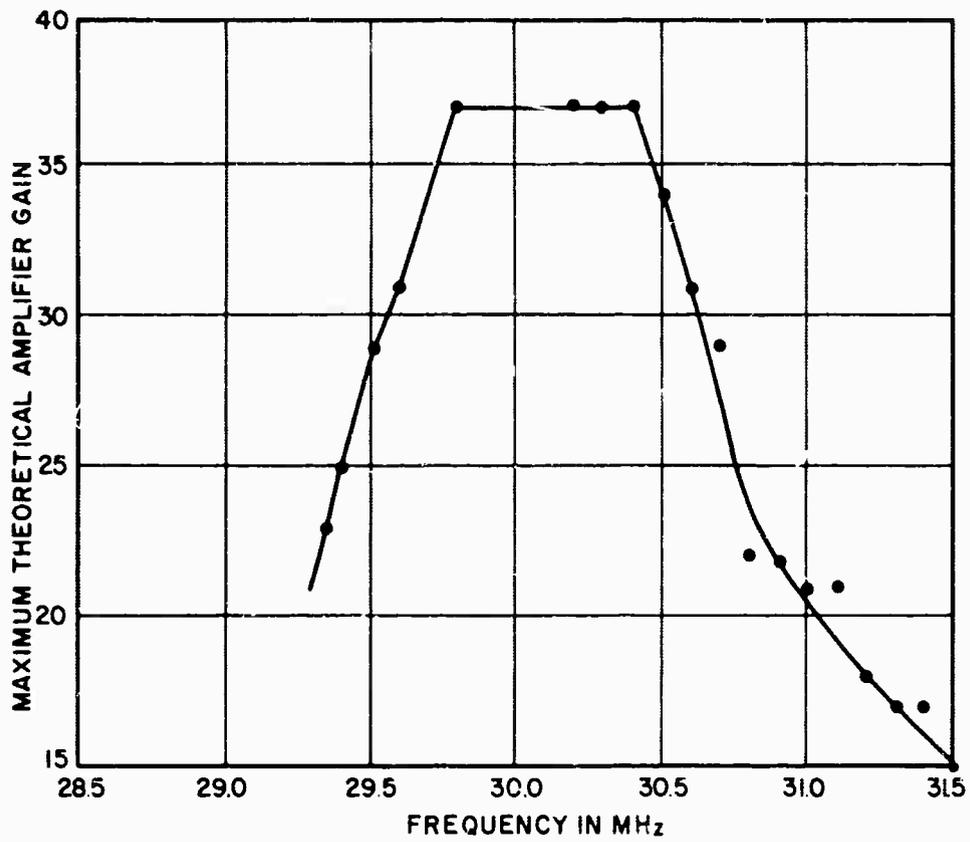
FIGURE 33. MAXIMUM AMPLIFIER GAIN VS FREQUENCY (BASED ON ANTENNA VSWR MEASUREMENTS)
