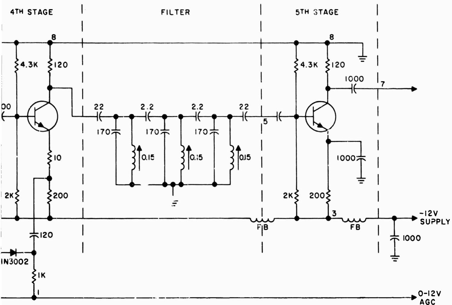
FIGURE 17. MICROMINIATURE 30-MHz TUNED AMPLIFIER
