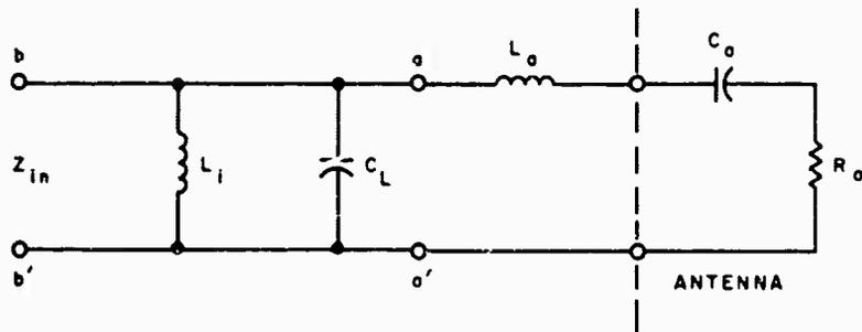
FIGURE 22. ANTENNA WITH DOUBLE-TUNED MATCHING SECTION
