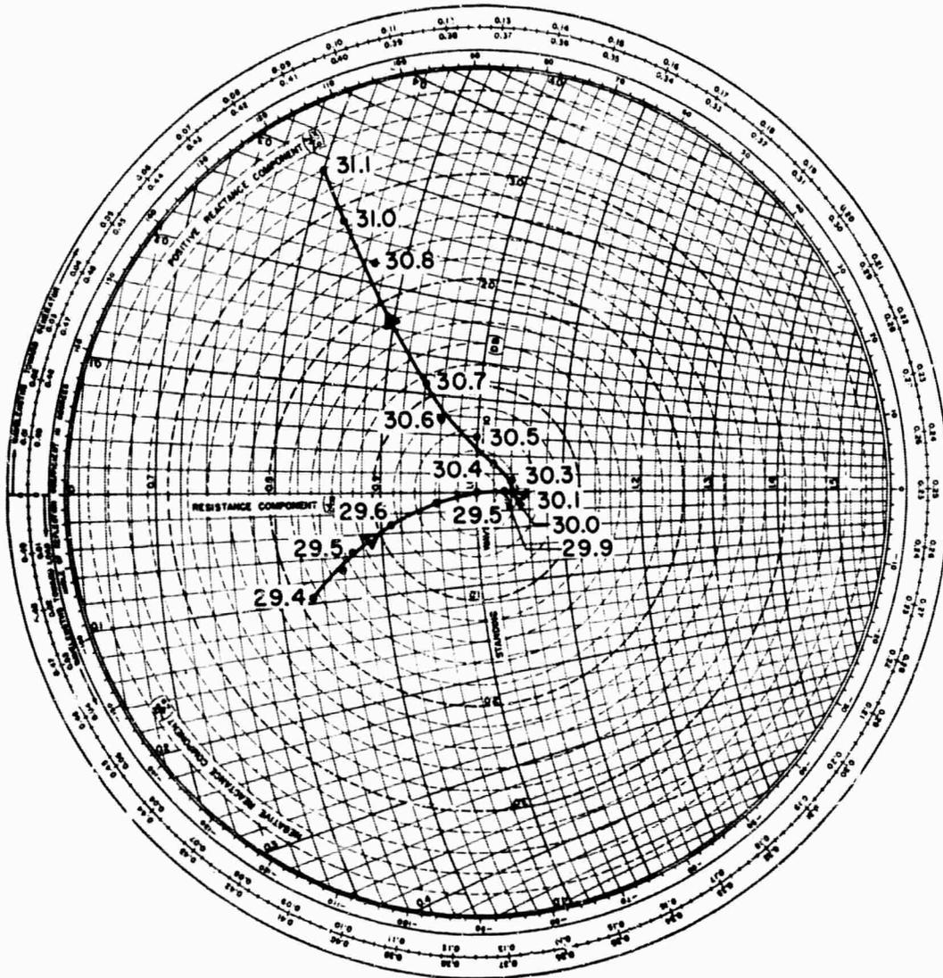
FIGURE 31. SMITH-CHART PLOT FOR MONOPOLE ANTENNA AND TWO-POLE MATCHING NETWORK VS FREQUENCY
