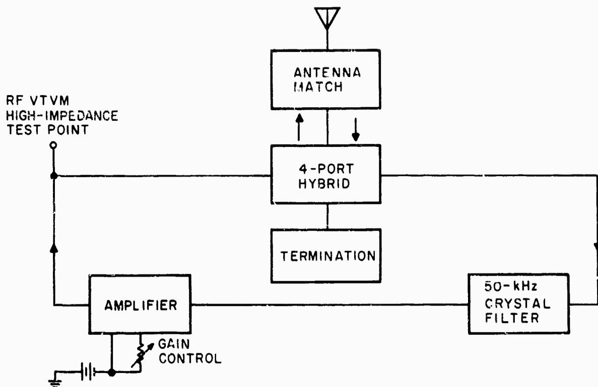
FIGURE 1. HIGH-GAIN REPEATER, BLOCK DIAGRAM
