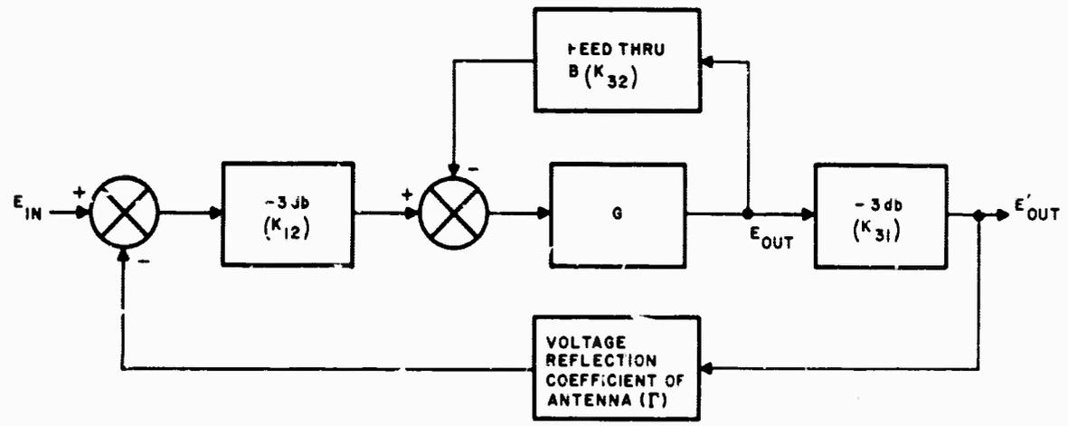
FIGURE 4. EQUIVALENT FLOW DIAGRAM
