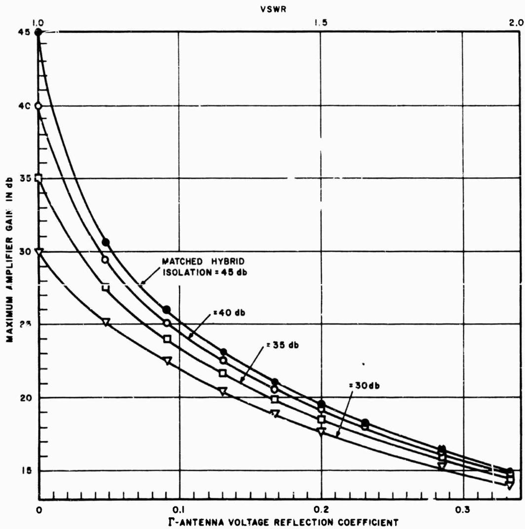
FIGURE 5. MAXIMUM REPEATER AMPLIFIER GAIN VS ANTENNA MISMATCH FOR  $F_1, F_1$  REPEATER
