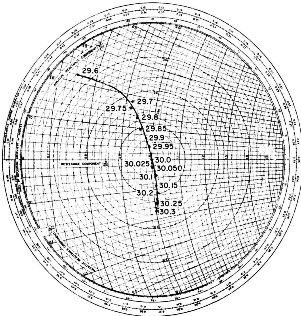
FIGURE 28. SMITH-CHART PLOT OF MONOPOLE ANTENNA AND BASIC MATCHING NETWORK VS FREQUENCY
