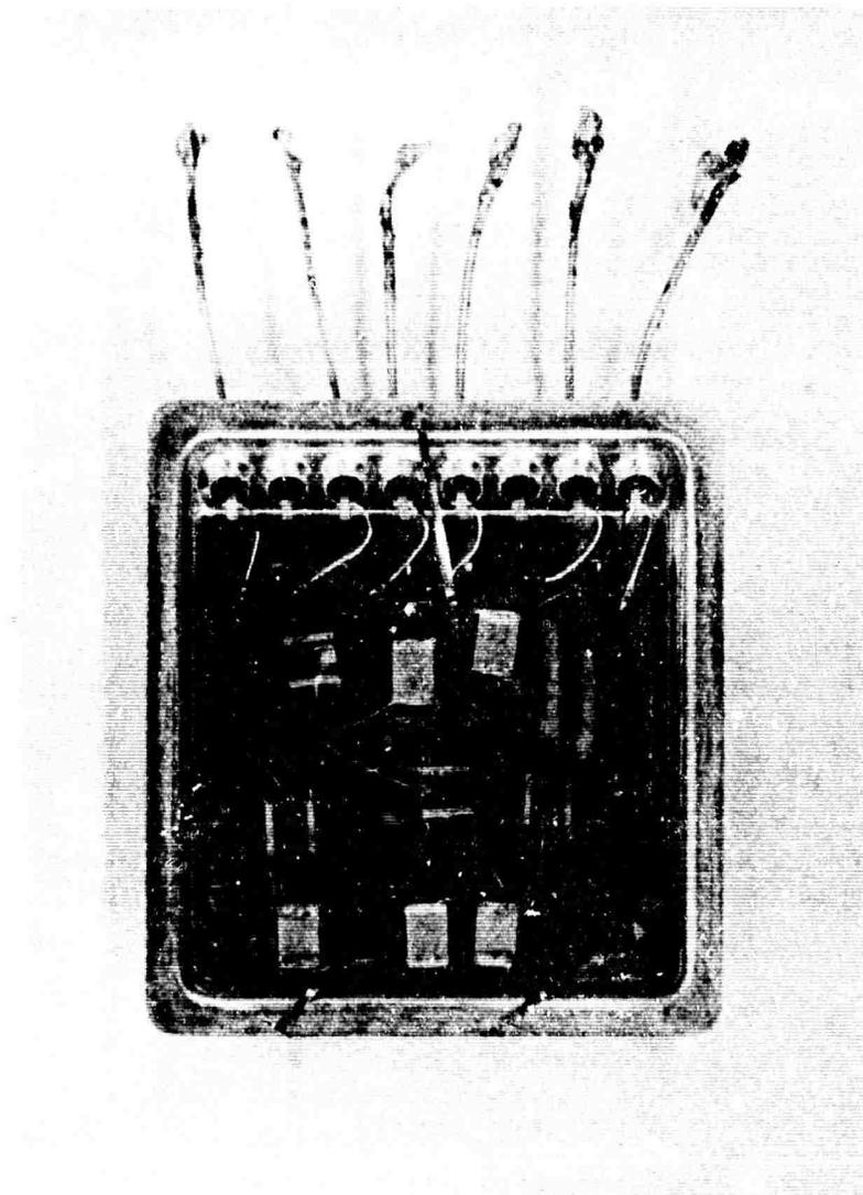
FIGURE 18. HIGH-GAIN MICROMINIATURE AMPLIFIER
