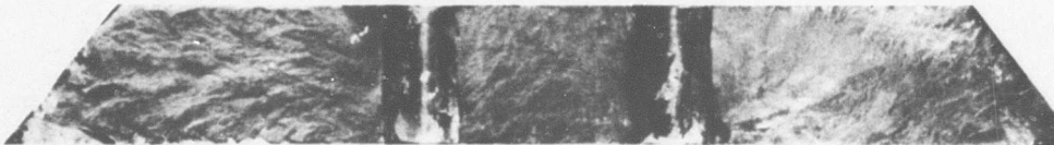
Figure 50. Typical Fracture Surface for Ti-6Al-6V-2Sn Cuff.
