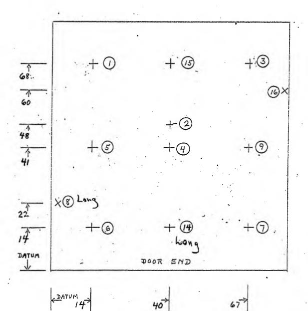
Notes: Thermocouples #16 and # 8 to be attached to inner skin on side walls as shown 40 inches from floor.
