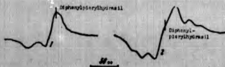
Fig. 1. EPR spectra of solutions of \text{H}_2\text{O} and \text{H}_2\text{O}_2 + n-propyl alcohol in water:
