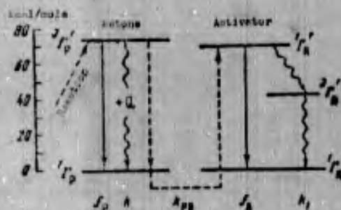
FIG. 1. Energy level diagram illustrating chemiluminescence in the reaction of oxidation of ethylenebenzene and transfer of energy to derivatives of anthracene. Rate constants of radiative (solid lines) and nonradiative transitions (wavy lines) and transfer (dotted lines) are designated.
