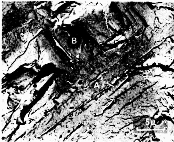
Fig. 3. Fractograph showing cleavage (A) in the single-phase hexagonal martensite of Ti-5Al-2.5Sn (2000 F/15 min/NQ). Ductile failure occurred at B.
