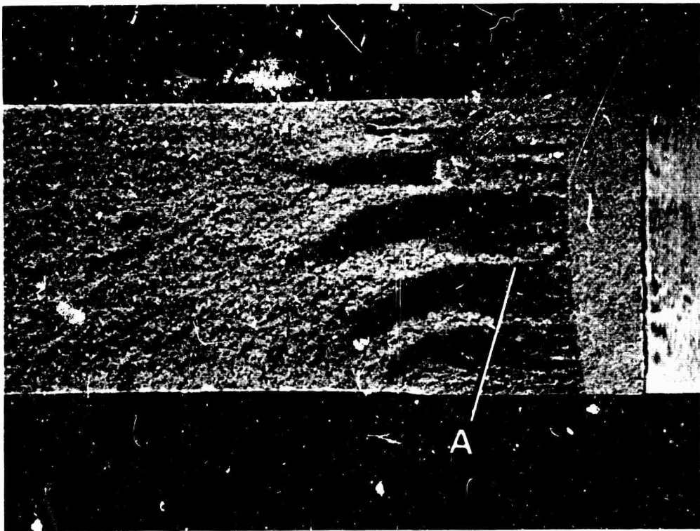
Fig. 1 Specimen Failed in 3% NaCl Solution, Showing Fatigue Crack, Slow Crack Growth, and Fast Fracture Regions. Magnification: 3X
