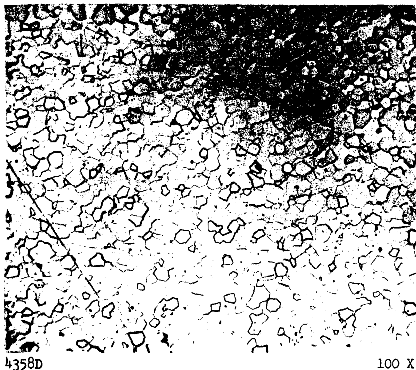
Figure 18. Cross Section of transparent section of forging FA-110 perpendicular to plane of pressing.
