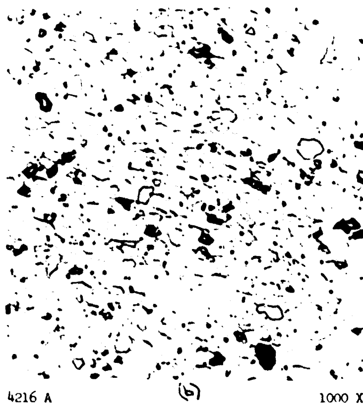
Figure 32. Microstructural texture in relatively low temperature press forged alumina (a) parallel, and (b) perpendicular to press forging direction.
