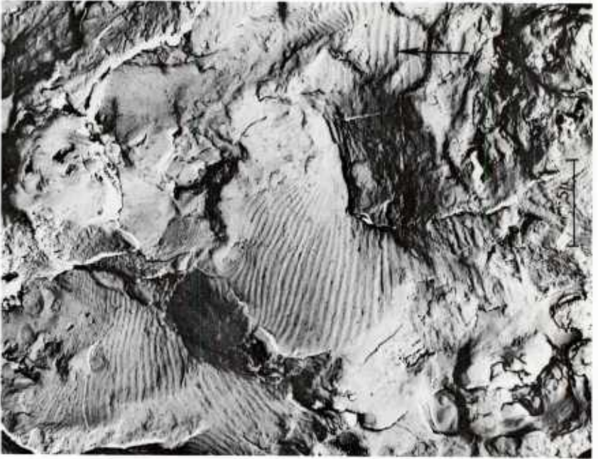
b. Regions of ductile striations and of brittle fracture at second-phase particles. / Photographs through the courtesy of Regis M. N. Pelloux; see Boeing Report DI-82-0169-RI (1963).
