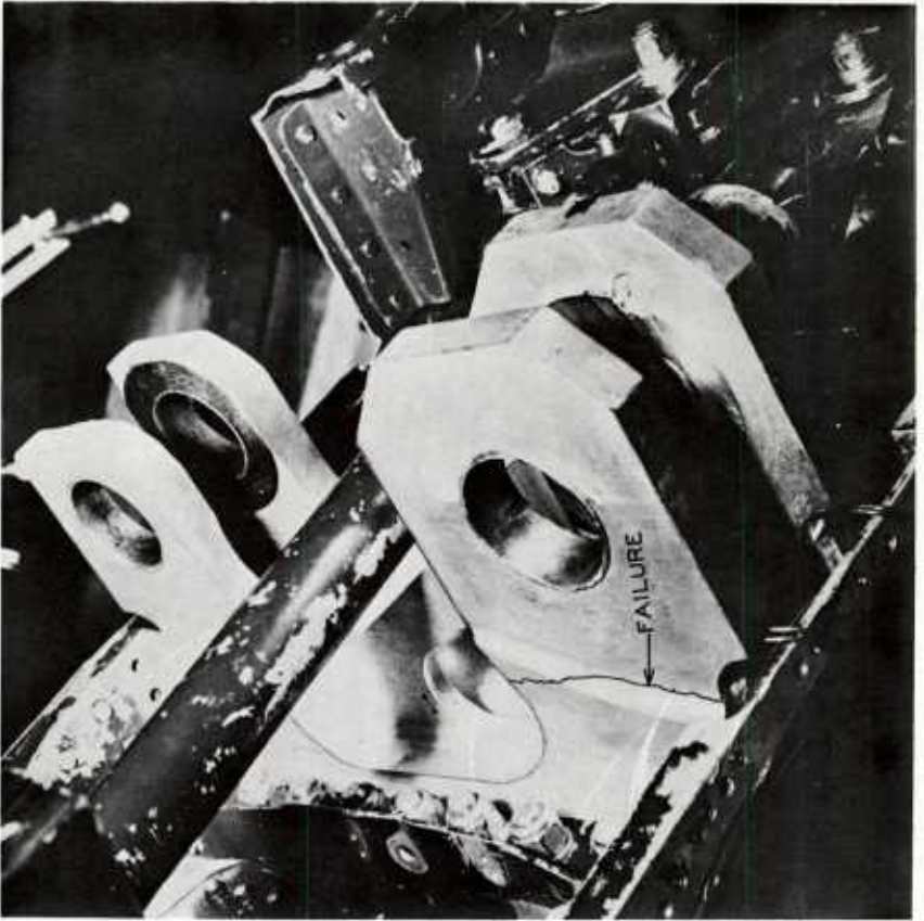
FIGURE 140.—Fatigue failure in wing-fold fitting—gouged fillet.
