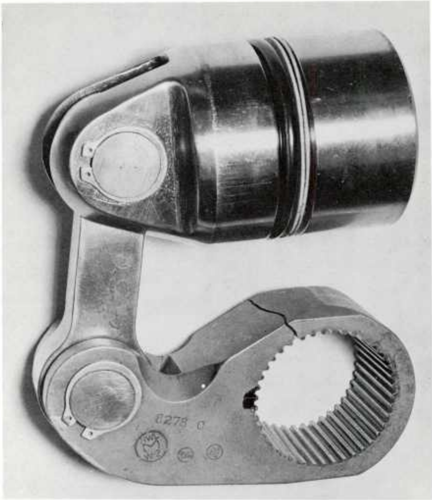
FIGURE 14.—Fatigue crack originating at spline.
