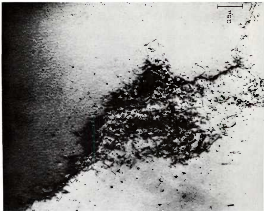
FIGURE 21.—Electron microscope transmission photos of fatigued pure aluminum—Continued.
