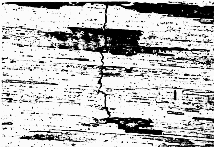
Figure A-3 - Intergranular R-direction stress-corrosion cracks originating from tip of transgranular W-direction crack; 7075- T6 exposed to methanol for 19,906 minutes at K_{Ii} = 30.7 \text{ ksi } \sqrt{\text{in.}} 50X magnification.
