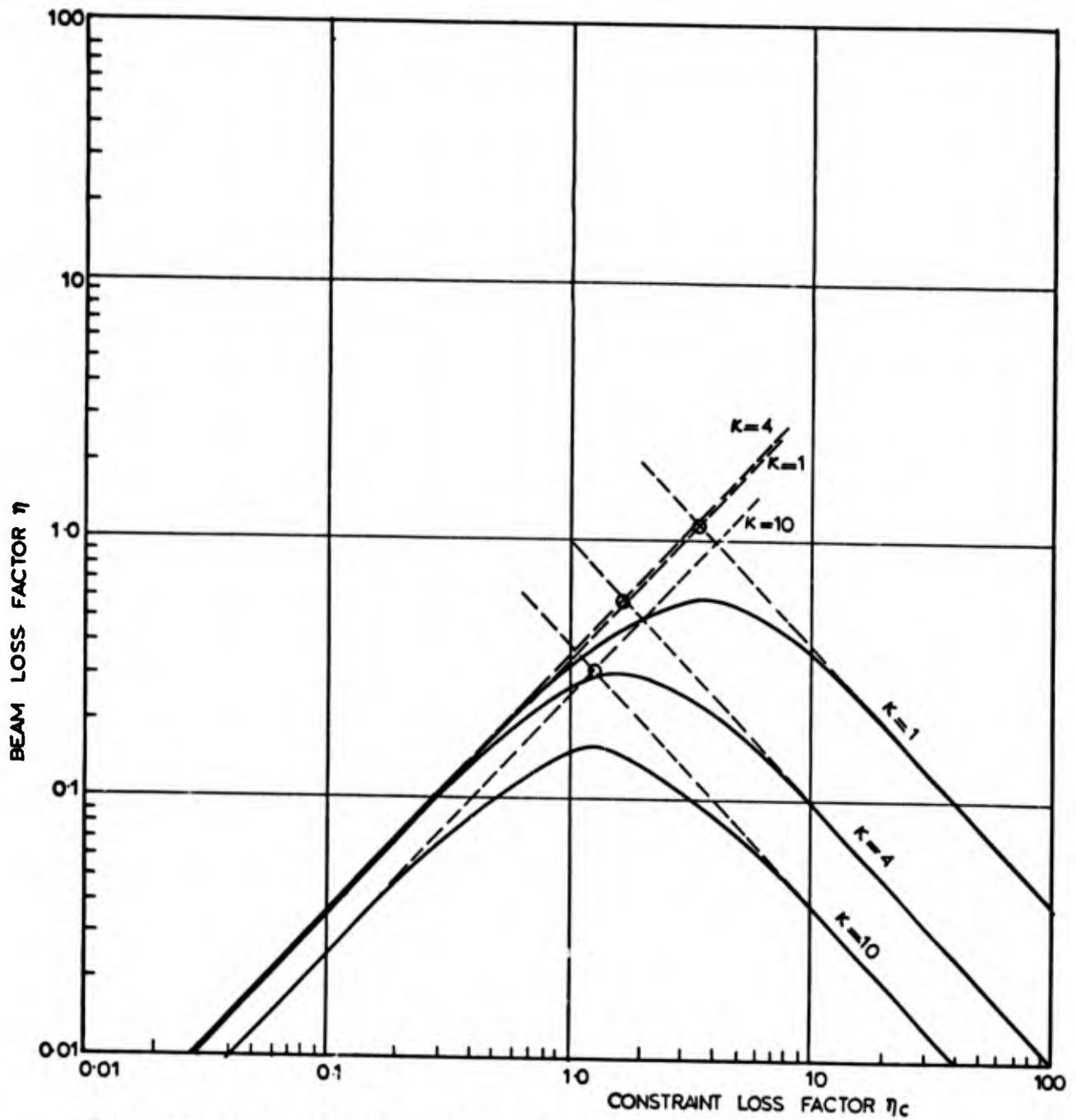
Figure 7. Beam loss factors for given constraint stiffnesses  $\kappa$
