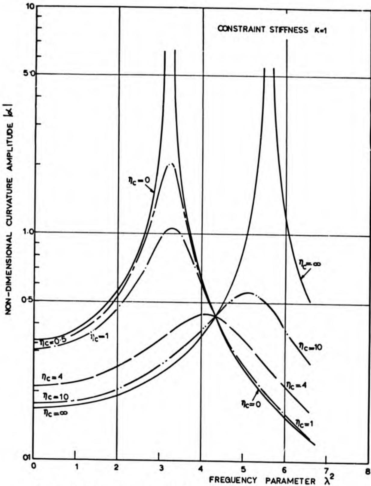
Figure 2. Curvature amplitude at beam centre  $|\kappa|$  plotted against frequency parameter  $\lambda^2$ . Constraint stiffness  $\kappa=1$
