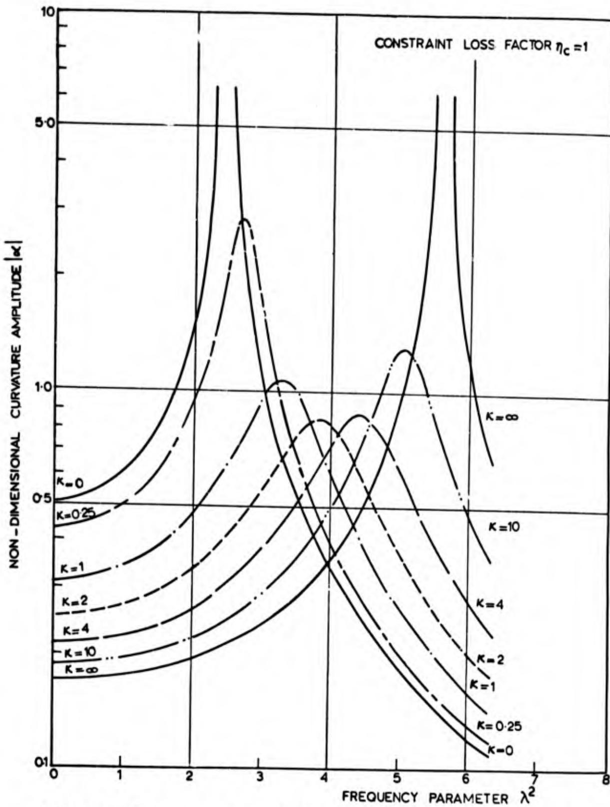
Figure 3. Curvature amplitude at beam centre  $|\alpha|$  plotted against frequency parameter  $\lambda^2$ . Constraint loss factor  $\eta_c = 1$
