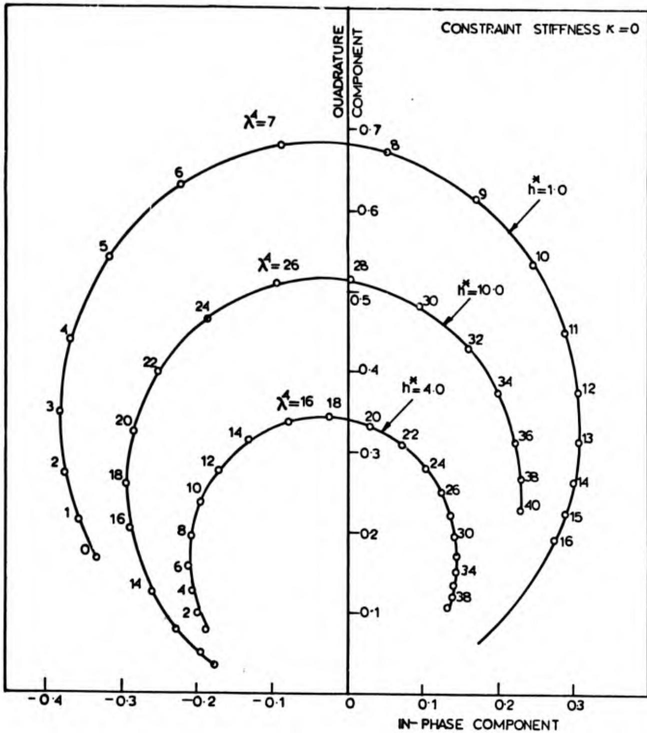
Figure 5. Vector response diagram. Variation with  $(\text{frequency})^2$
