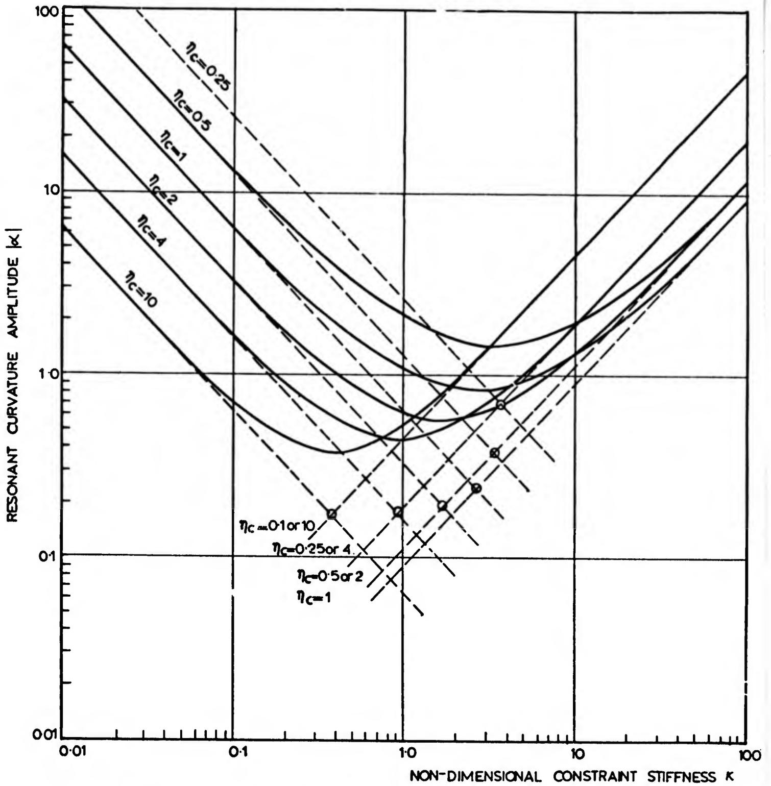
Figure 6. Resonant curvatures of beam for given constraint loss factors  $\eta_c$
