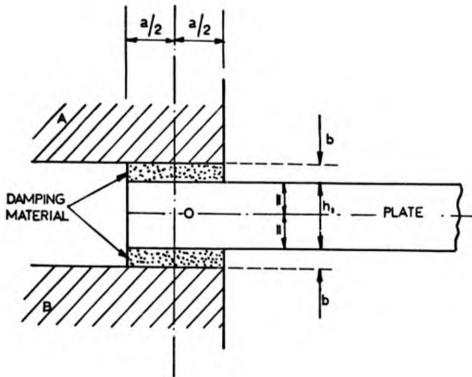
Figure 9. Diagram showing dimensions of root constraining layers
