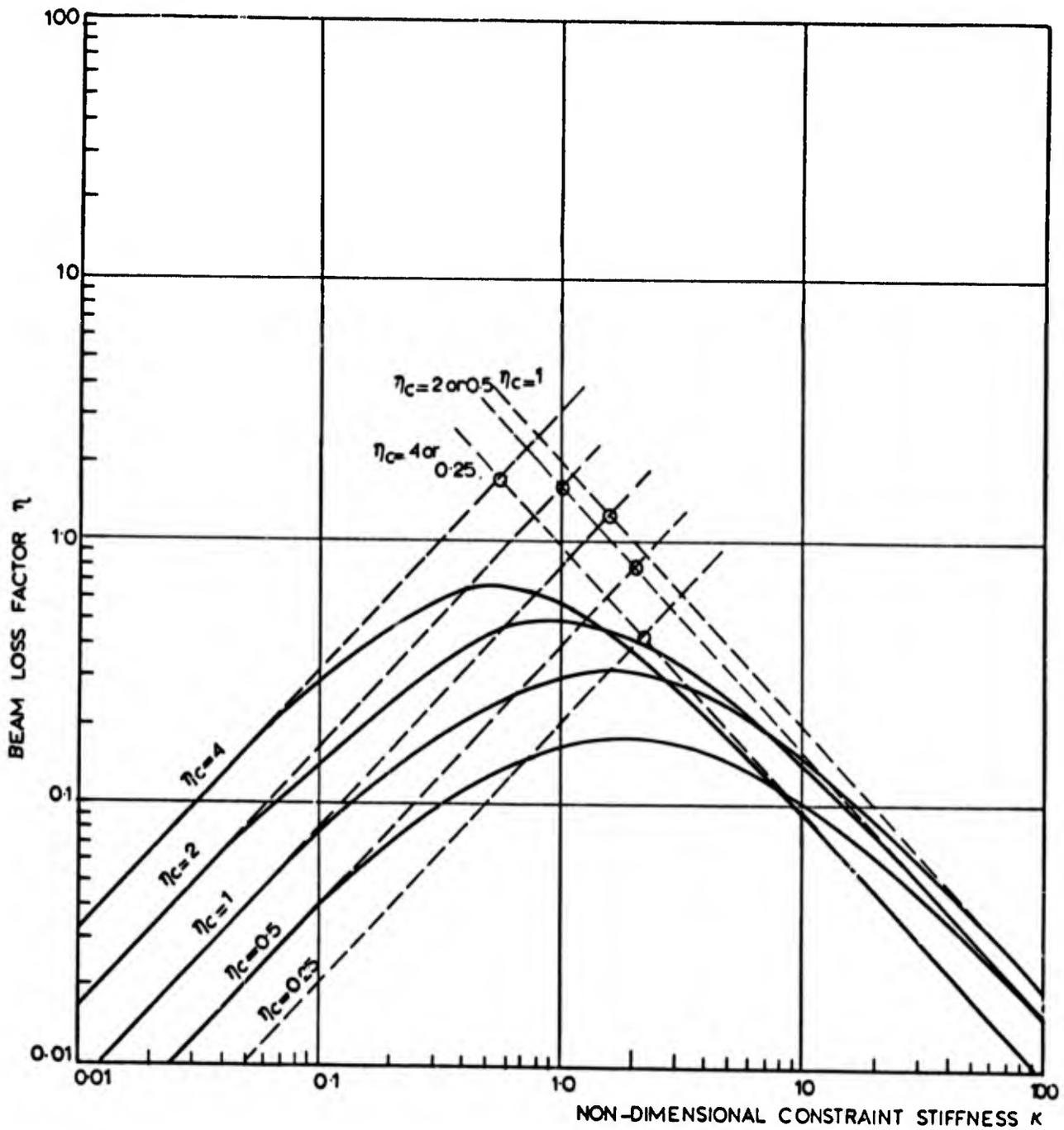
Figure 8. Beam loss factors for given constraint loss factors
