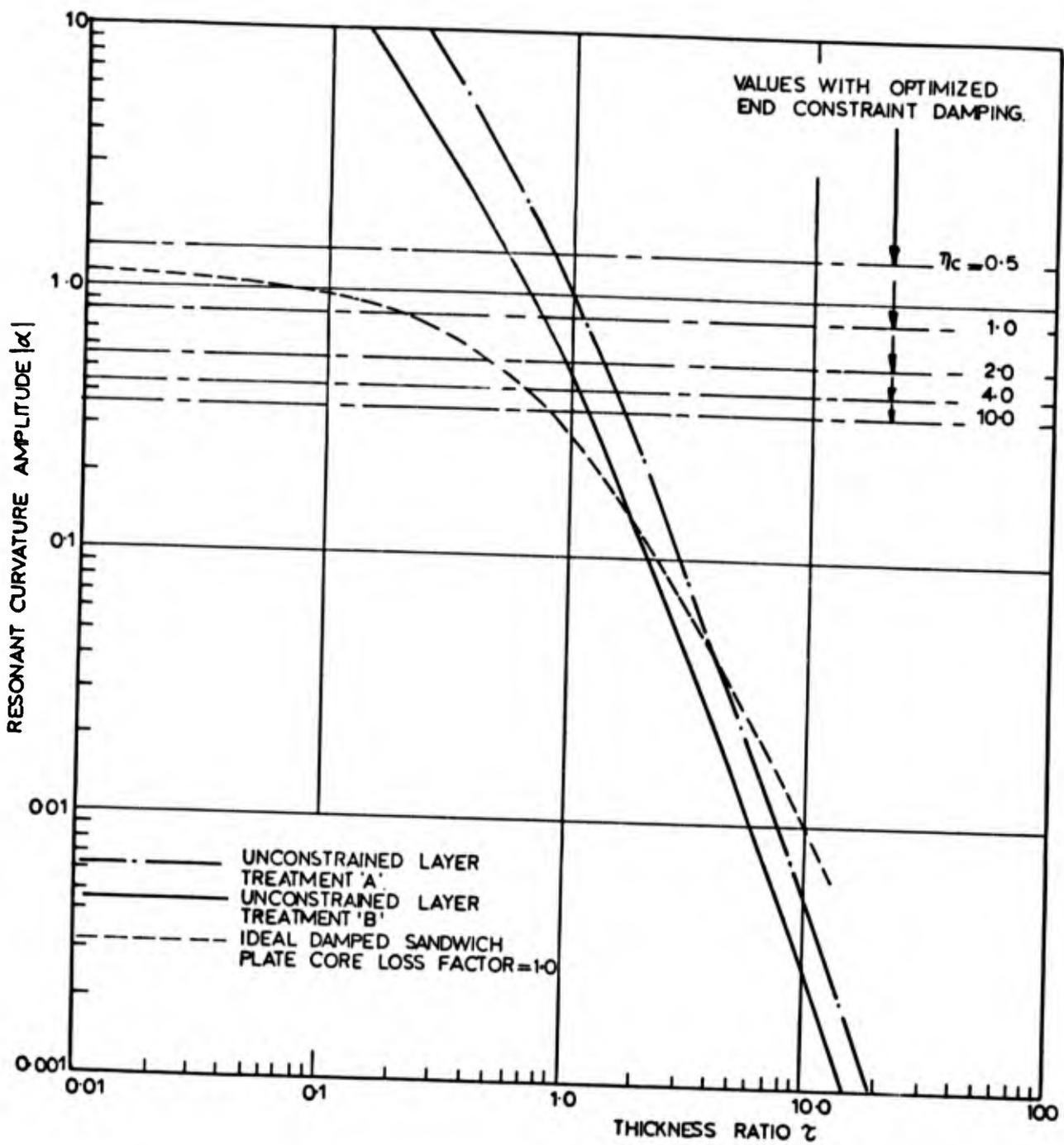
Figure 10. Resonant curvatures of beam with different damping mechanisms
