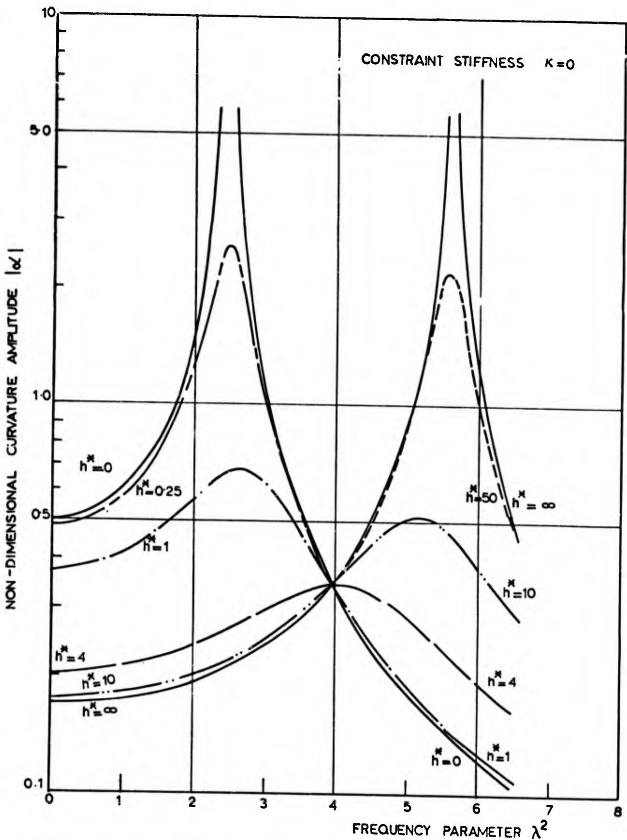
Figure 1. Curvature amplitude at beam centre  $|\alpha|$  plotted against frequency parameter  $\lambda^2$ . Constraint stiffness  $k = 0$
