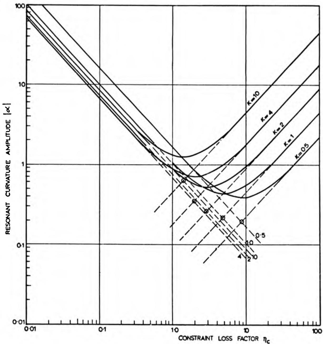
Figure 4. Resonant curvatures of beam for given constraint stiffnesses  $\kappa$
