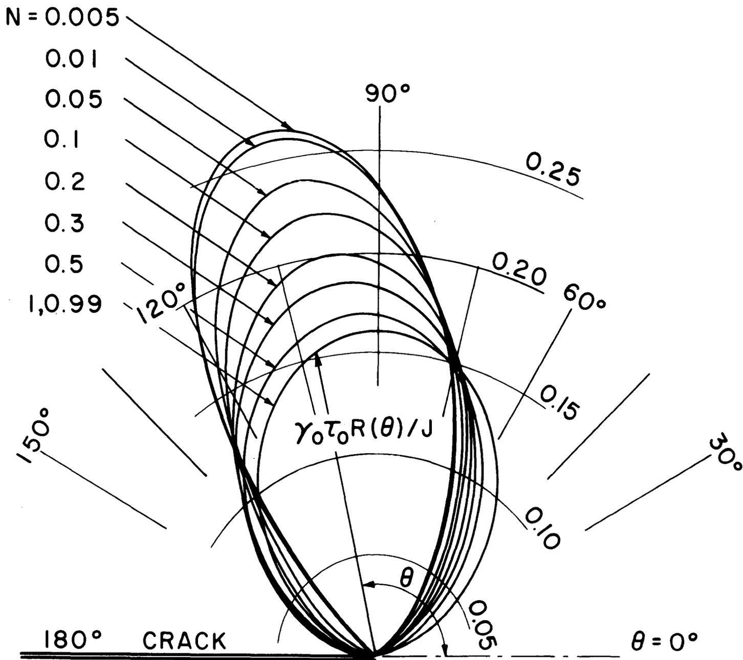
FIG. 3. APPROXIMATE LOCATION OF ELASTIC-PLASTIC BOUNDARY AND GEOMETRICAL SHAPE OF CONSTANT EQUIVALENT SHEAR LINES VERY NEAR THE CRACK TIP.
