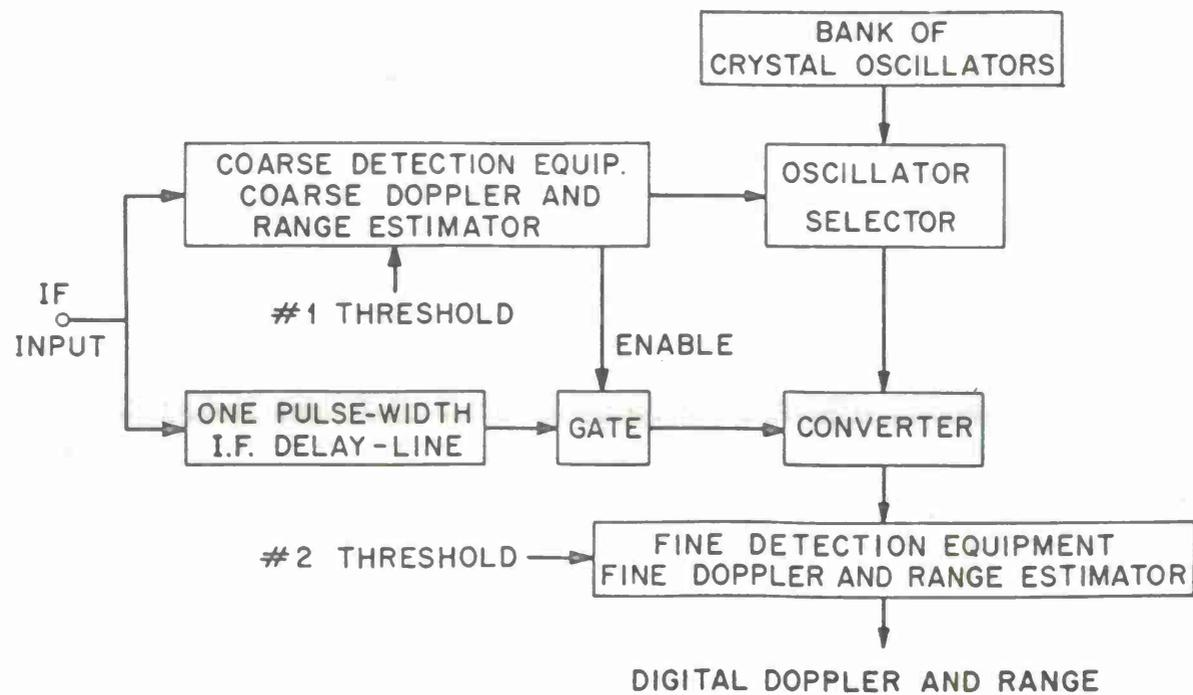
SEQUENTIAL DETECTION AND PROCESSING SYSTEM
