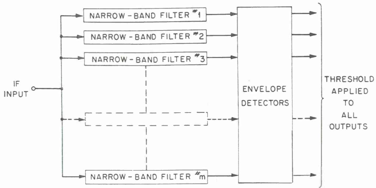
METHOD FOR DETECTION GOOD AT LOW, MEDIUM AND HIGH S/N
