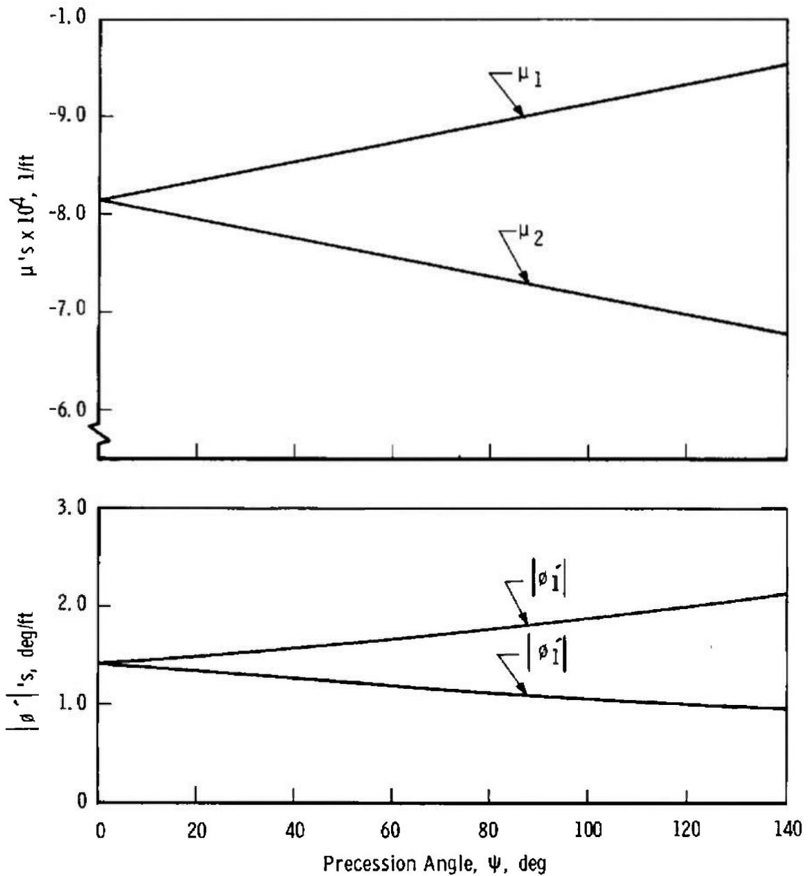
Fig. 5 Variation of  $\mu'$ 's and  $\phi'$ 's as Functions of Precessional Angle for a Simulated 5-deg, Semiangle Cone Model
