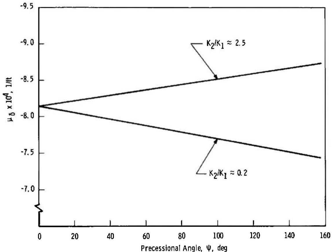
Fig. 6 Damping Evolved from the Amplitude Variation of the Computed Motion for a Simulated 5-deg, Semiangle Cone Model,  $|\mu_2| > |\mu_1|$
