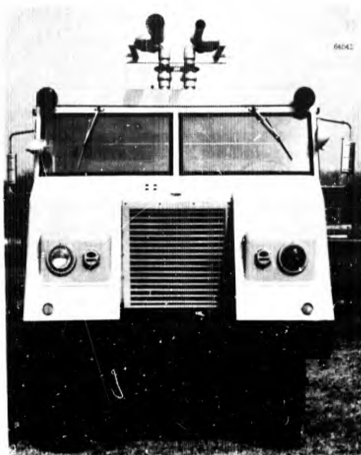
Fig. 10 - Front view of O6X experimental vehicle, showing mounting of the twinned-agent turret
