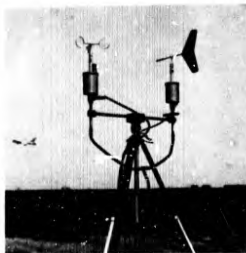
Fig. 16 - Overall view of portable wind-speed and direction instrumentation which fed into master recorder
