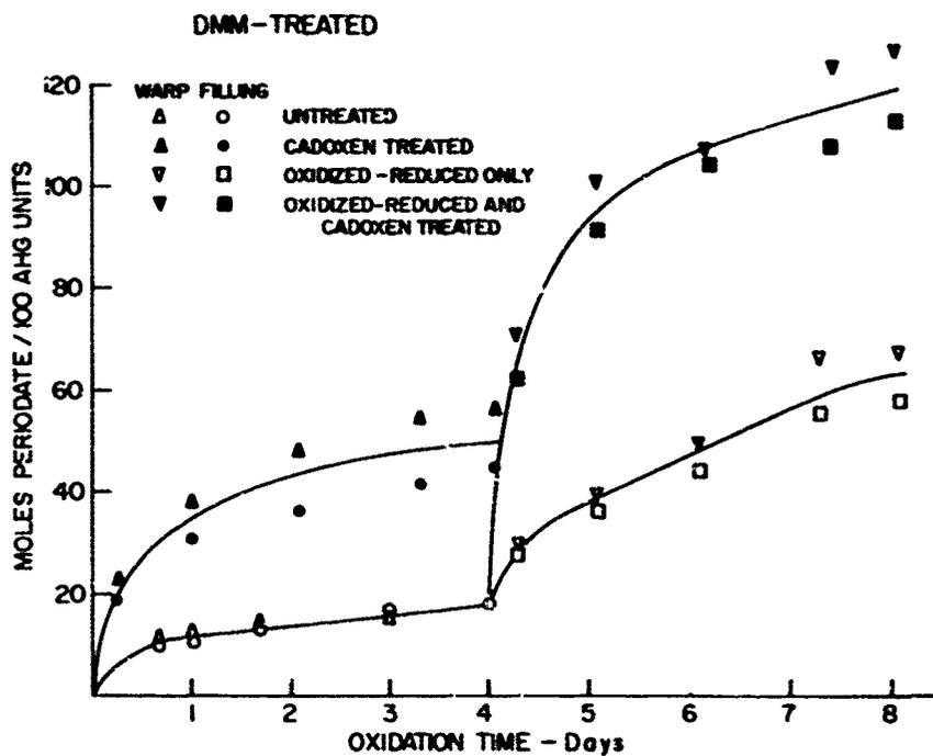
Fig. 21. Effect of cadoxen treatment on periodate oxidation.
