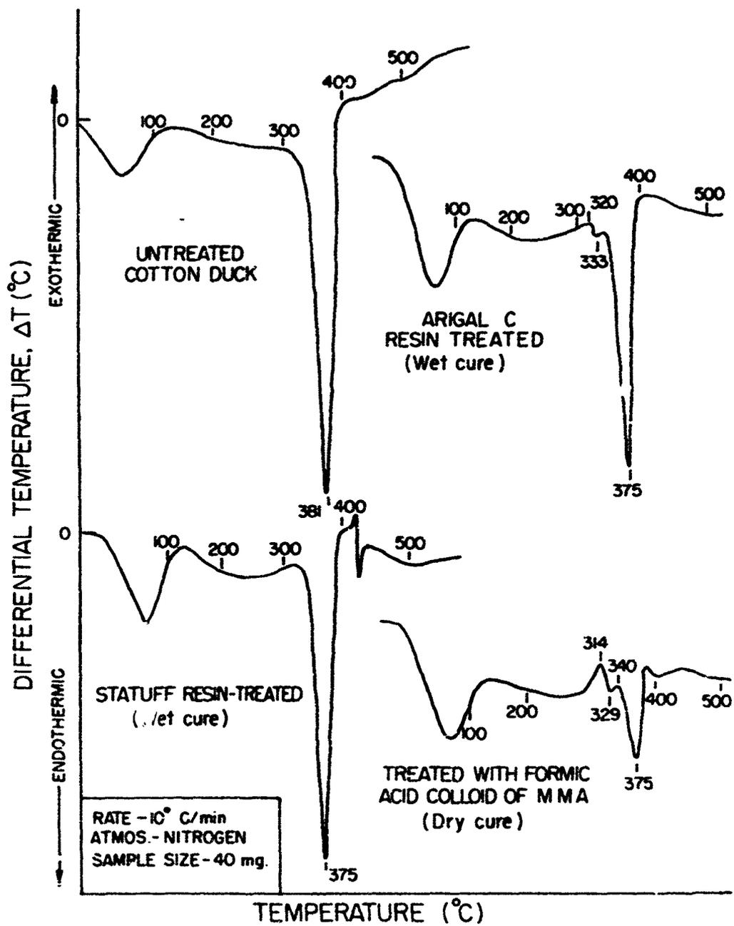
Fig. 1. DTA Curves of Untreated and Resin-Treated Cotton Duck.
