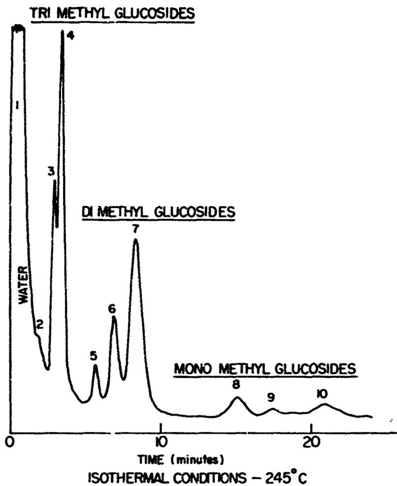
Fig. 7. Gas Chromatogram Showing Separation of Methyl Glucosides.
