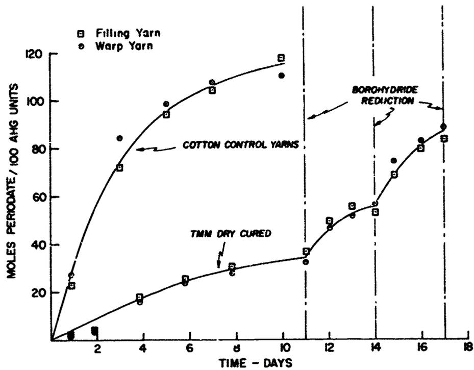
Fig. 14. Peroxide Oxidation of TMM-treated Cotton Sheeting, Buffered at pH 5.2.
