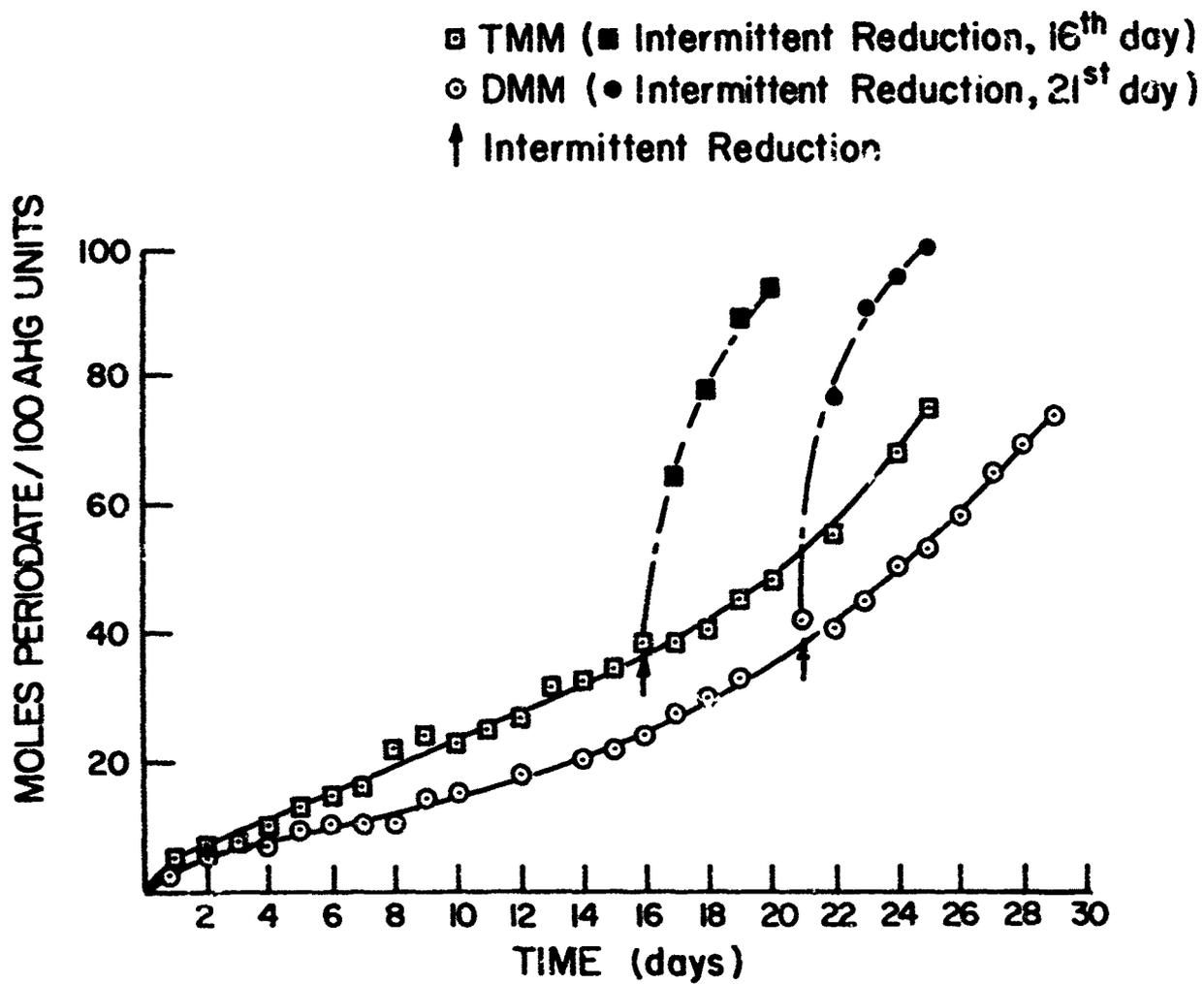
Fig. 12. Periodate Oxidation of TMM and DMM Dry-Cured Cotton Print Cloth with Intermittent Reduction.
