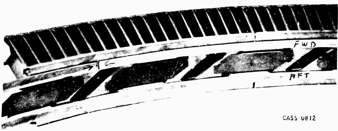
Figure I-77 Lift Fan Rotor Segmented Torque Band
