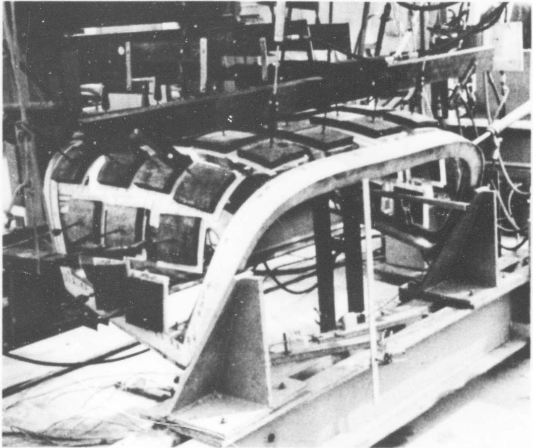
Figure 111 View of Canopy Test Whiffletree Setup and Supporting Structure
