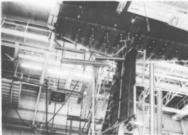
Figure 62 View Showing Aft Vertical and Side Whiffletree Loading Arrangement
