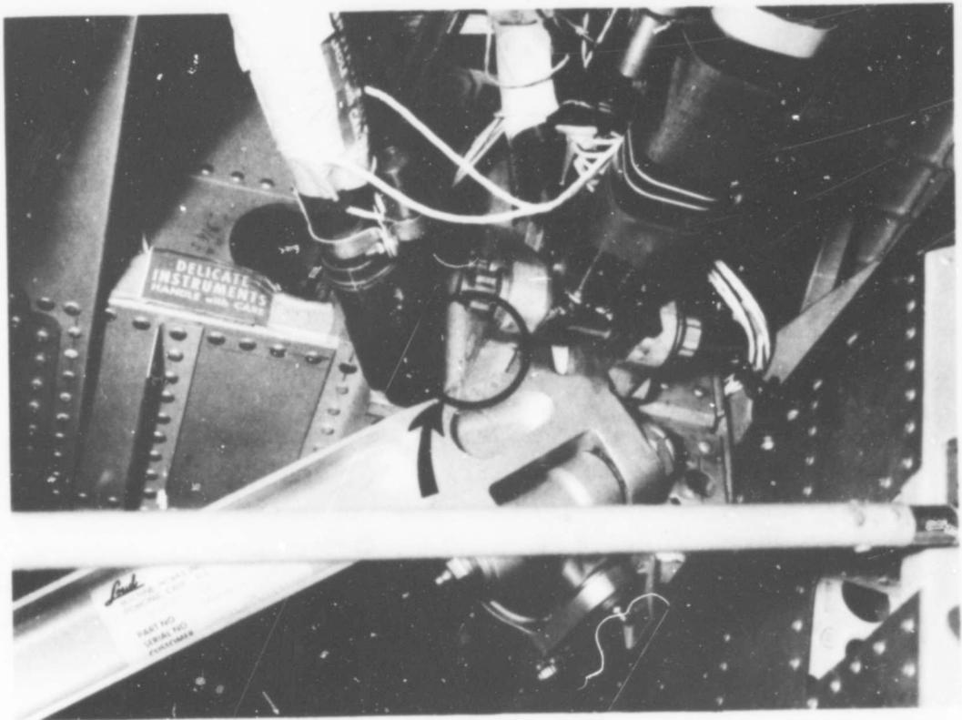
Figure 96 View Showing Failed Bolt on Landing Gear Brace Bracket
