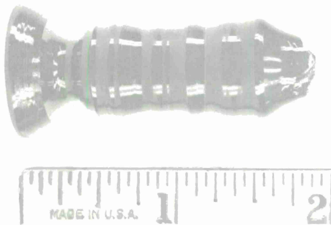
Fig. 1. Photograph of single crystal \text{Ti}_2\text{O}_3 boule 115 grown as described in the text.
