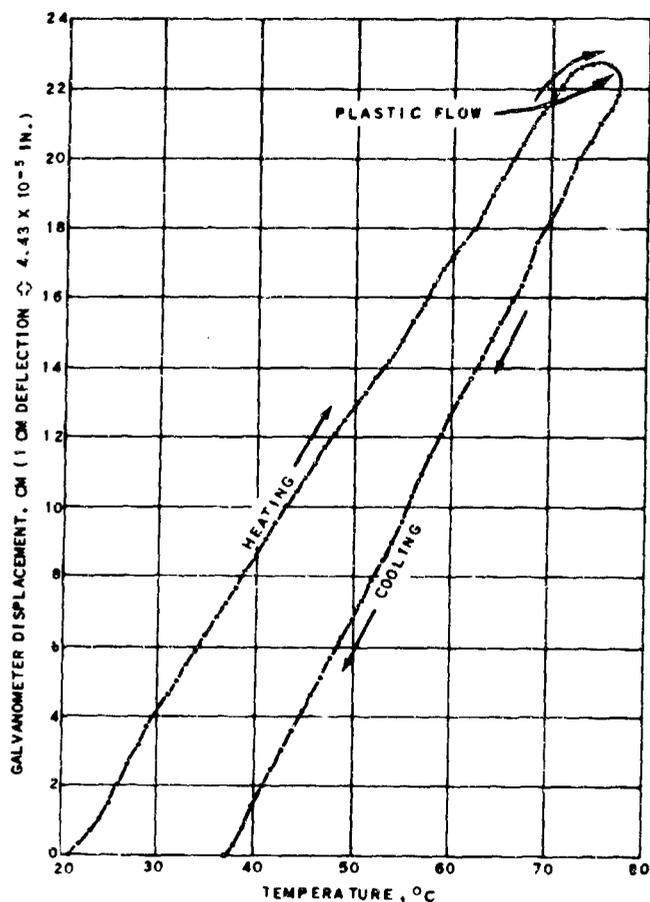
Fig. 5. Length Changes of Alpha-TNT Along the Intermediate Axis.
