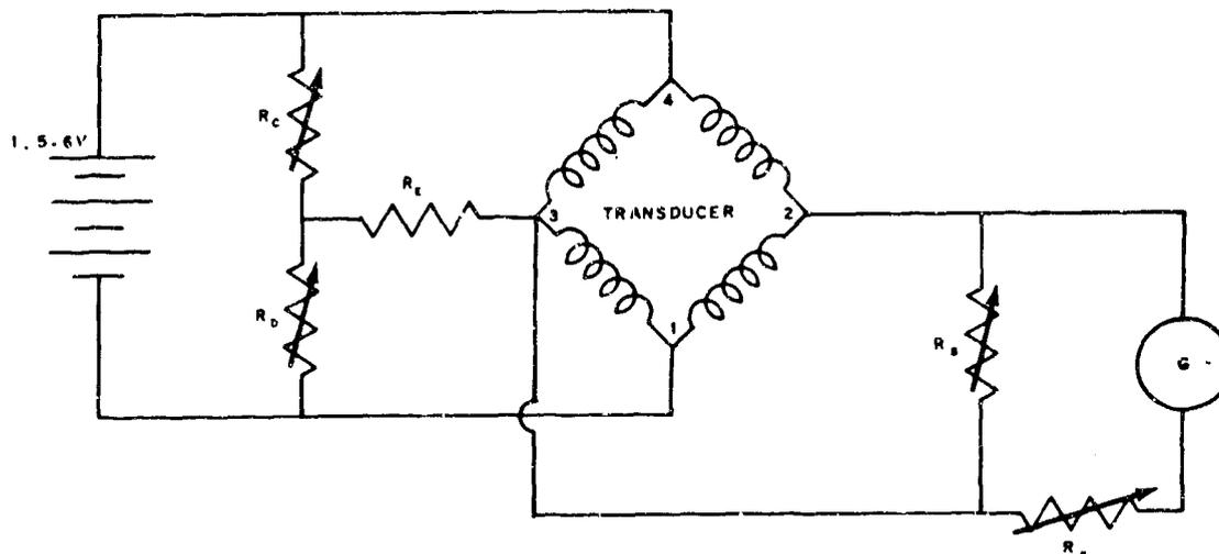
Fig. 2. Transducer Circuit for Measuring Displacement.  $R_C$ ,  $R_D$ ,  $R_S$ , and  $R_X$  are decade resistance boxes with a range of 0 to 100,000 ohms;  $R_E$  is a fixed wire-bound resistor with a resistance of 5,000 ohms; and  $G$  is a suspension galvanometer with a sensitivity of  $0.0013 \mu\text{amp/mm}$ .
