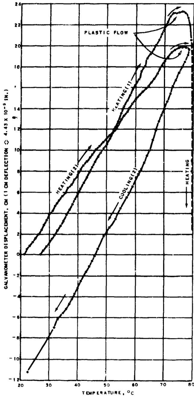
Fig. 6. Length Changes of Alpha-TNT Along the Long Axis.
