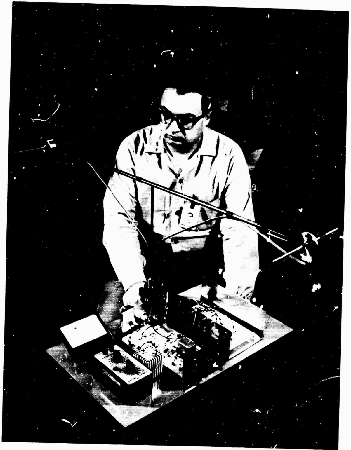
FIGURE 15. Differentially Connected Magnetometers and Associated Circuits
