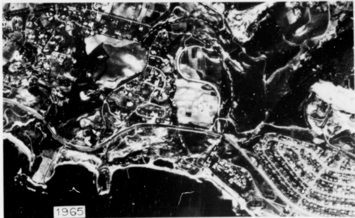
Aerial photographs of the same Portuguese Bend landslide area taken in 1956 and 1965. Note the absence of many houses between the highway and the shore in 1965. Dashed lines indicate approximate slide boundaries (1965).
