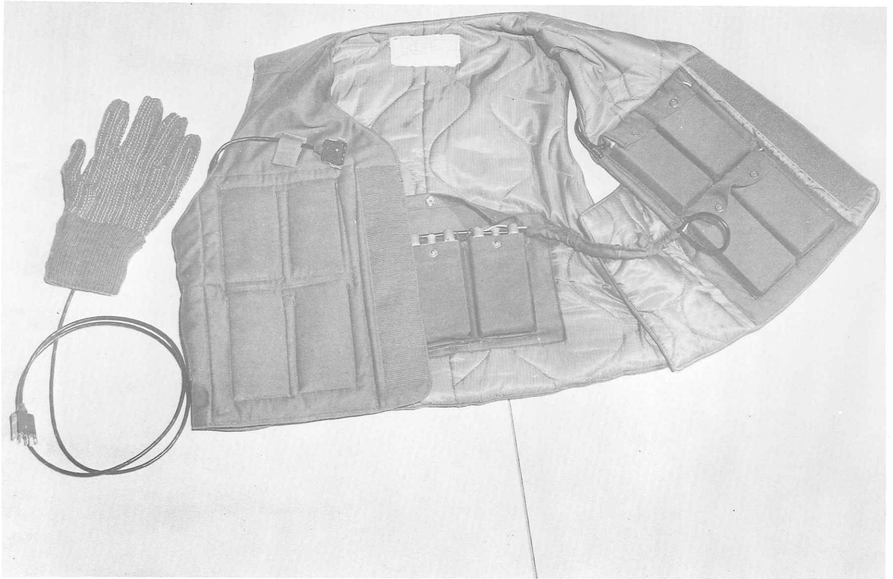
Figure 4. Type of Electrically Heated Handwear Unit Supplied to an Antarctic Plateau Expedition, Including a Battery Vest with 11 Silver Cadmium, 1.1 volt, 10 Ampere Rechargeable Cells and Wired Glove
