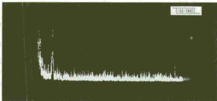
Fig. II-2. Return signal from moving automobile displayed on spectrum analyzer. Entire trace corresponds to frequency shifts of 1 MHz. Signal is seen near 100 kHz. At left is zero frequency response of analyzer.
