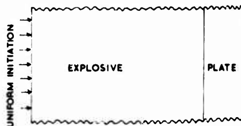
Fig. 1 - The 1D geometry calculated by NIP
