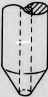
D. SHARP-EDGE TIP (WITH VACUUM PICKUP)
