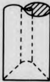
G. TRUNCATED-PYRAMID TIP (WITH VACUUM PICKUP)
