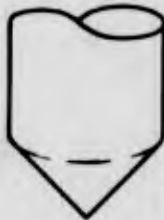
d. BLUNT NEEDLE-POINT TIP (45°-60° SLOPE)
