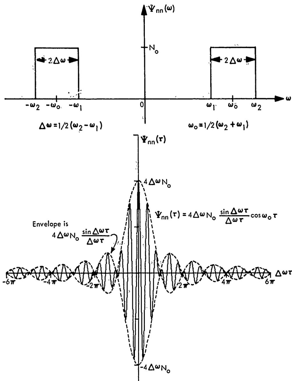
FIGURE 3. RECTANGULAR NARROW BAND SPECTRUM AND ASSOCIATED AUTOCORRELATION.
