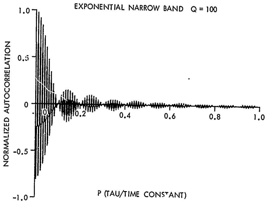
FIGURE 17 . EXPONENTIAL PULSE OF NARROW BAND NOISE
