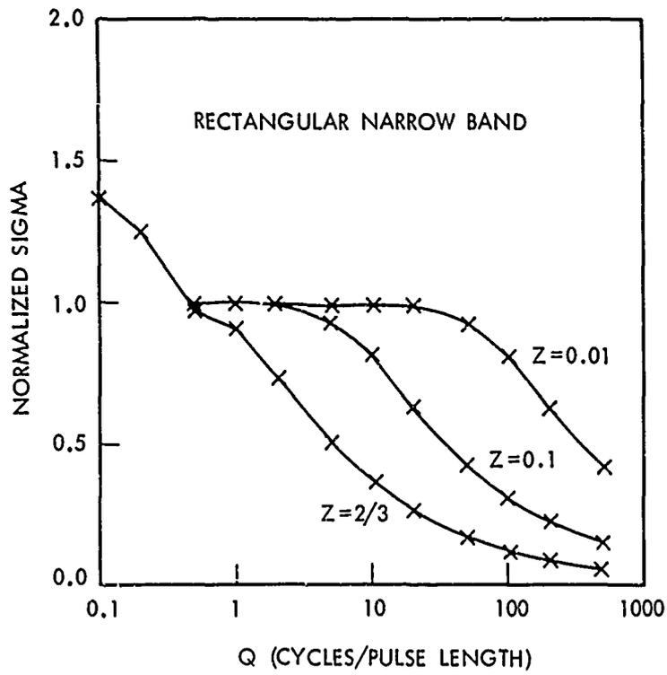
FIGURE 15. RECTANGULAR PULSE OF NARROW BAND NOISE
