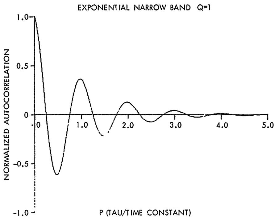
FIGURE 16. EXPONENTIAL PULSE OF NARROW BAND NOISE
