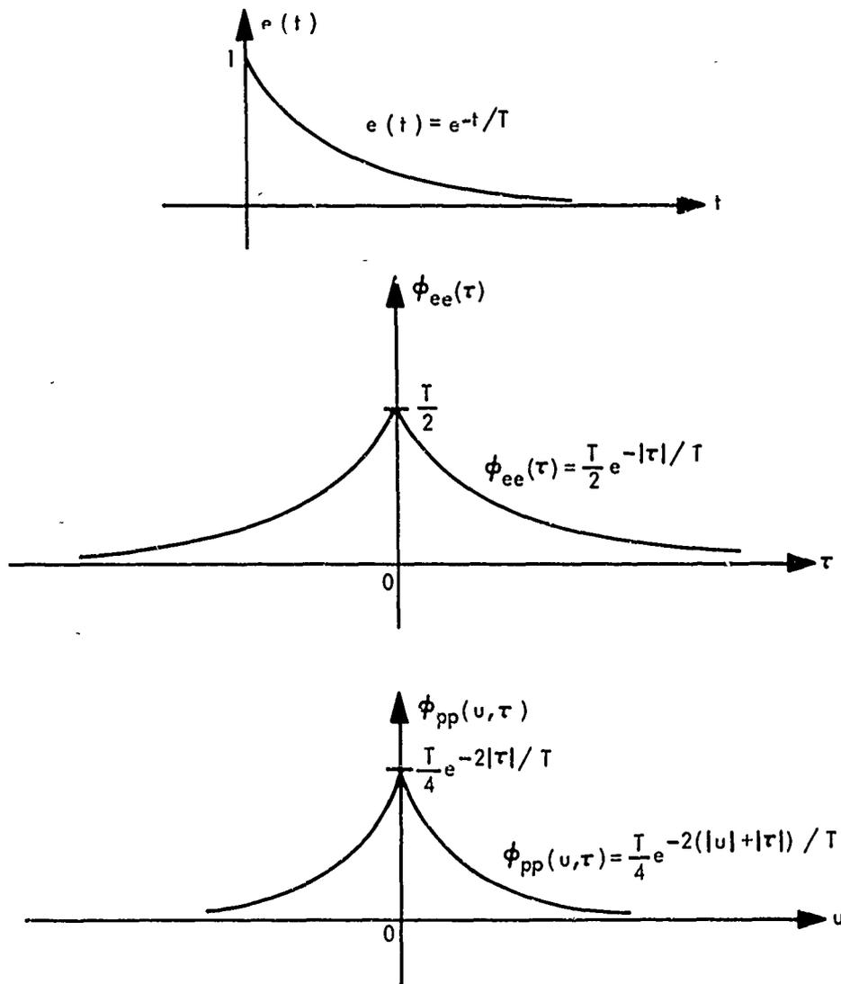
FIGURE 5. EXPONENTIAL ENVELOPE AND ASSOCIATED AUTOCORRELATION FUNCTIONS.
