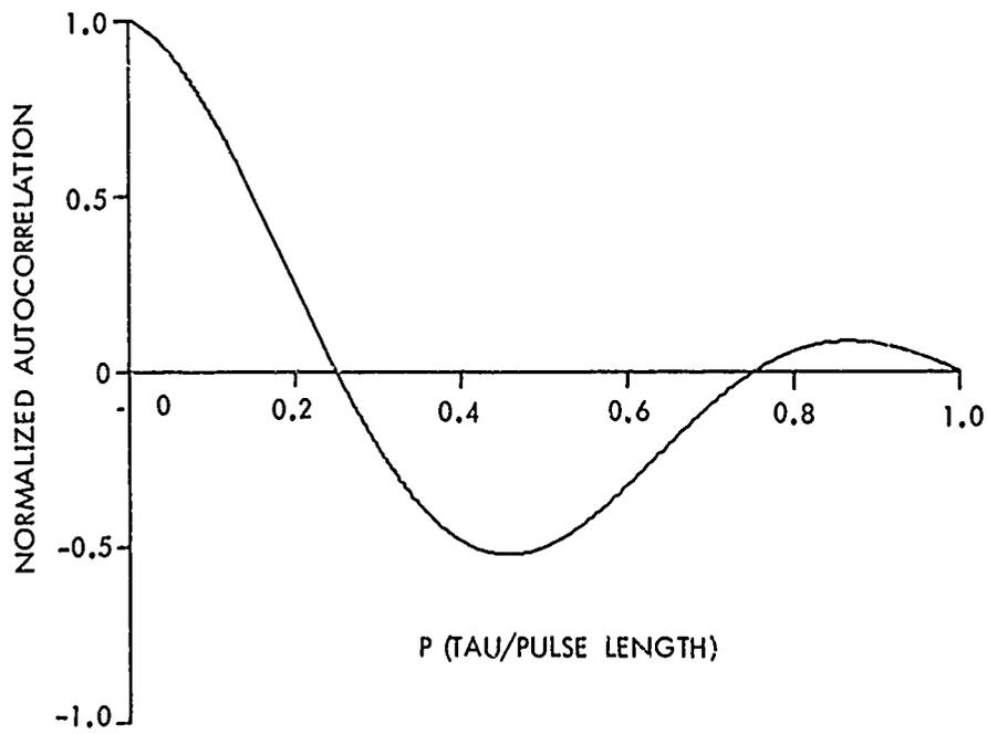
FIGURE 13. RECTANGULAR PULSE OF NARROW BAND NOISE AVERAGE AUTOCORRELATION FOR  $Z=0.1$
