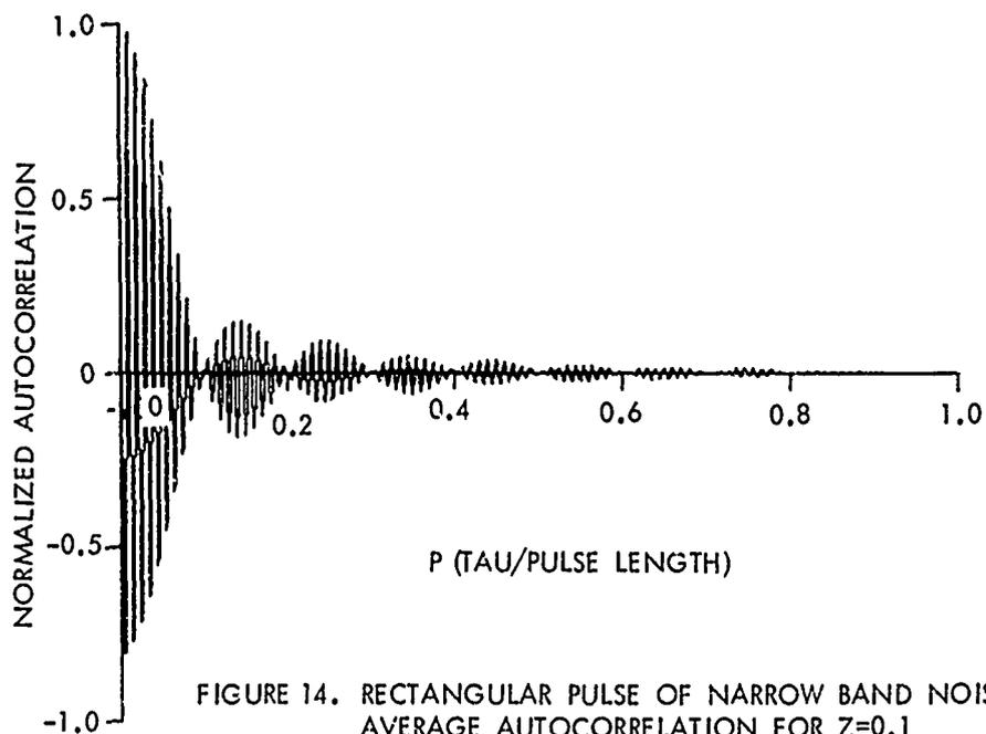
FIGURE 14. RECTANGULAR PULSE OF NARROW BAND NOISE AVERAGE AUTOCORRELATION FOR  $Z=0.1$
