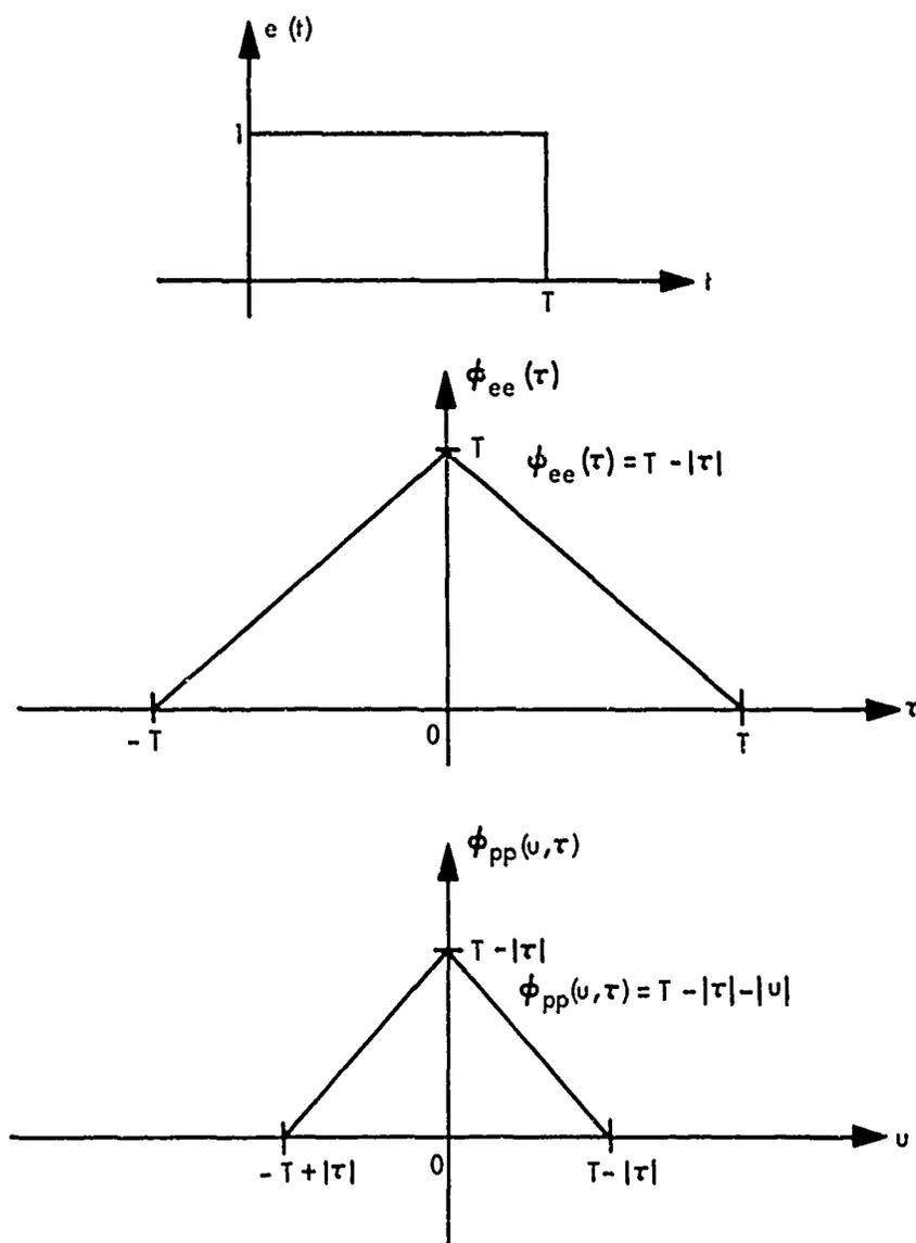
FIGURE 4. RECTANGULAR ENVELOPE AND ASSOCIATED AUTOCORRELATION FUNCTIONS
