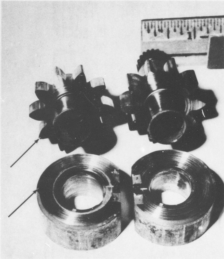
Figure 81. Fuel Pump Element Showing Worn Faces on Gears and Bearings (Arrows).
