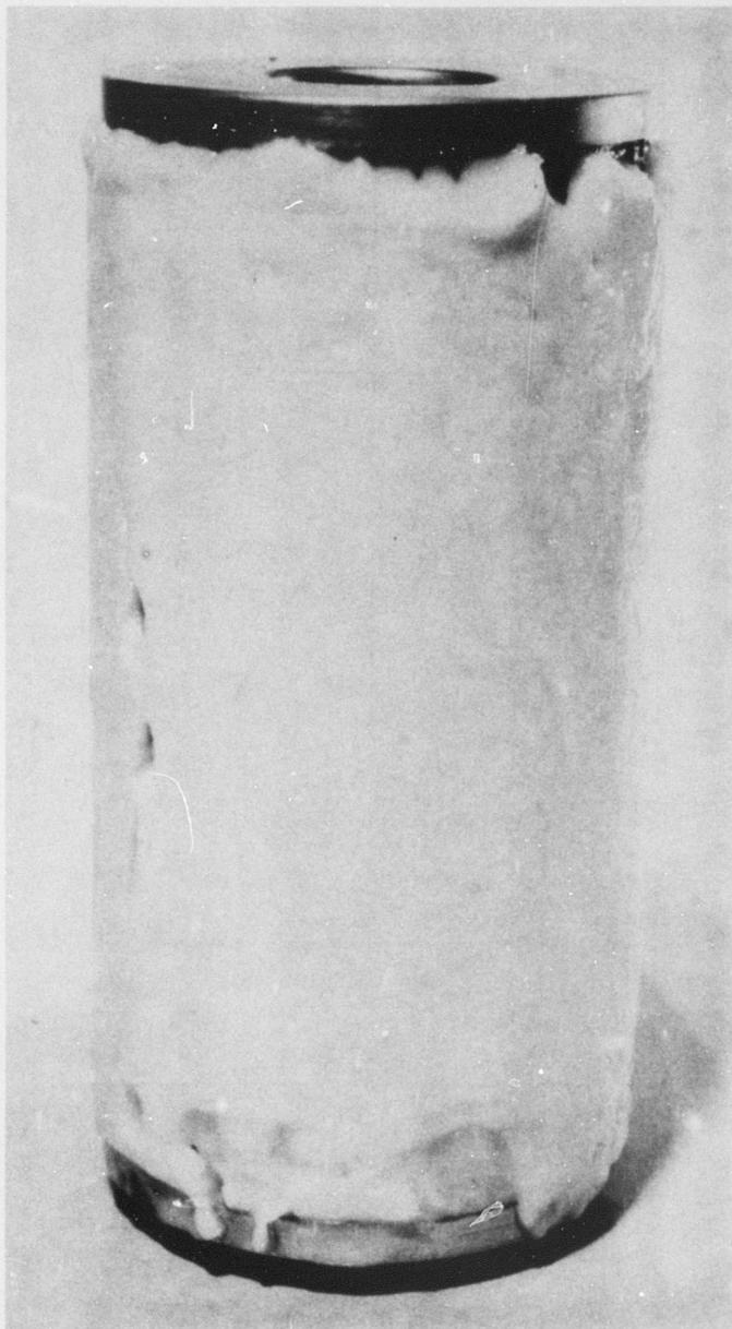
Figure 68. Fuel Filter Completely Clogged With Emulsified Fuel.
