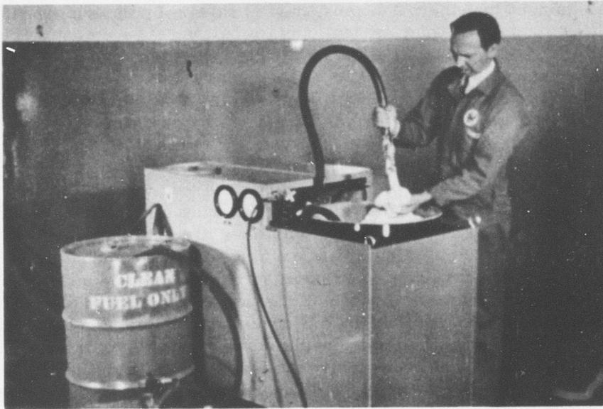
Figure 21. Westco emulsified fuel mixing and supply rig during fuel mixing.
