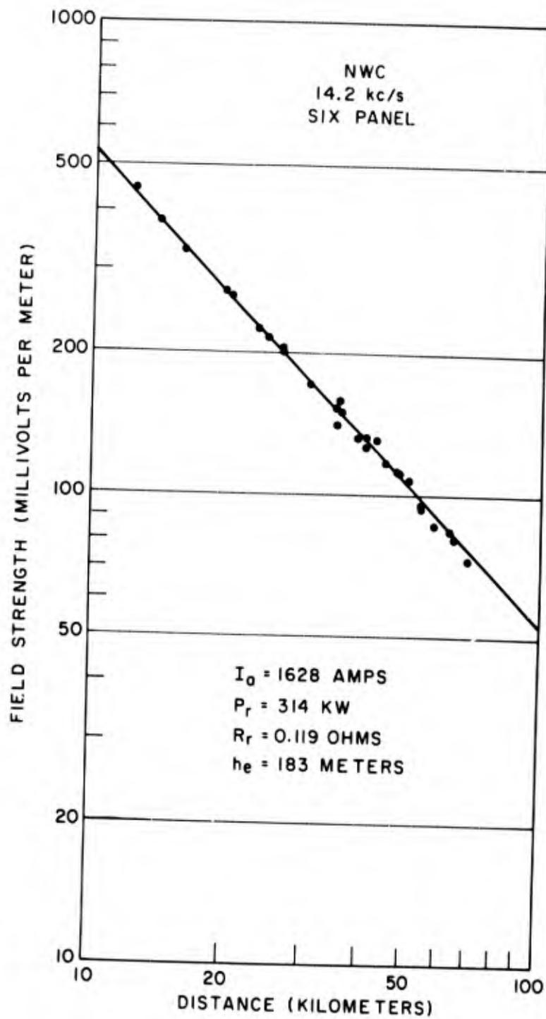
Figure 4 - Field strength normalized to a constant antenna current as a function of distance from the NWC antenna operating with six panels at 14.2 kc/s
