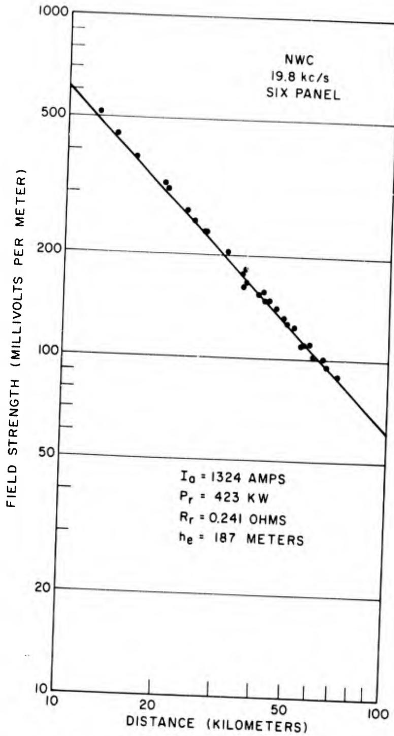
Figure 6 - Field strength normalized to a constant antenna current as a function of distance from the NWC antenna operating with six panels at 19.8 kc/s
