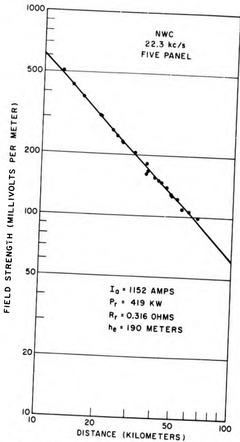
Figure 12 - Field strength normalized to a constant antenna current as a function of distance from the NWC antenna operating with five panels at 22.3 kc/s
