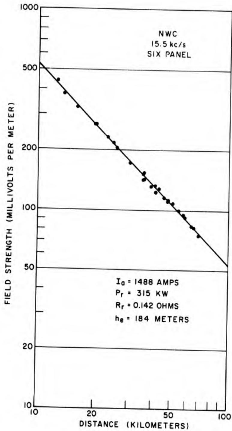
Figure 5 - Field strength normalized to a constant antenna current as a function of distance from the NWC antenna operating with six panels at 15.5 kc/s
