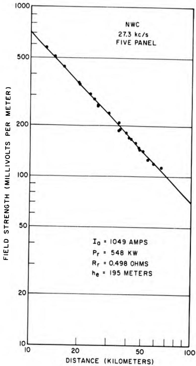
Figure 13 - Field strength normalized to a constant antenna current as a function of distance from the NWC antenna operating with five panels at 27.3 kc/s
