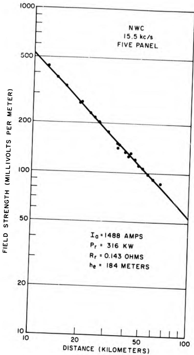
Figure 10 - Field strength normalized to a constant antenna current as a function of distance from the NWC antenna operating with five panels at 15.5 kc/s
