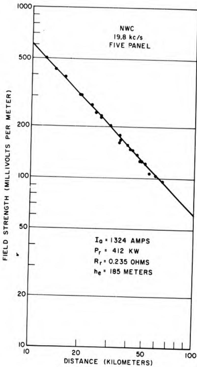
Figure 11 - Field strength normalized to a constant antenna current as a function of distance from the NWC antenna operating with five panels at 19.8 kc/s
