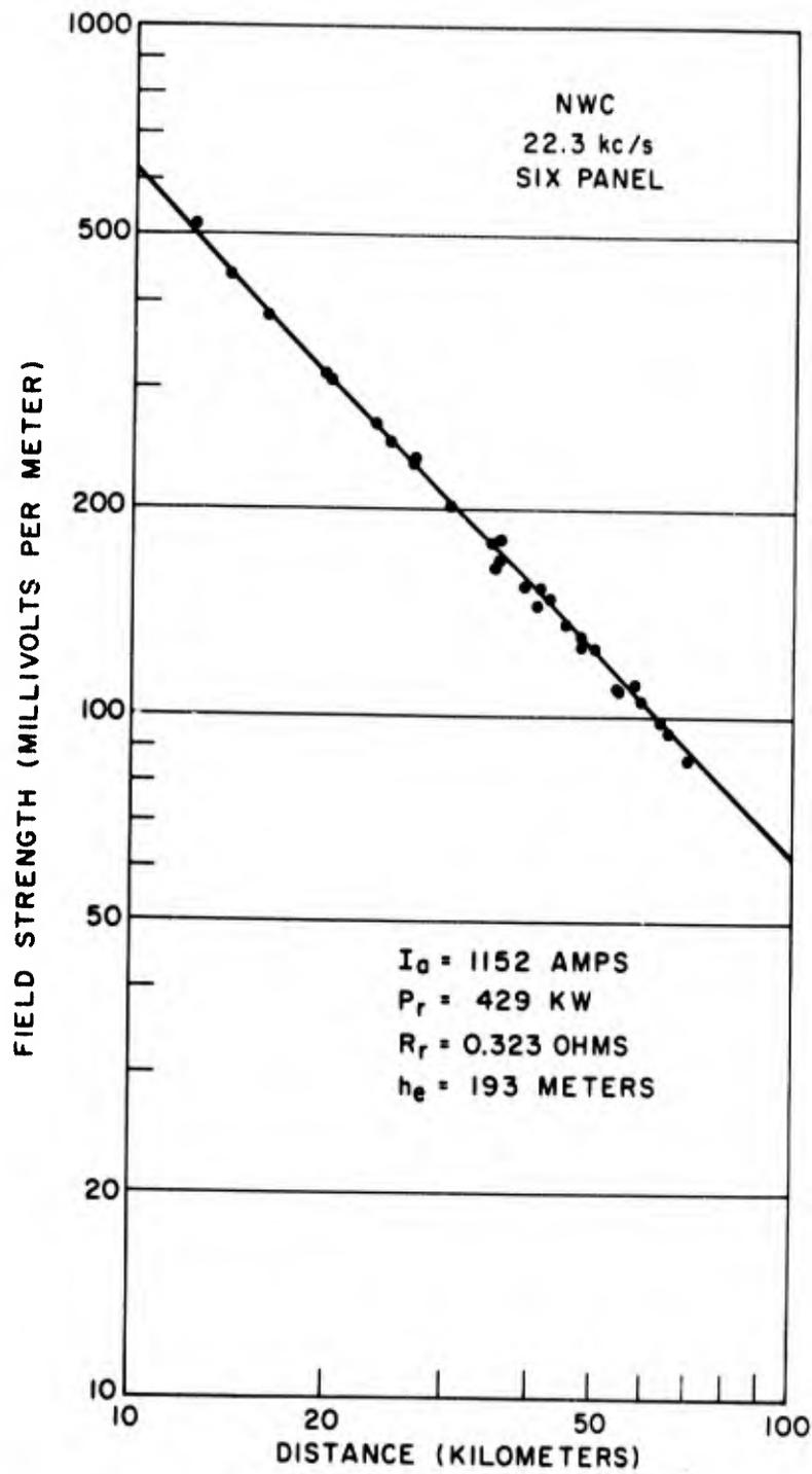
Figure 7 - Field strength normalized to a constant antenna current as a function of distance from the NWC antenna operating with six panels at 22.3 kc/s
