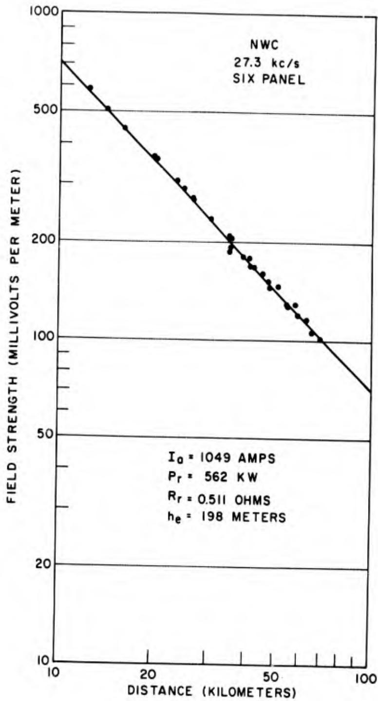
Figure 8 - Field strength normalized to a constant antenna current as a function of distance from the NWC antenna operating with six panels at 27.3 kc/s
